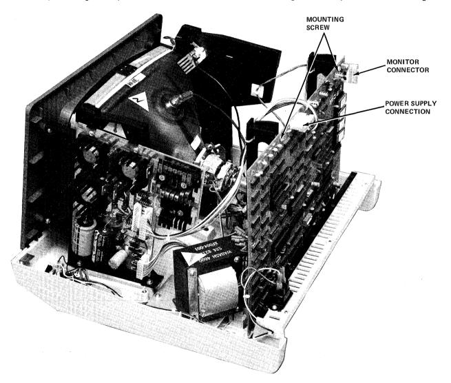
Figure 10-2. PCB Mounting
