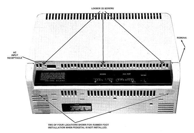
Figure 10-1. Top Cover Removal
