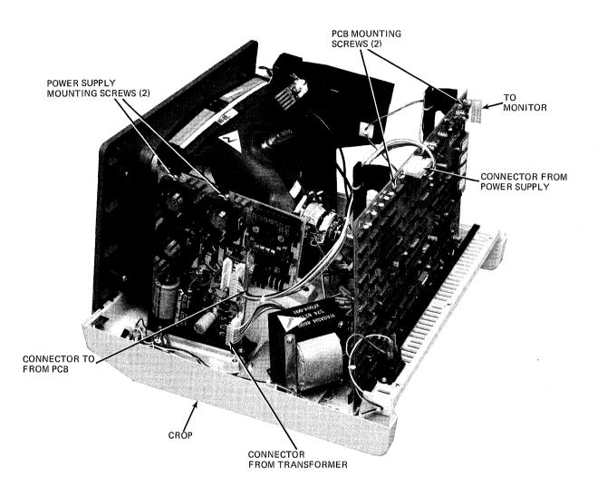
Figure 10-3. PCB Mounting
