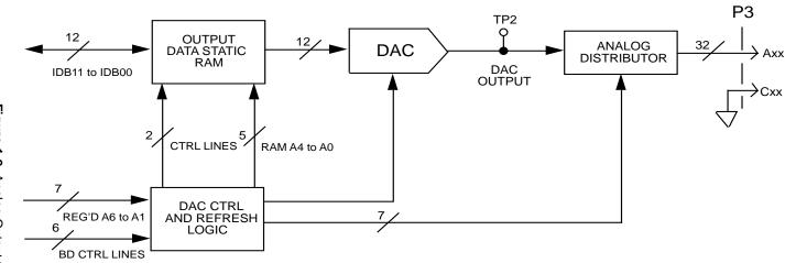
Figure 1-3 Analog Output Distribution
