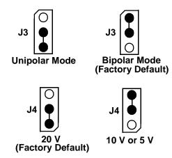
Figure 2-5 Loopback Input Voltage Range Selection
