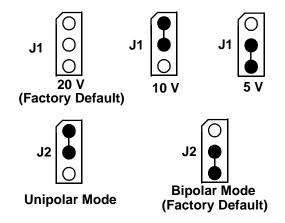
Figure 2-4 Analog Output Voltage Range Selection
