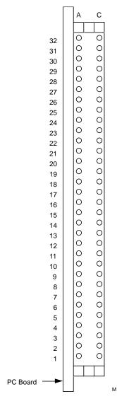
Figure 2-7 P3 Connector Pinout
