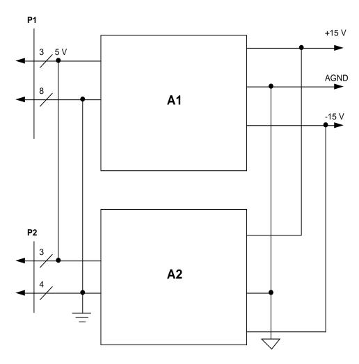
Figure 1-6 DC-to-DC Converter
