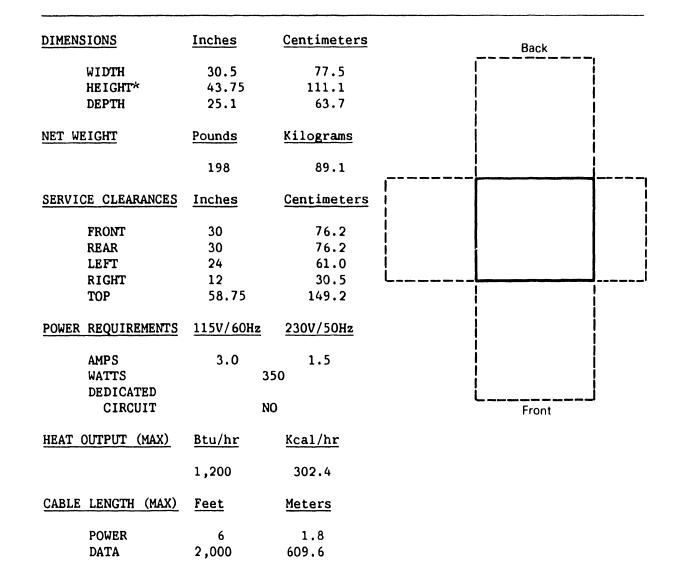
%Height with stand, cover closed. Height without stand: 14.5 in. (36.8 cm) cover closed 29.5 in. (74.9 cm) cover open
