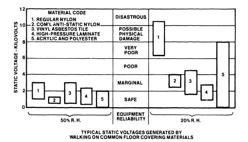
FIGURE 2-1 STATIC POTENTIAL OF COMMON FLOOR COVERINGS
