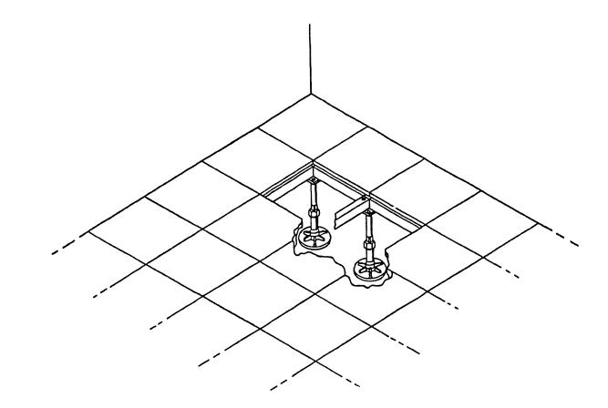
FIGURE 2-2 PEDESTAL-TYPE RAISED FLOORING
