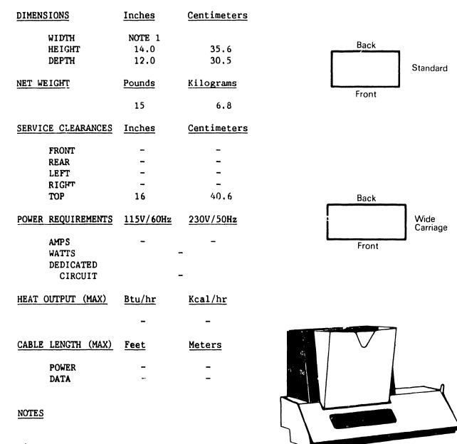
Width: Standard Printer - 23.5 in. (59.7 cm) Wide Carriage - 28.5 in. (72.4 cm)
