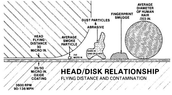
FIGURE 3-1 HEAD/DISK GAP IN RELATION TO POSSIBLE CONTAMINANTS
