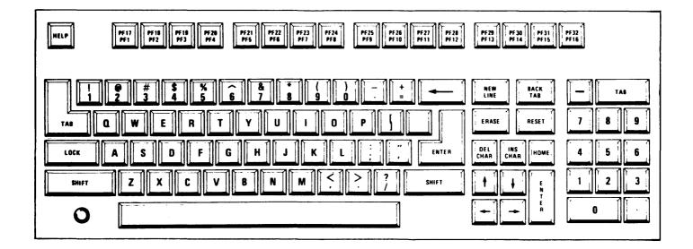
Figure 2-1. The VS Data Processing Workstation Keyboard
