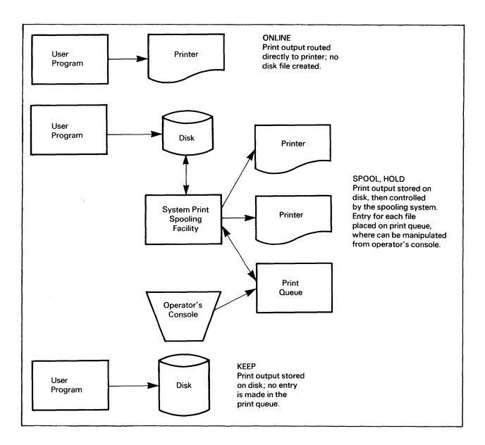
Figure 1-4. Schematic Representation of Print Modes
