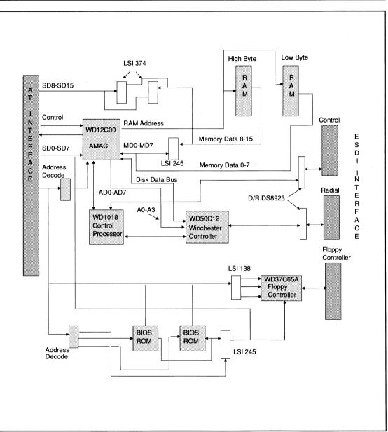
FIGURE 1. WD1007A-WA2 BLOCK DIAGRAM
