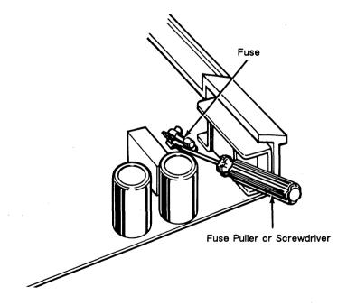
3. Check the fuse. If the fuse is broken or blackened, push a new fuse into the fuse socket.
