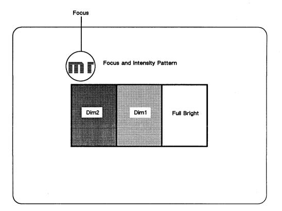
This pattern is an 80 or 132-column display of characters. (Hold the CTRL key and press the S key to toggle between 80 and 132 columns.) Three blocks in the center of the pattern indicate brightness: bright, normal, and dim.
