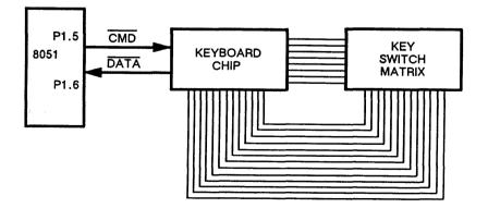
The keyboard PCB is arranged as a matrix of up to 13 rows of eight columns each. Each key switch connects one row to one column when that key is pressed. The keyscanner interface chip has 13 opendrain row outputs and eight column inputs with active pullups. The integrated circuit communicates with the external processor on two lines: the command line (CMD) and the data line (DATA).
