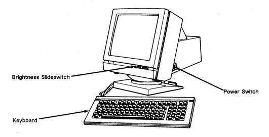
The power switch is on the right side of the terminal. Pressing the back of the switch turns AC power on.
