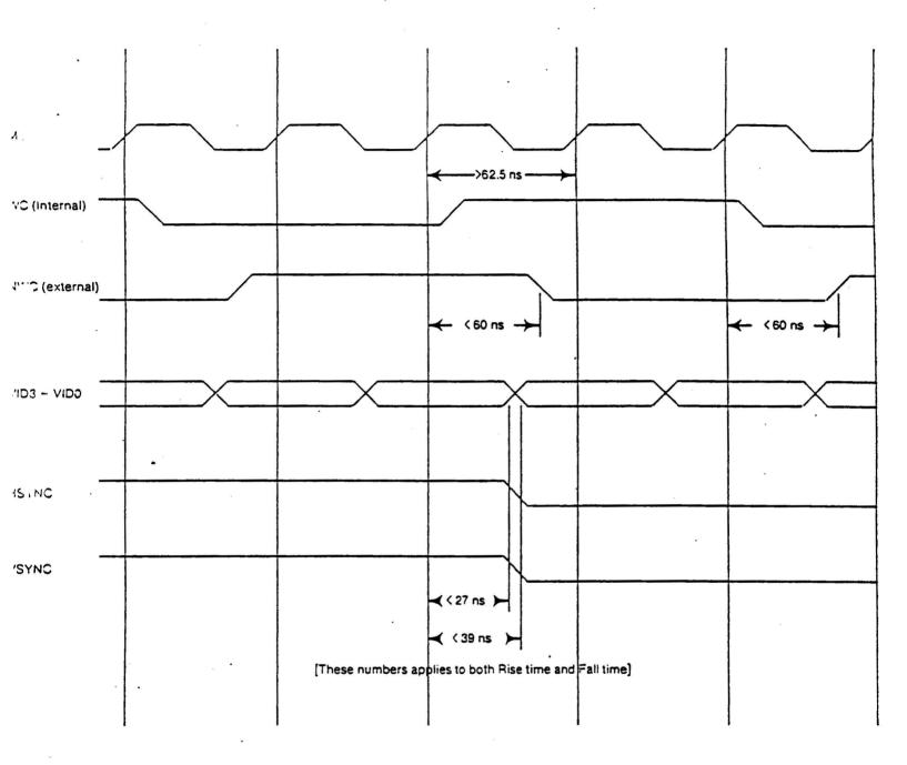
Aaximum rise time or Fall time is 12 ns Rise time is mesured from 0.8V to 2.0V fall time is mesured from 2.0V to 0.8V
