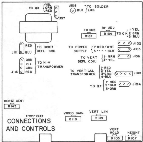
Fig. 5-1 Circuit Board Component Location and Intercabling Diagram.
