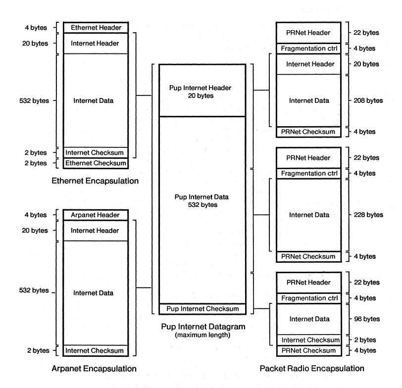
Figure 2. Pup Encapsulation in Various Networks
