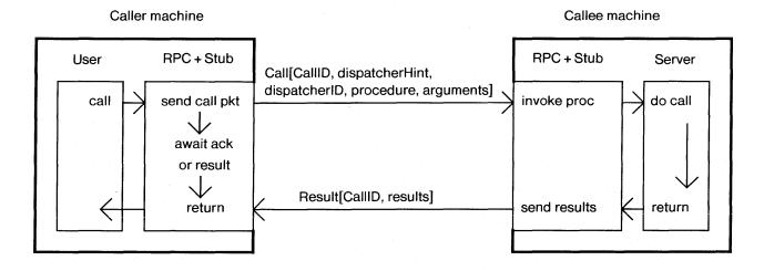
Figure 3: The packets transmitted during a simple call.
