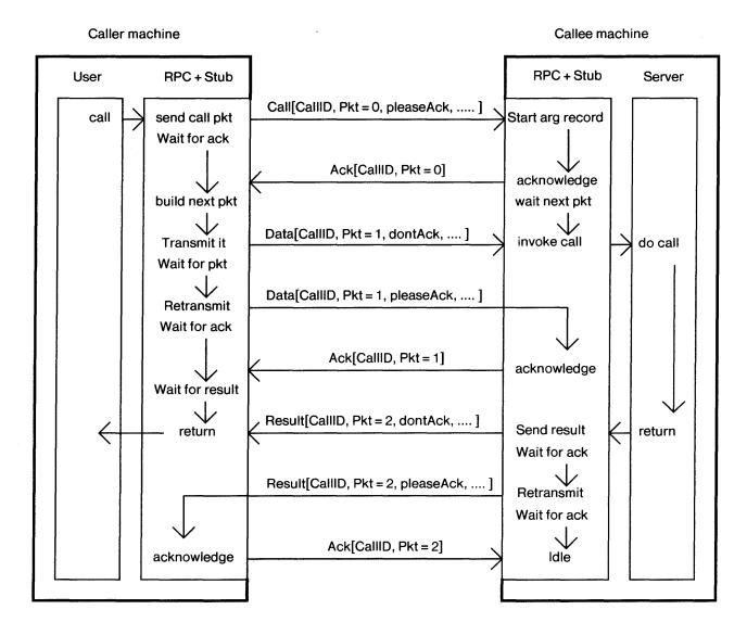
Figure 4: A complicated call. The arguments occupy two packets. The call duration is long enough to require retransmission of the last argument packet requesting an acknowledgement, and the result packet is retransmitted requesting an acknowledgement because no subsequent call arrived.
