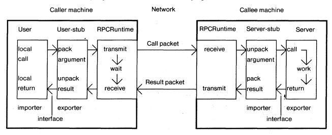
Figure 1: The components of the system, and their interactions for a simple call.
