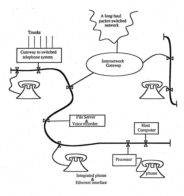
Figure 1: An Ethernet system supporting voice traffic.
