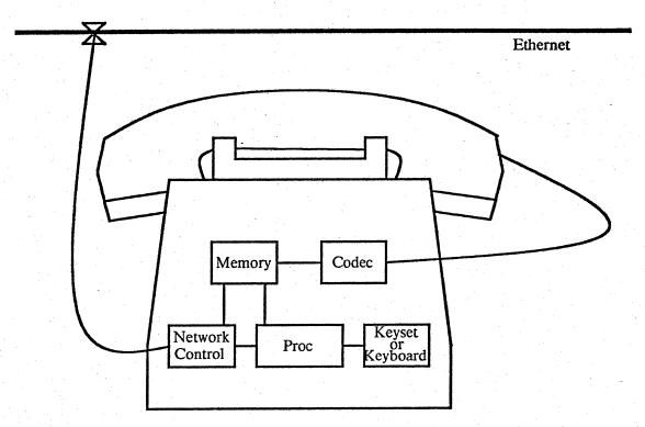
Figure 3: An integrated phone and Ethernet interface.
