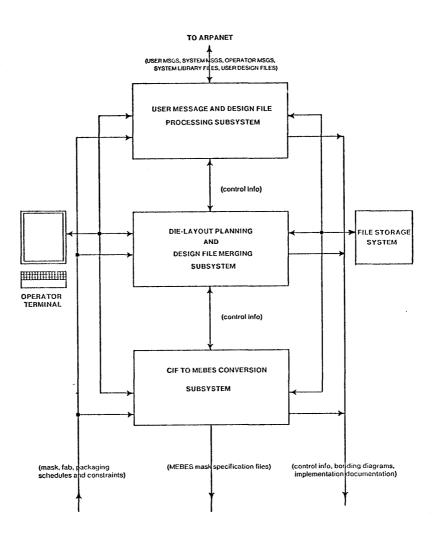
Figure 2. Block Diagram of the VLSI Implementation System
