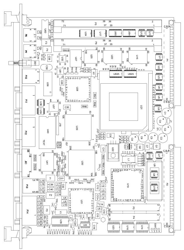
Figure B-1 Assembly Drawing for XVME-658 and XVME-653/31x
