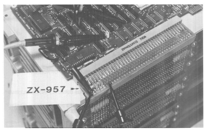
The ZX-957 MULTIBUS extender card plugs into the end of an SBC-604/614 card cage creating an extra slot outside the cage. The card under scrutiny is then plugged into this new slot, thereby eliminating the obstruction caused by the card cage. Every test point on that board can then be easily and quickly reached with probes.
