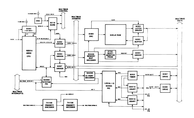
FIG. 2: ZX-85/88 PROCESSOR BLOCK DIAGRAM
