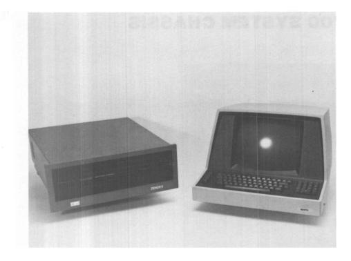
Model 235 Development System. Includes ZX-85 CPU, ZX-200A Disk Controller, and dual 8" floppy disks. Includes ZX-904 for parallel printer and MDS-UPP input/output.
