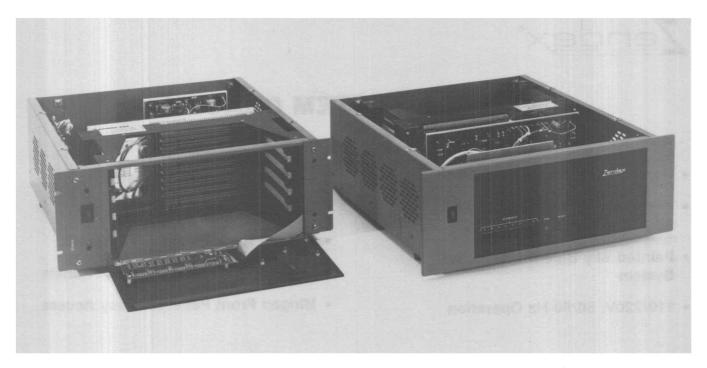
FIG. 2: Two ZX-660A CHASSIS' shown here with cardcase/power supply reversed in one.
