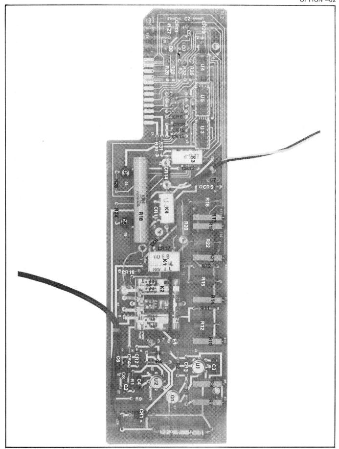
Figure 6-3. OHMS CONVERTER PCB ASSEMBLY
