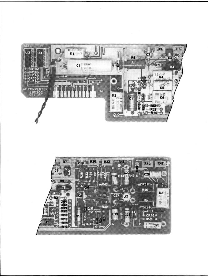
Figure 6-7. AC CONVERTER PCB ASSEMBLY
