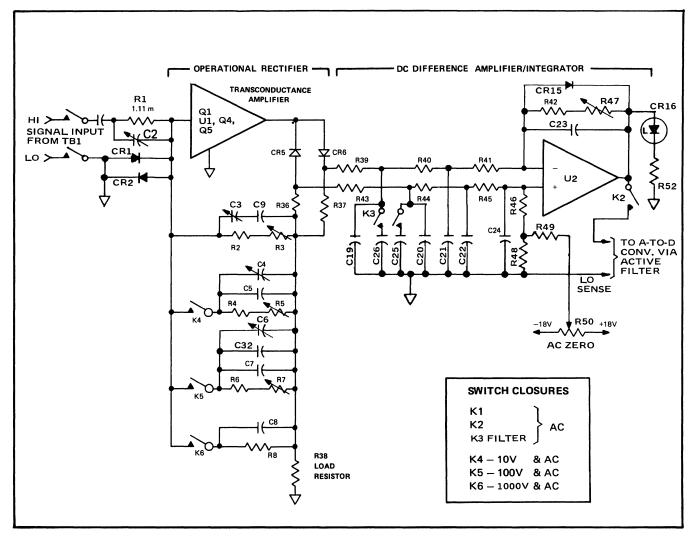
Figure 6-1. CIRCUIT DIAGRAM AC CONVERTER
