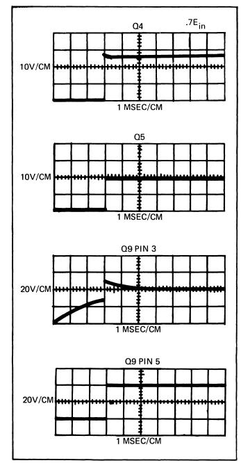
Figure 4-24. DC External Reference Stylized Waveforms
