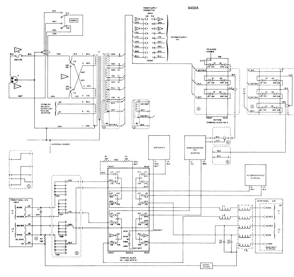
FIGURE 8-2 MODEL 8400A WIRING DIAGRAM (8400A-1000)
