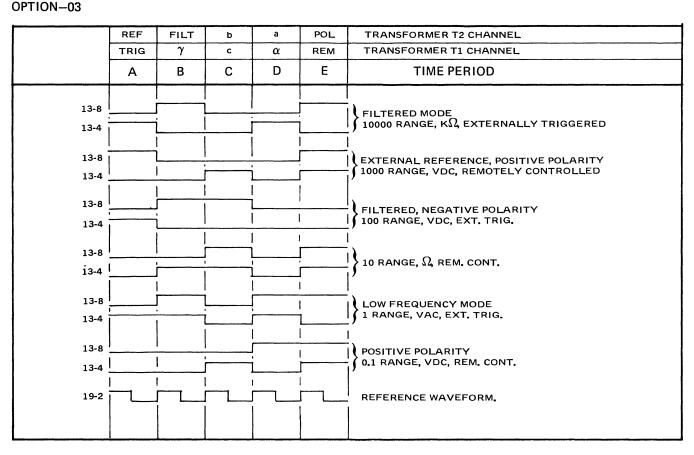
Figure 6-9. EXAMPLE WAVEFORMS FOR TROUBLESHOOTING
