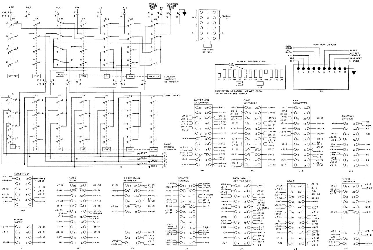
FIGURE 8-16 A14 DISPLAY PCB ASSEMBLY SHEET 1 of 2 (8400A
