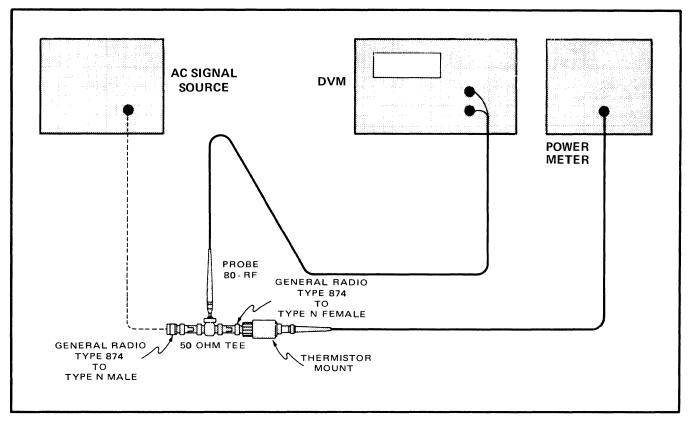
Figure 6-3. HIGH FREQUENCY RESPONSE CHECK
