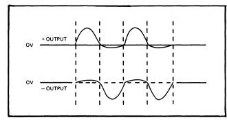
Figure 6-2. RECTIFIER OUTPUT WAVEFORMS
