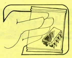
5. USE STATIC SHIELDING CONTAINERS FOR HANDLING AND TRANSPORT
