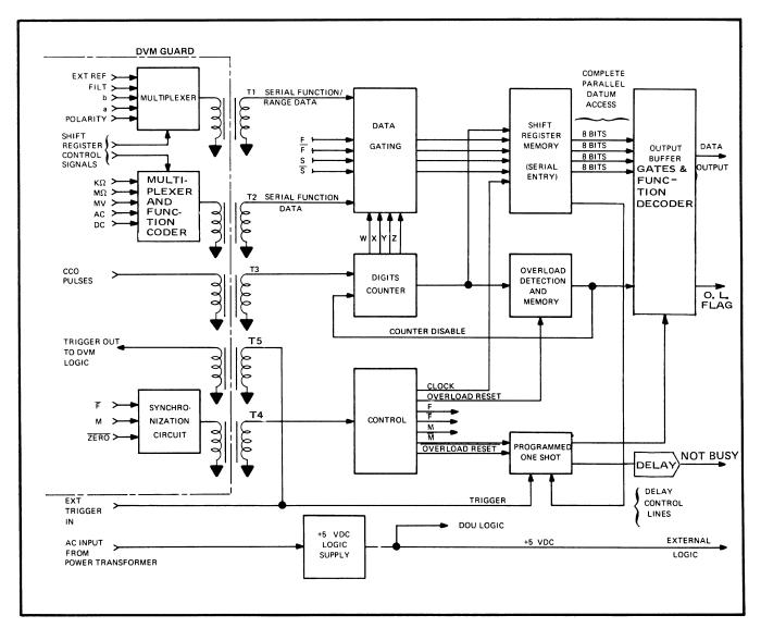
Figure 6-1. DATA OUTPUT UNIT BLOCK DIAGRAM.
