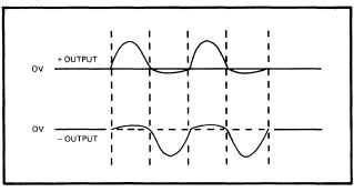
Figure 6-2. RECTIFIER OUTPUT WAVEFORMS
