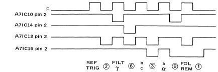
4. **DOU LOAD COMMANDS CORRECT?** Refer to the following load signals. Use the same setup as in part 3 of this figure. A dual-trace scope is useful.
