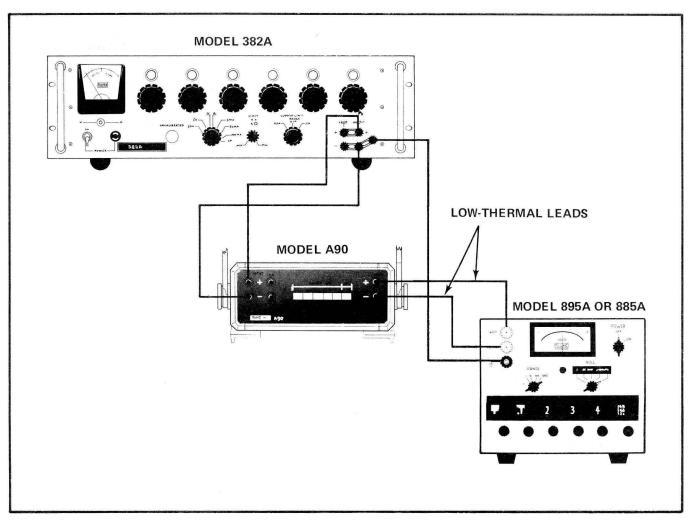
Figure 6-8. EQUIPMENT CONNECTIONS - 10 MA, 100 MA, AND 1000 MA RANGE CHECKS
