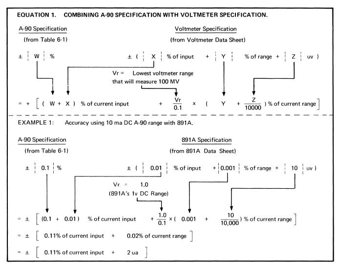
Figure 6-5. EQUATION 1 – COMBINING A90 AND VOLTMETER SPECIFICATIONS (Sheet 1 of 2)
