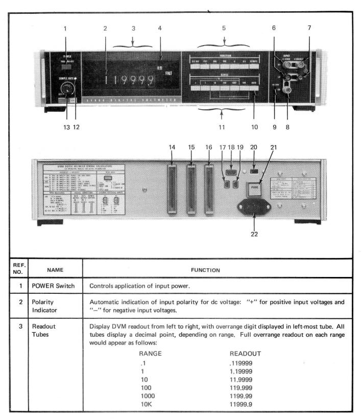
Figure 2-1. CONTROLS, TERMINALS, AND INDICATORS (Sheet 1 of 3)
