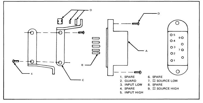
Figure 6-1. REAR INPUT MATING CONNECTOR
