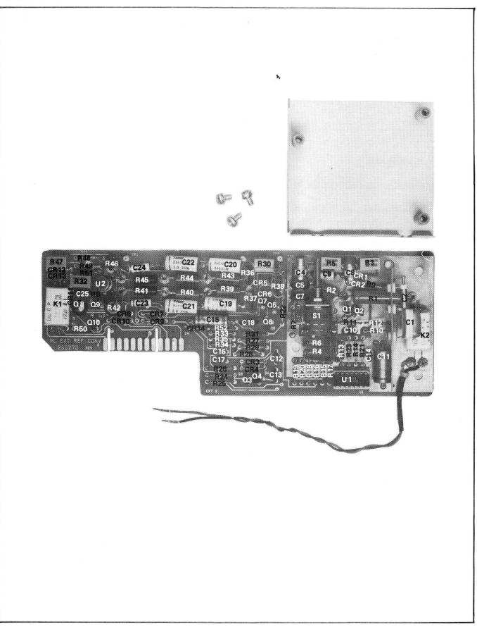
Figure 6-4. AC EXTERNAL REFERENCE PCB ASSEMBLY
