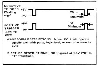
Figure 2-3. DATA OUTPUT UNIT TRIGGER REQUIREMENTS
