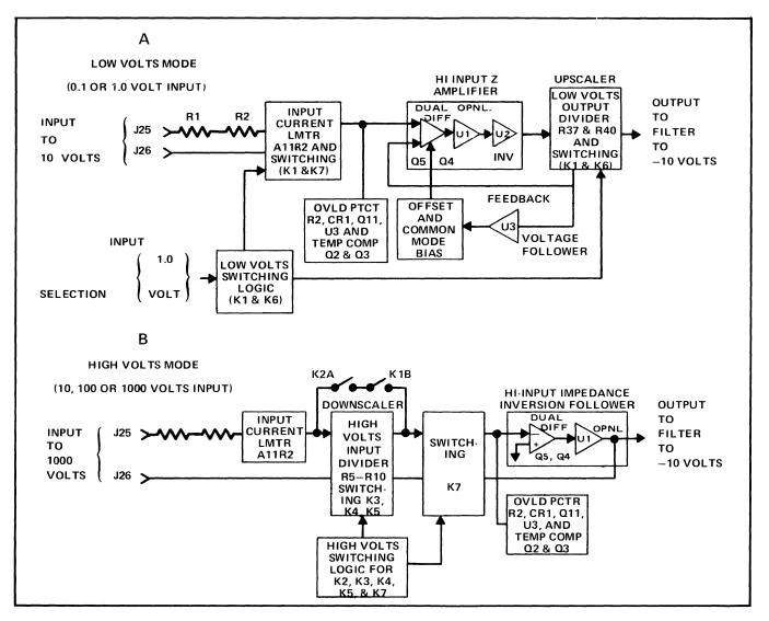
Figure 3-3. BUFFER AMPLIFIER BLOCK DIAGRAM
