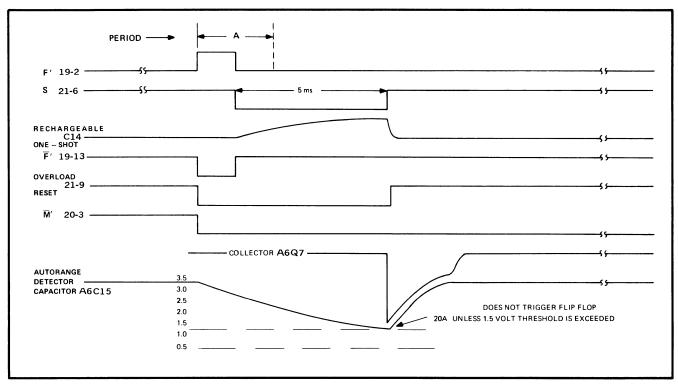
Figure 6-5. CONTROL SIGNAL TIMING DURING AUTORANGE
