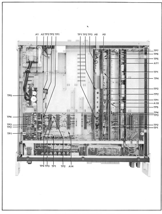
Figure 4-10. ASSEMBLY AND TEST POINT LOCATIONS
