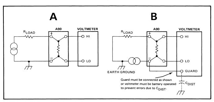
Figure 6-4. EQUIPMENT CONNECTIONS FOR CURRENT MEASUREMENT.
