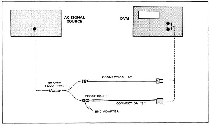
Figure 6-2. LOW FREQUENCY RESPONSE CHECK
