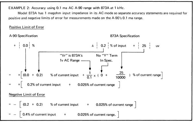
Figure 6-5. EQUATION 1 - COMBINING A90 AND VOLTMETER SPECIFICATIONS (Sheet 2 of 2)
