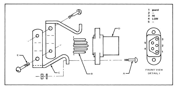
Figure 6-1. EXTERNAL REFERENCE MATING CONNECTOR
