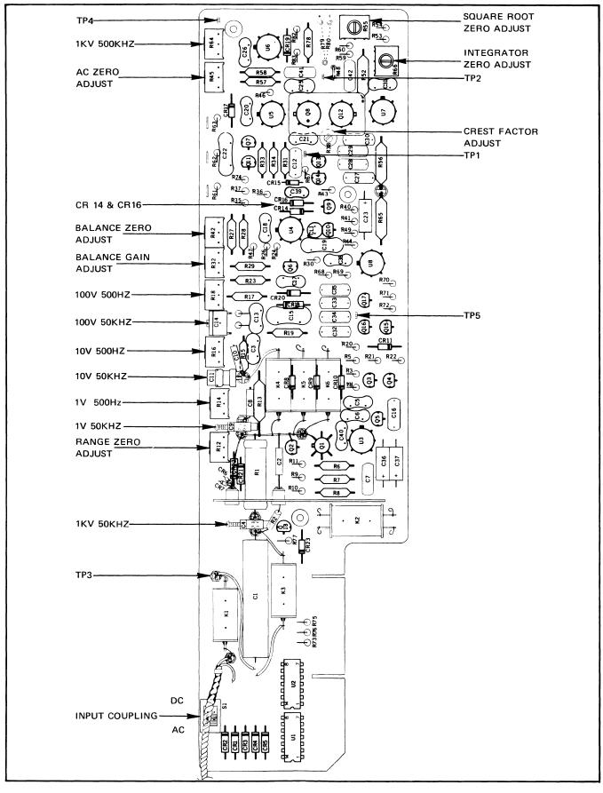
Figure 6-3. RMS CONVERTER ADJUSTMENTS AND TEST POINTS
