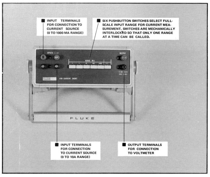
Figure 6-3. MODEL A90 CONTROLS AND TERMINALS.
