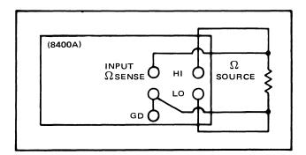
Figure 6-2. EQUIPMENT CONNECTIONS FOR OHMS TEST
