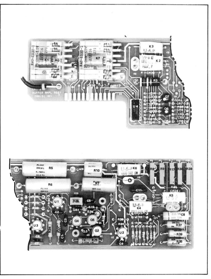
Figure 5-7. BUFFER AMPLIFIER PCB ASSEMBLY
