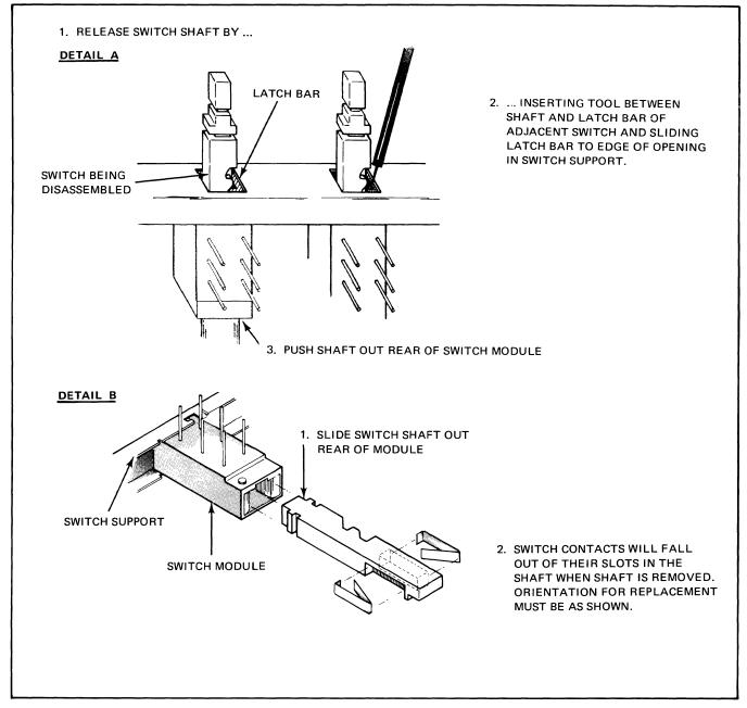
Figure 4-3. PUSHBUTTON SWITCH DISASSEMBLY
