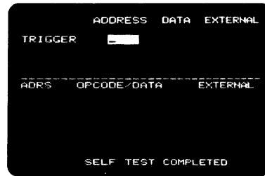
EXAMPLE OF CORRECT POWER-ON DISPLAY
