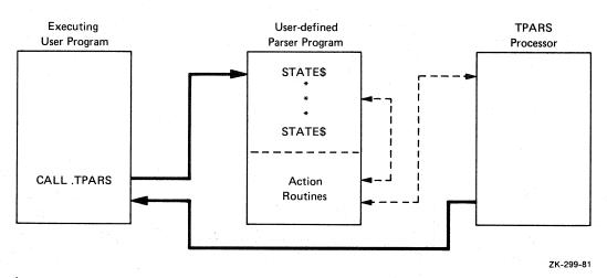
Figure 7-2 Flow of Control When TPARS Is Called from an Executing User Program
