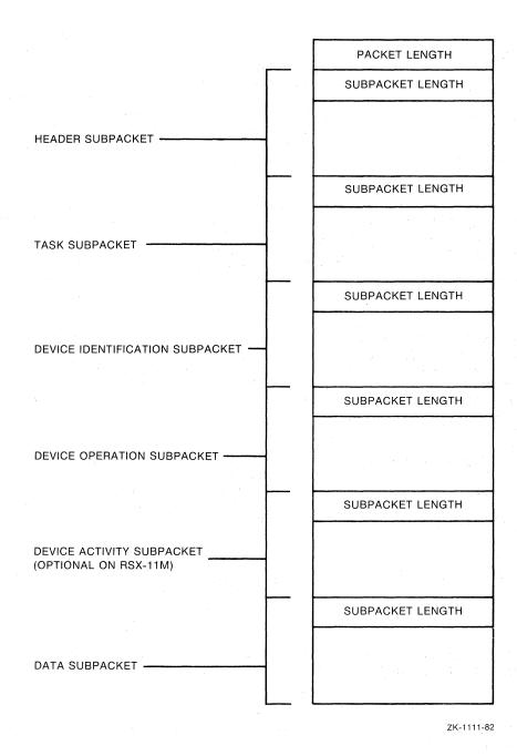
Figure 4-1 - Structure of Error-Logging Packet
