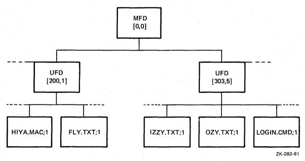
Tasks running under an RSX-11M system access data within files through one of two sets of routines: FCS, or File Control Services, and RMS-11, or Record Management Services. Both FCS and RMS-11 organize information within files. RMS-11 was developed after FCS and allows more complex file organization than is possible with FCS.
