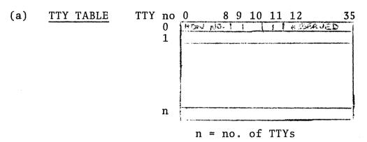
The TTY table consists of n 36 bit entries, where n is the number of TTYs (software lines). Each entry is as follows:
