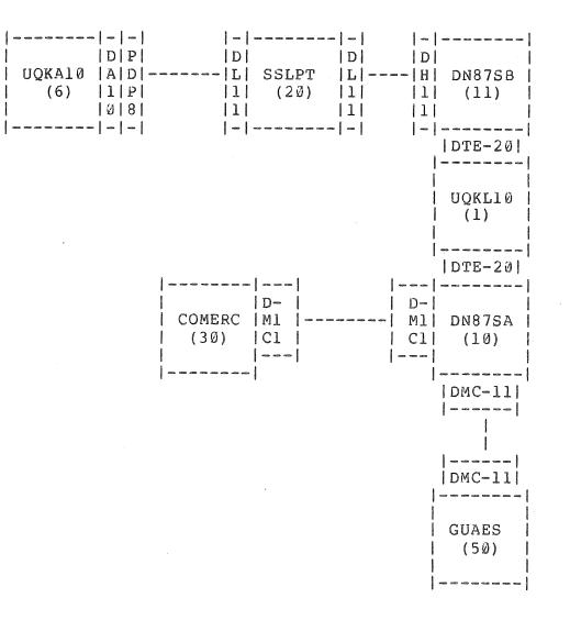
A network is just a collection of computers connected together by some form of data path. Each computer in the network is called a node and each node within the network is known by a unique name and number. On the diagram nodes are represented by the larger boxes while the smaller boxes represent the devices used to control the data paths between the nodes.
