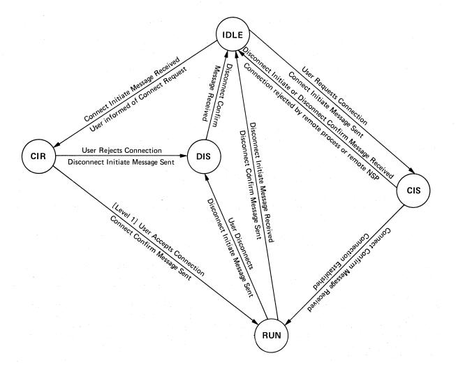
Figure 5-1 Logical Link State Diagram
