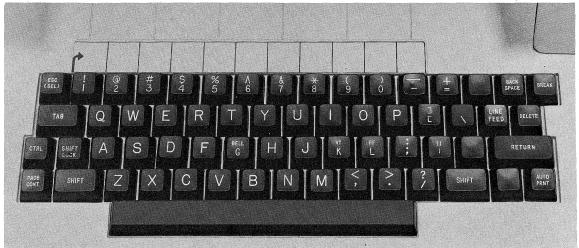
The VT50 keyboard incorporates a special provision for self-explanatory function switches. Its architecture is designed to permit the space above the top row of keys to act as a labeling area for special user-defined Escape sequences. Ten keys are available for this special coding; the labeling can be changed easily to accommodate changing functions and applications.
