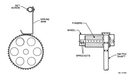
Figure 5-10 Spring Arm Adjustment for PR68B
