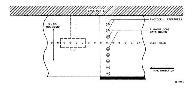
Figure 5-8 Lateral Adjustment of Sprocket Wheel
