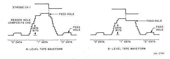
Figure 5-15 Relationship of PR68D/DA Reader Data and Strobe Pulse
