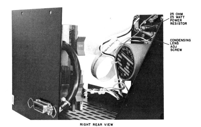
Figure 5-12 PR68D/DA Reader Adjustment Location (Cont)
