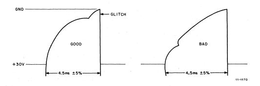
Figure 5-16 Punch Solenoid Waveform
