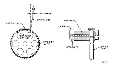
Figure 5-14 Spring Arm Adjustment for PR68D/DA
