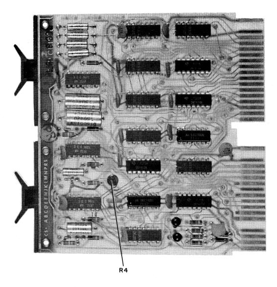
Figure 5-3 M710 Punch Control Adjustment Location
