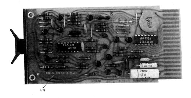
Figure 5-1 M401 Reader Clock Adjustment Location
