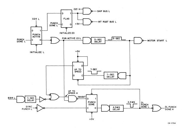
Figure 4-3 M710 Punch Control for PA63, Simplified Logic Diagram
