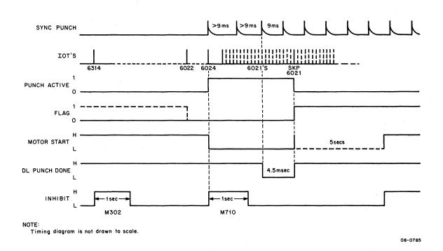
Figure 4-2 Tape Punch Timing Sequence for PA63
