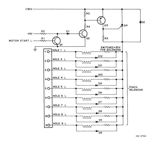
Figure 4-9 Punch Solenoid Control, Simplified Functional Diagram
