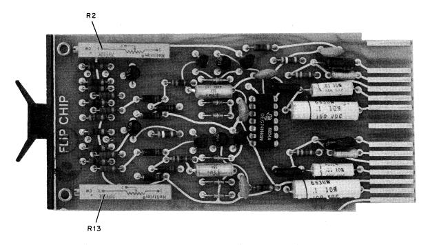
Figure 5-17 M302 Dual Delay Multivibrator Module
