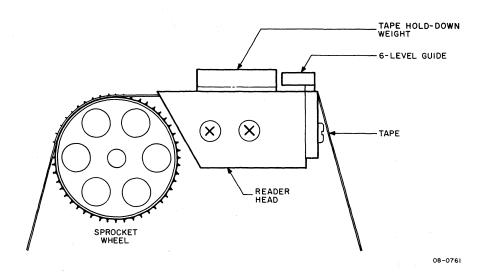
Figure 5-6 6-Level Guide and Reader Head Adjustment
