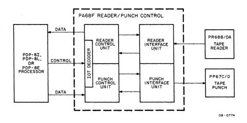
Figure 1-3 Single Reader/Punch System
