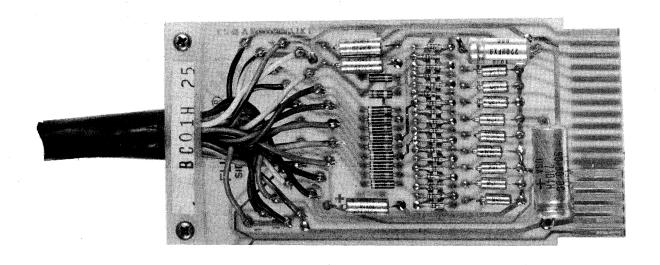
Figure 2-4 M978 Connector Module
