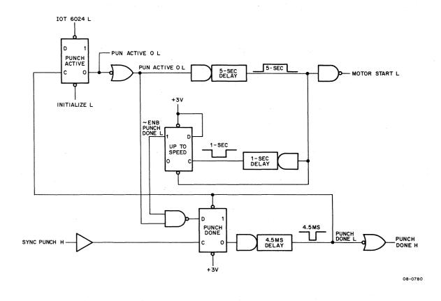
Figure 4-6 M710 Punch Control for PA68F, Simplified Logic Diagram
