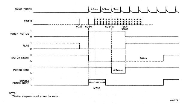
Figure 4-5 Tape Punch Timing Sequence for PA68F
