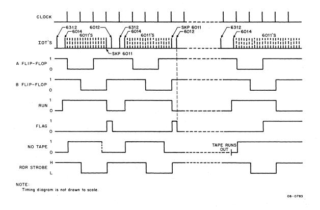
Figure 4-1 Tape Reader Timing Sequence for PA63
