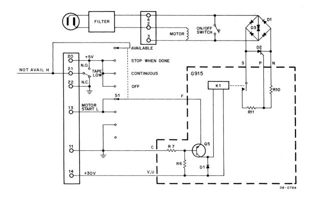
Figure 4-8 Punch Motor Control, Simplified Functional Diagram
