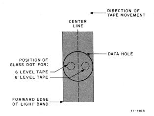
Figure 5-13 Relationship of Data Hole and Photocell for PR68D/DA
