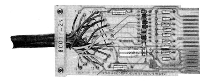
Figure 2-5 M979 Connector Module
