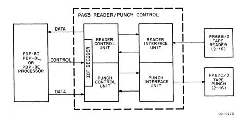
Figure 1-2 Multiple Reader/Punch System
