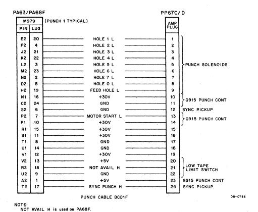
Figure 2-3 PP67C/D Punch/Interface Cable Interconnection
