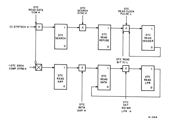
Figure 4-11 DTC Read Data Command, Block Diagram (Revised)
