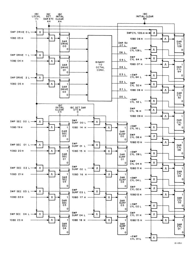
Figure 4-7 RP10 Data Address Register, Block Diagram (Revised)
