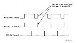
Figure 4-20 RDS DATA WIND Waveform
