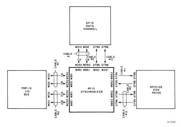
Figure 1-4 RP10/RP01/02 Electrical Interface
