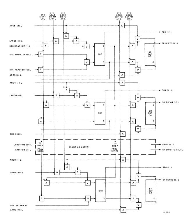
Figure 4-9 RP10 Shift Register, Block Diagram
