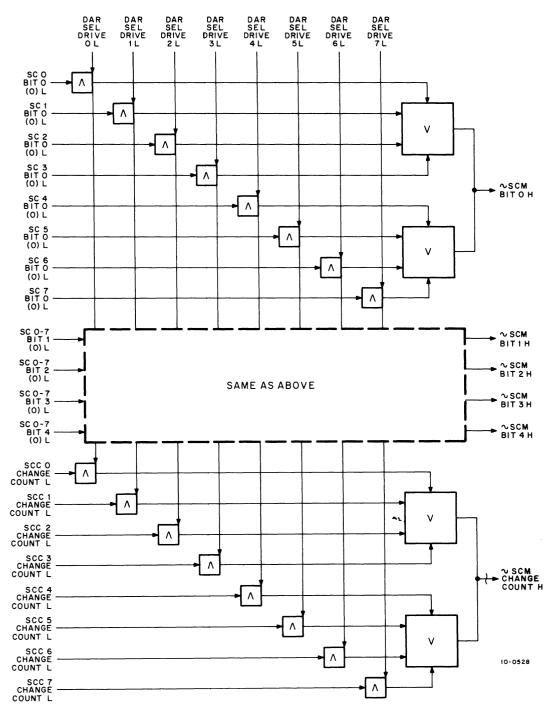
Figure 4-27 RP10 Sector Counter Multiplexer, Block Diagram
