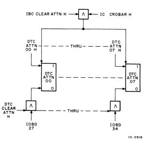
Figure 4-14 DTC Clear Attentions Command, Block Diagram (Revised)
