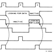
Figure 4-23 Optimum Window Generation Waveforms
