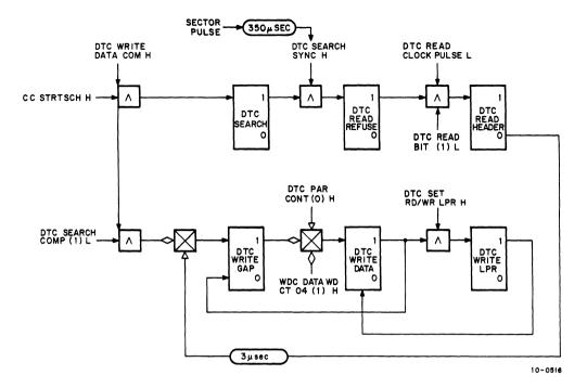
Figure 4-12 DTC Write Data Command, Block Diagram (Revised)
