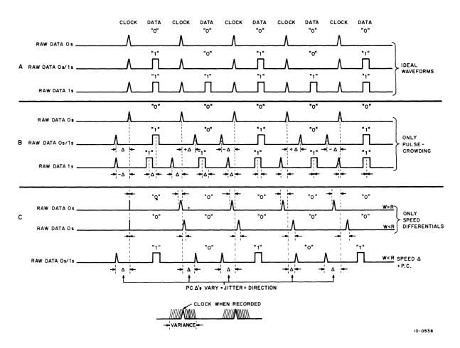
Figure 4-18 Sources of Jitter in Disk Playback
