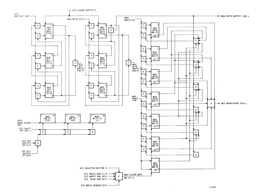
Figure 4-28 RP10 Word Counters Block Diagram (Revised)
