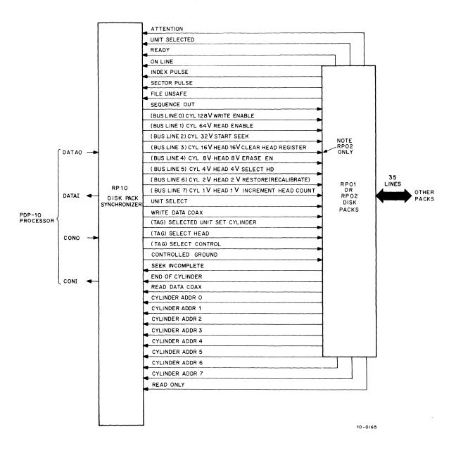
Figure 3-3 RP10/RP01/RP02 Data Control Signals
