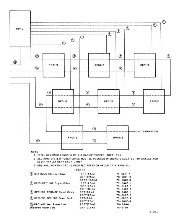
Figure 2-2 RP10-RP01/RP02 Signal and Power Connections
