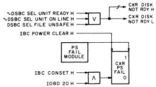
Figure 4-6 RP10 Condition Register, Block Diagram
