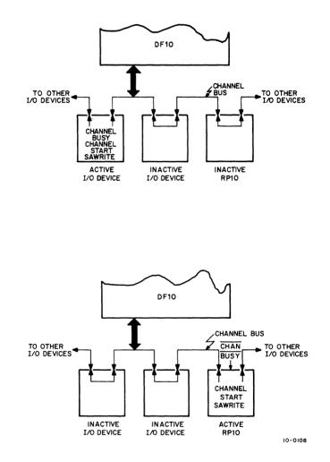
Figure 4-2 RP10 Active and Inactive Functions
