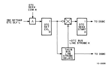
Figure 4-17 DTC Seek Command, Block Diagram
