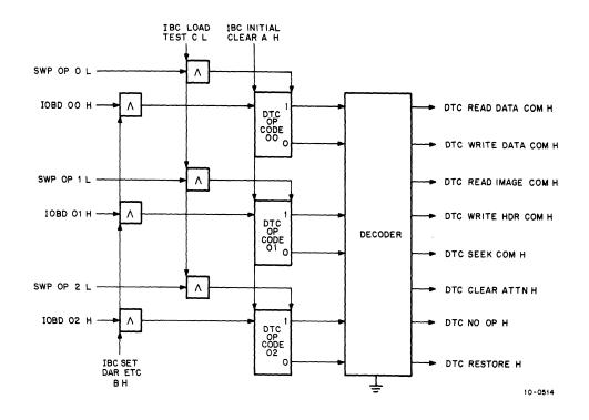
Figure 4-10 DTC OP Decoding, Block Diagram (Revised)
