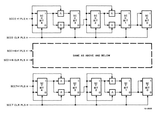
Figure 4-24 RP10 Sector Counter, Block Diagram
