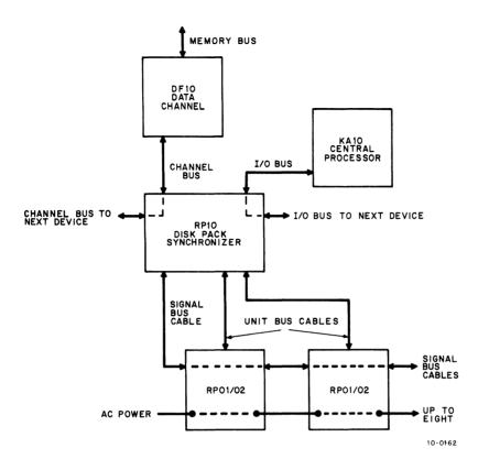
Figure 1-3 RP10/DF10/RP01/RP02/I/O Interface
