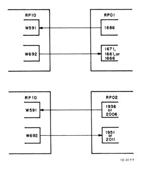
Figure 1-5 RP10 Interface Wiring Diagram
