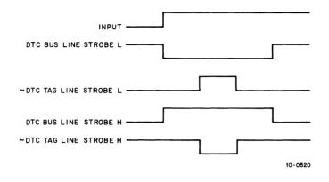
Figure 4-16 Tag and Bus Line Strobe Waveforms
