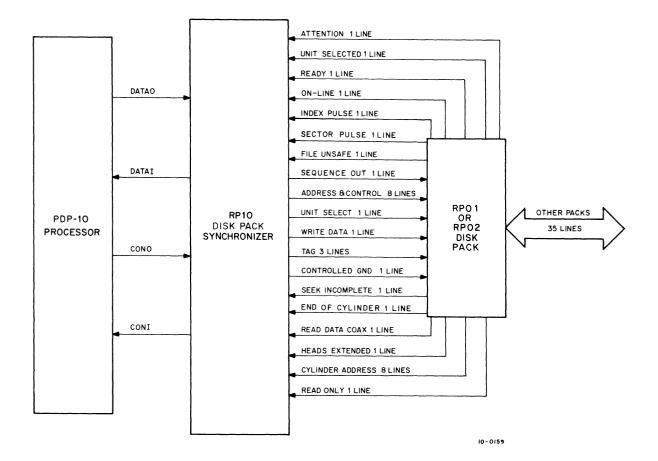
Figure 4-1 RP10 General Block Diagram
