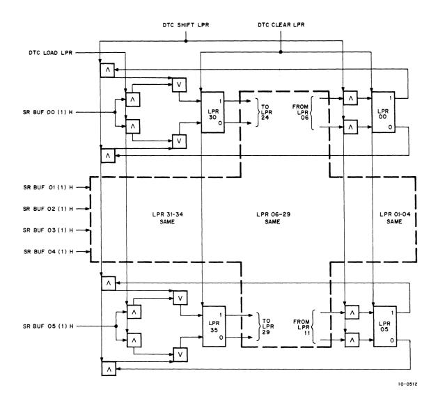
Figure 4-8 RP10 Longitudinal Parity Register, Block Diagram
