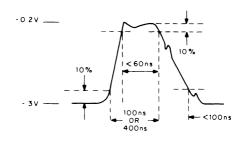
Figure 5-2 R-Series and S-Series Pulses
