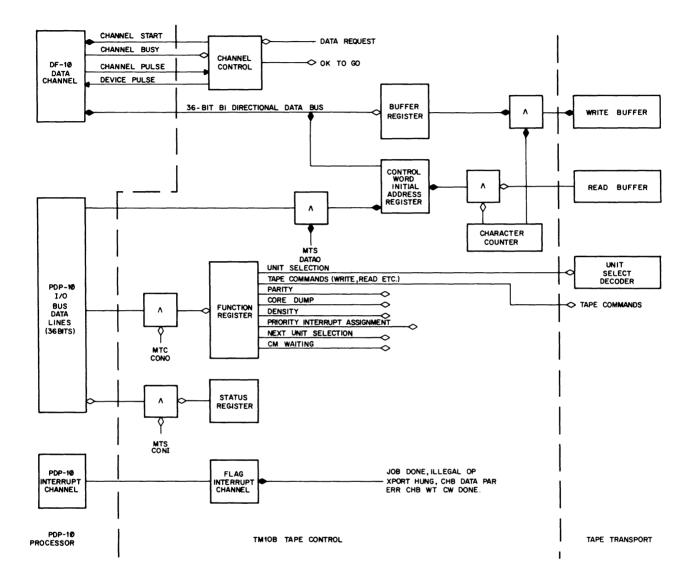
Figure 3-4 TM10B Tape Control Block Diagram
