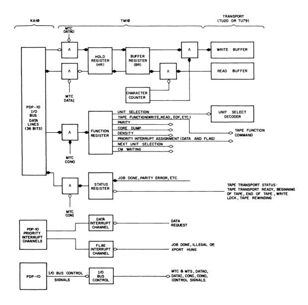
Figure 3-3 TM10A Tape Control Block Diagram
