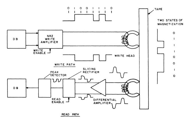
Figure 3-2 Tape Write and Read Signal Flow
