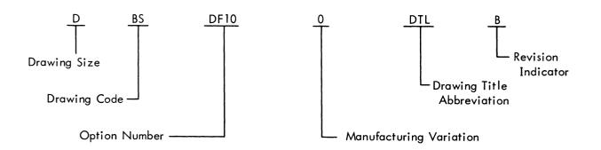
The drawing size, option number, and the drawing title abbreviation are self-explanatory. The manufacturing variation letter identifies the variation that the drawings reflect. For example: 0 reflects drawing applicable to all variations; A reflects the 60 Hz equipment; etc. The drawing code identifies the type of drawing. A list of the common drawing codes follows.
