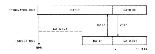
Figure 2-4 DATIP-DATO(B) Cycle (Read, Modify, Write)
