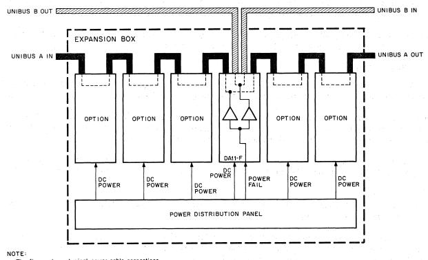
The figure shows typical power cable connections for a DA11-F when installed in a PDP-11 expansion box
