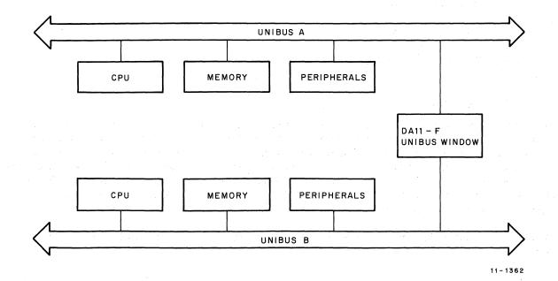
Figure 1-1 Unibus Window, Simplified Block Diagram
