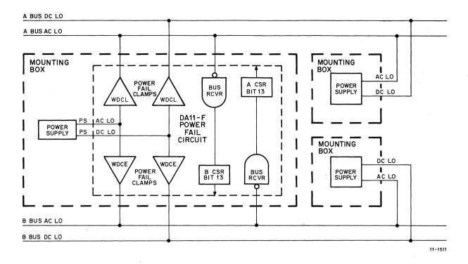
Figure 2-20 Power Fail Simplified Block Diagram
