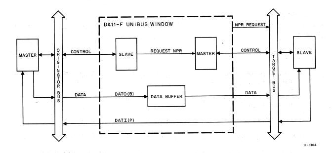
Figure 2-1 Unibus Window, Simplified Block Diagram
