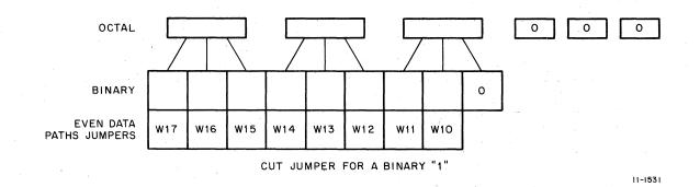
Figure 4-4 Window Starting Address Chart
