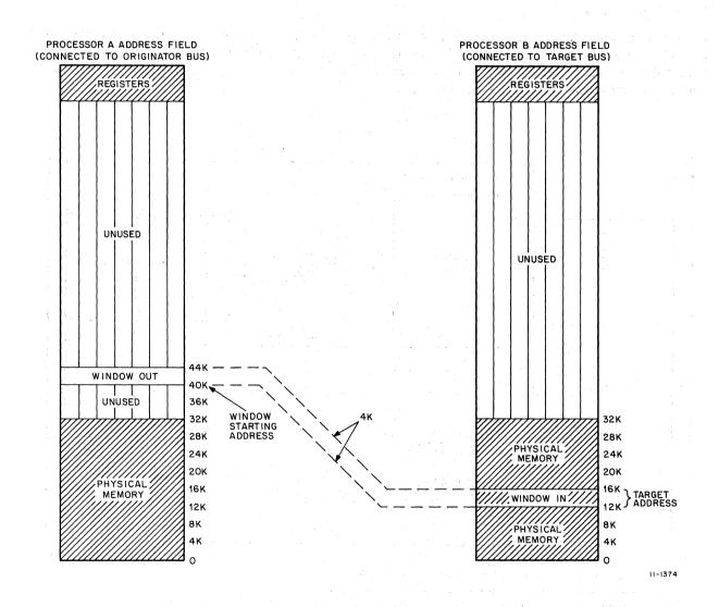
Figure 2-11 Unibus Window Concept
