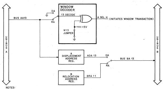
Bits (15:10) employ circuitry similar to that shown above. Bit 13 is shown for simplicity. Bits (09:00) are hardwired from the Displacement Address Register and are not decoded. Bits (17:16) are hardwired from the Relocation Address Register.
