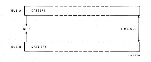
Figure 2-7 Duplex DATIP-DATO(B)/DATIP-DATO(B) Cycles
