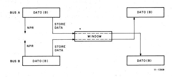
Figure 2-5 Duplex DATO(B)/DATO(B) Cycles
