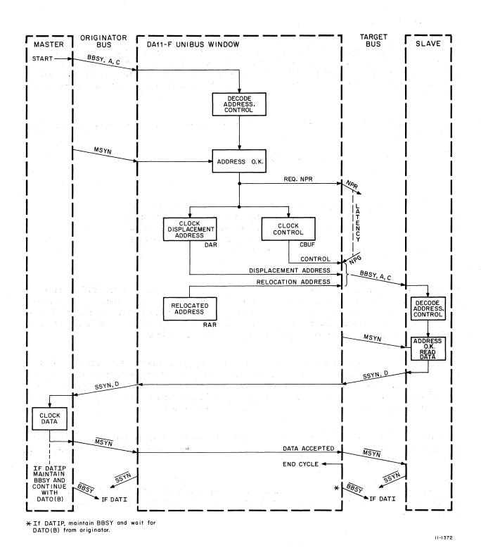
Figure 2-9 Detailed DATI, DATIP Cycle
