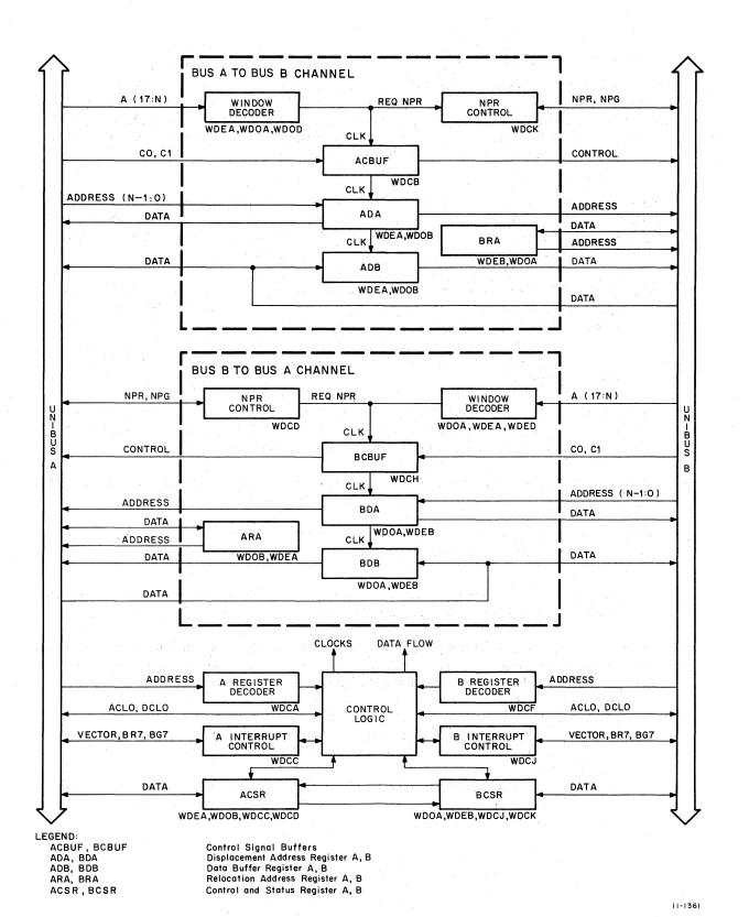
Figure 2-10 DA11-F Functional Block Diagram
