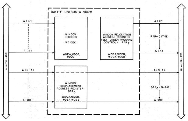
$RAR_T$  (17:N) = Window Relocation Address Register Target. DAR<sub>0</sub> (N-1:O) = Window Displacement Address Register Originator. Target Address =  $RAR_T$  (17:N) +  $DAR_0$  (N-1:O).
