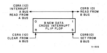
Figure 3-2 Cross Interrupt Logic
