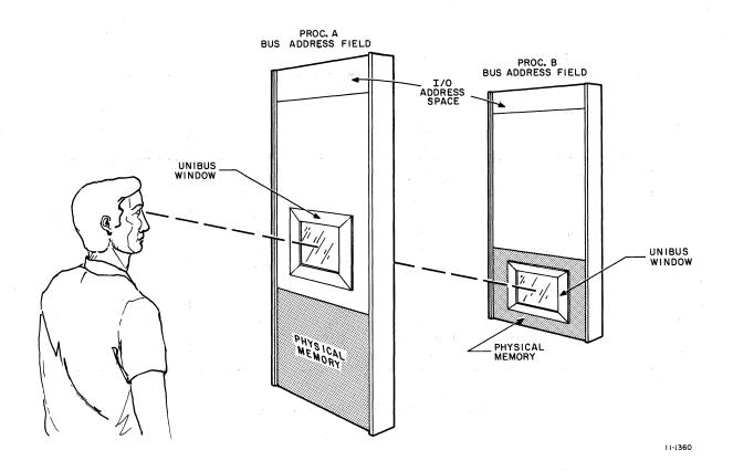
Figure 1-2 Relocated Target Address Concept
