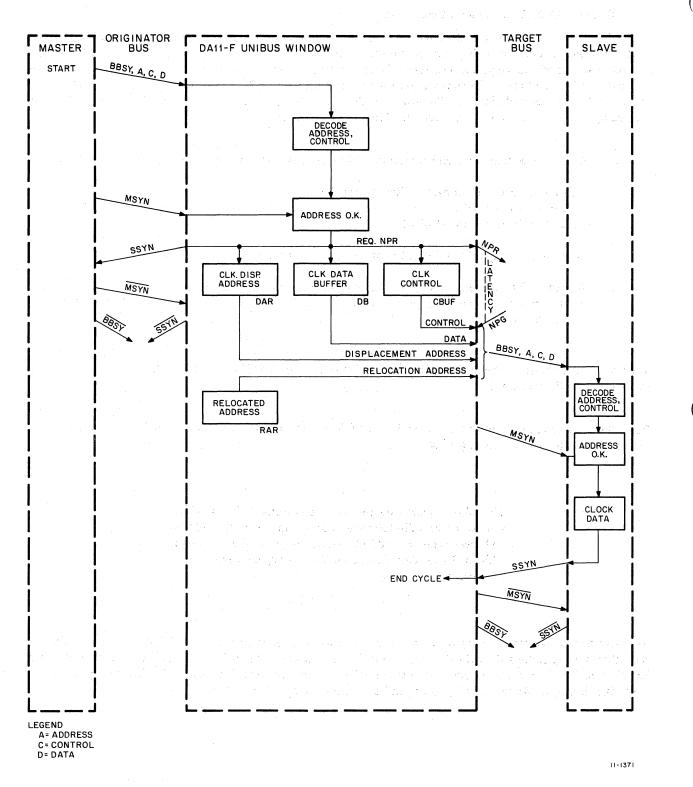
Figure 2-8 Detailed DATO, DATOB Cycle
