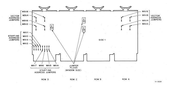
Figure 4-3 Data Path Module Jumper Locations
