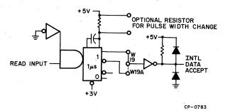
Figure 3-71 INTL DATA ACCEPT Circuit
