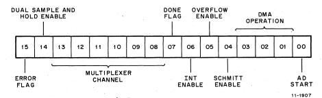
Figure 3-12 A/D Status Register Bit Assignments
