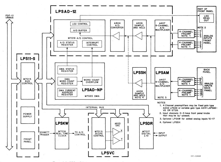
Figure 1-2 LPS11-S Laboratory Peripheral System and Options, Block Diagram
