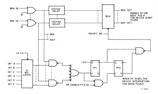
Figure 3-8 Bus Grant Inhibit Logic
