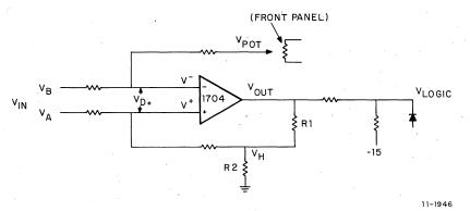
Figure 3-51 Schmitt Trigger Simplified Schematic Diagram
