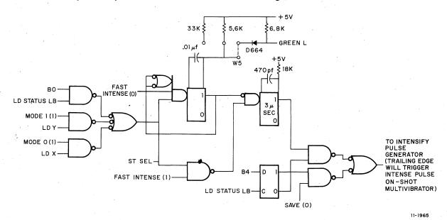
Figure 3-57 Deflection Delay Circuit
