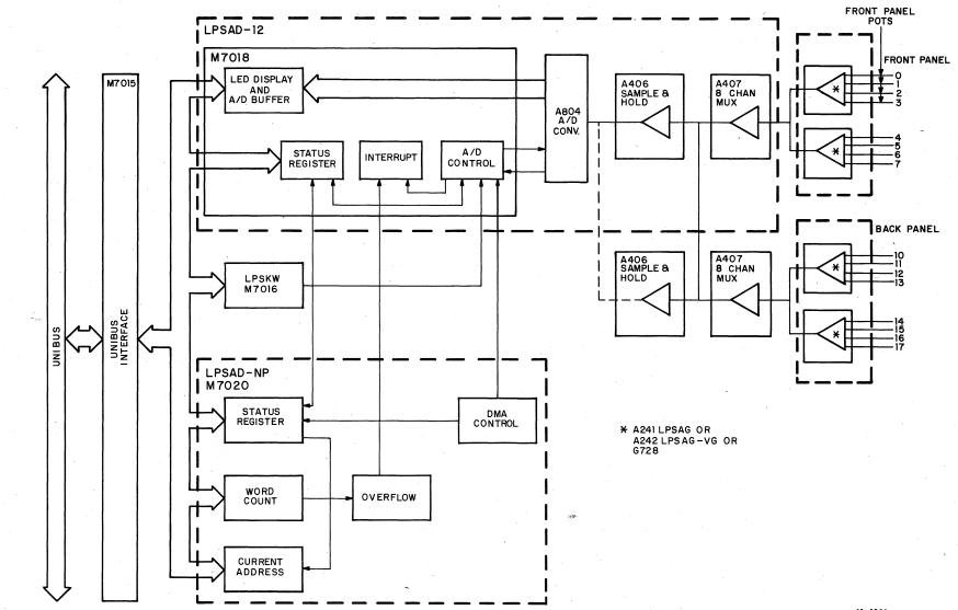
Figure 3-11 A/D Converter Block Diagram
