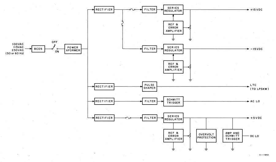
Figure 3-77 Power Supply Block Diagram
