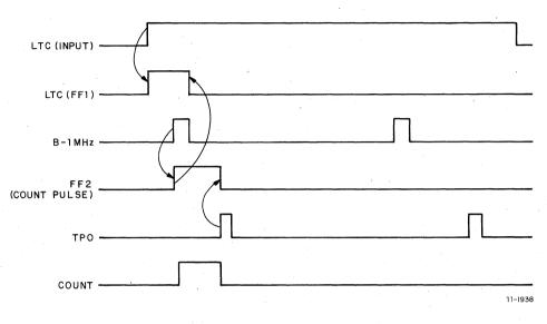
Figure 3-43 Count Pulse Timing Diagram
