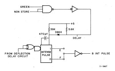
Figure 3-59 Intensify Pulse Generator
