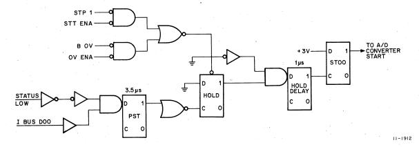
Figure 3-17 Program and Clock A/D Start Logic
