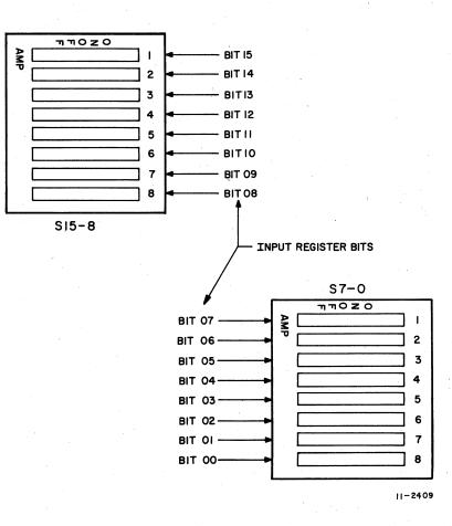
Figure 3-67 Input Register Interrupt Switches
