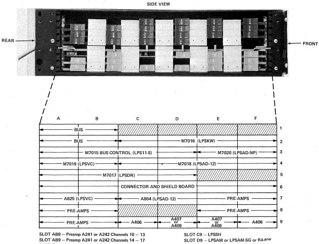
SLOT EF7 - Preamp A241 or A242 Channels 0 - 3
