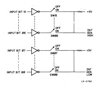
Figure 3-70 LPSDR-A Interrupt Structure for Input Register
