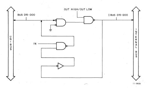
Figure 3-4 Internal Bus Logic
