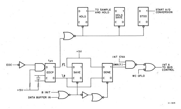
Figure 3-18 Basic EOCP Functions and Interrupt Logic
