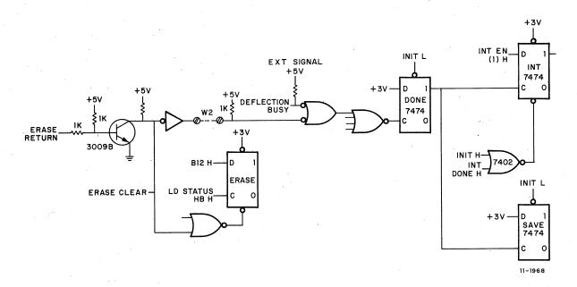
Figure 3-60 Storage Scope Logic
