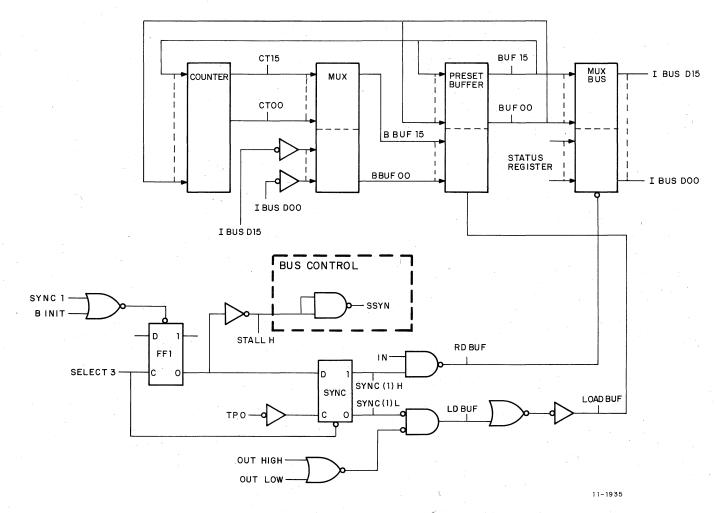
Figure 3-40 Clock Preset Buffer Gating
