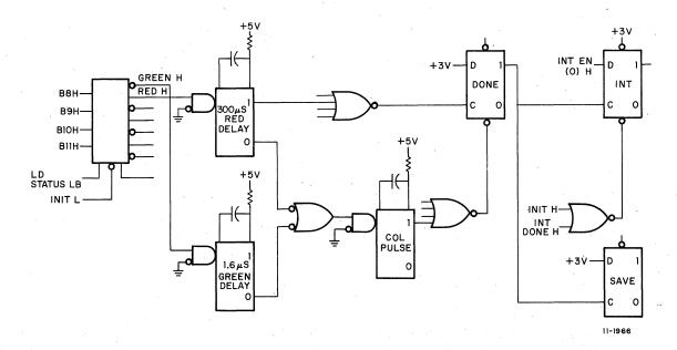
Figure 3-58 Delay Circuitry for VR20 Setup Time
