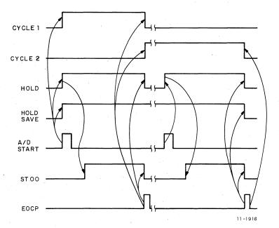
Figure 3-21 Dual Sample-and-Hold Timing
