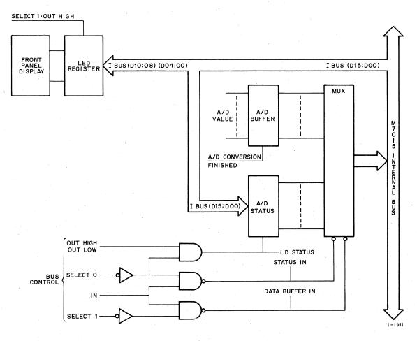
Figure 3-16 A/D Addressing Logic
