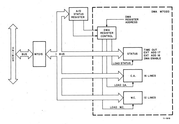
Figure 3-24 DMA Register Control Block Diagram
