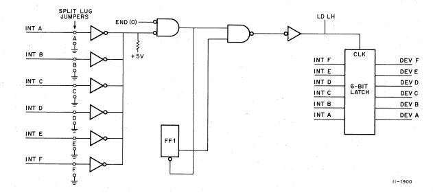
Figure 3-6 6-Bit Latch Logic
