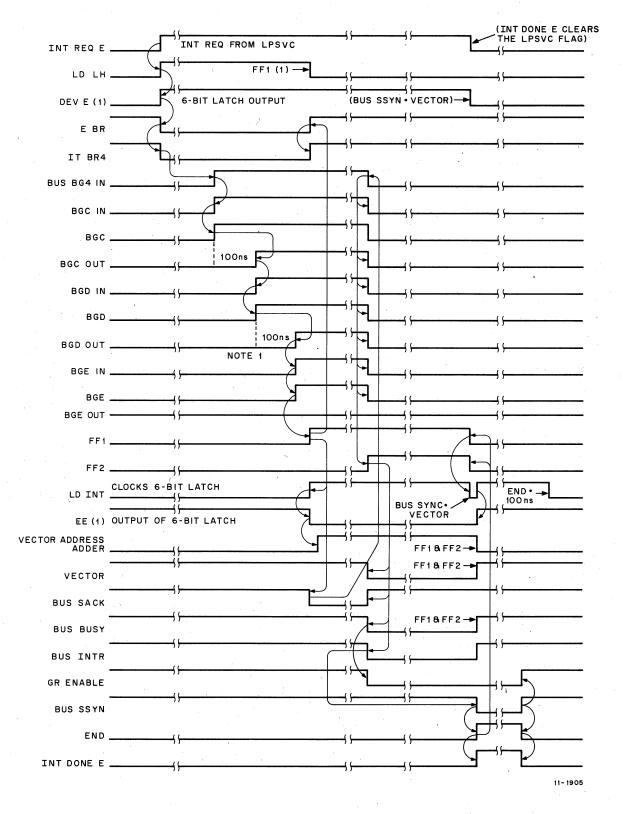
Figure 3-10 Interrupt Timing
