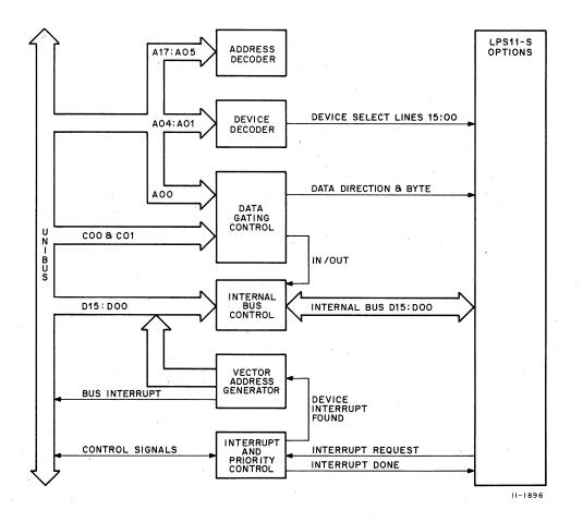
Figure 3-1 Bus Control Block Diagram
