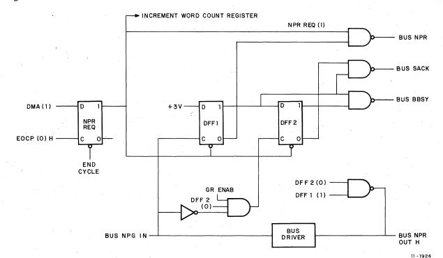
Figure 3-29 DMA Bus Control Logic
