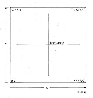
Figure 3-54 Display Control Grid Coordinate Scheme
