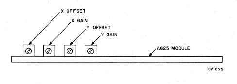
Figure 4-1 Location of A625 Offset and Gain Adjustments
