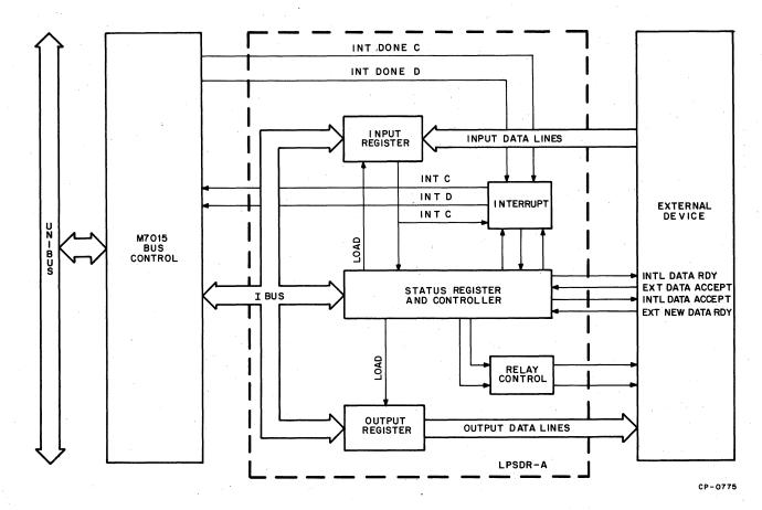
Figure 3-62 Digital I/O Block Diagram
