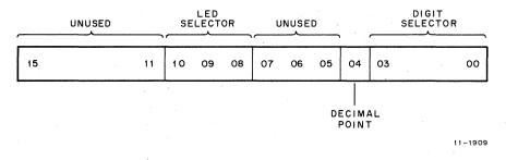
Figure 3-14 LED Register Bit Assignments as a Write-Only Address
