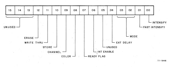
Figure 3-53 Display Control Status Register Bit Assignments
