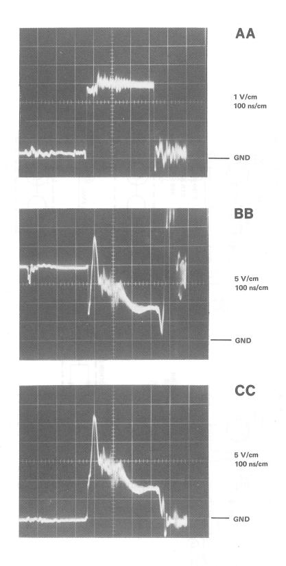
Figure 5-9 Drive Module Waveforms (Sheet 1 of 3)
