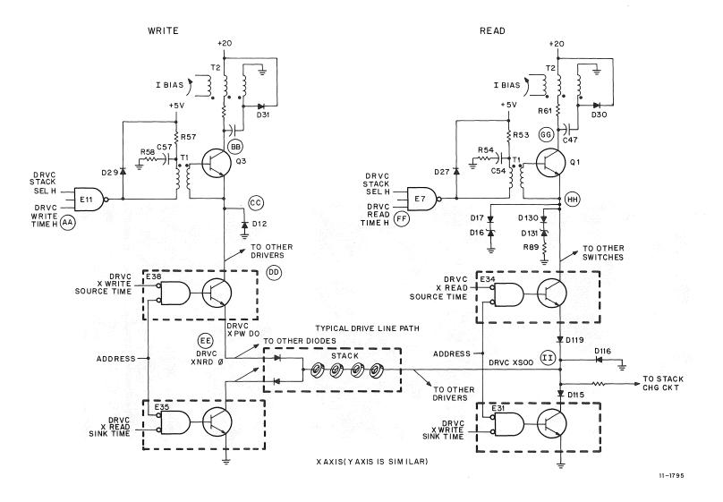
Figure 5-8 Typical Read/Write Drive Circuit
