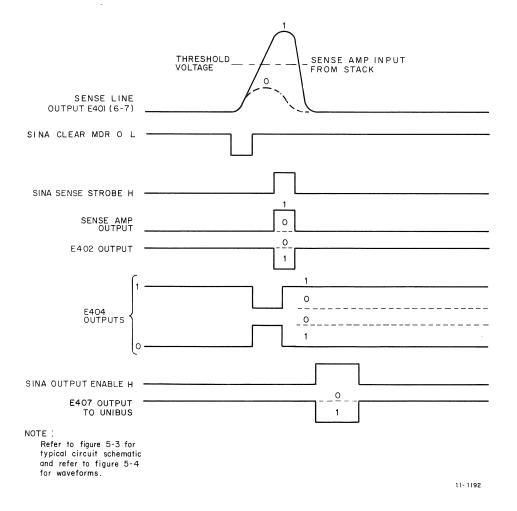
Figure 3-7 Sense Operation Timing Diagram
