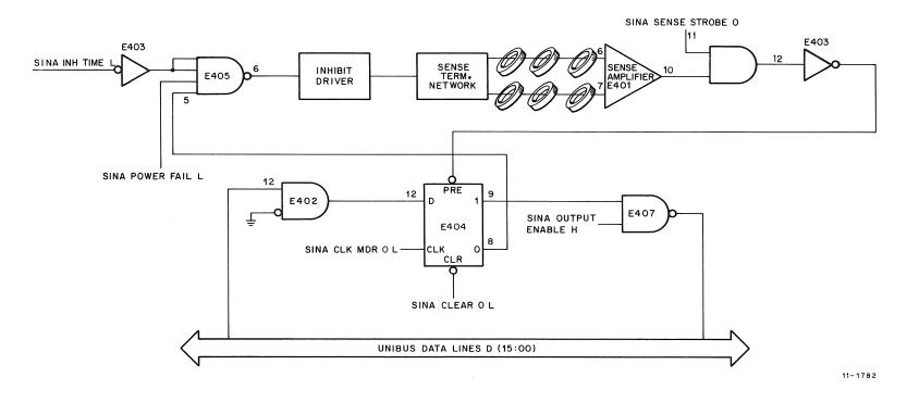
Figure 3-6 Interconnection of Unibus, Data Register, Sense Amplifier and Inhibit Driver
