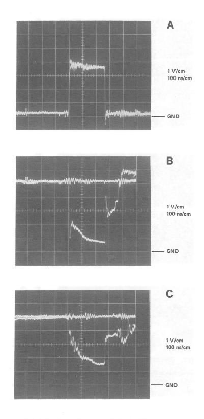
Figure 5-7 Sense Inhibit Module Waveforms (Sheet 1 of 4)
