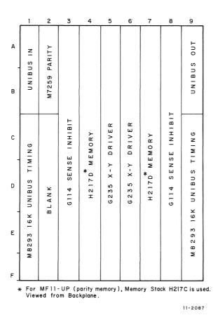
Figure 1-1 Module Utilization Chart
