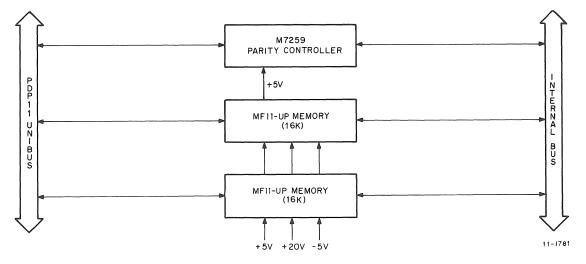
Figure 4-1 Parity Controller Internal Bus
