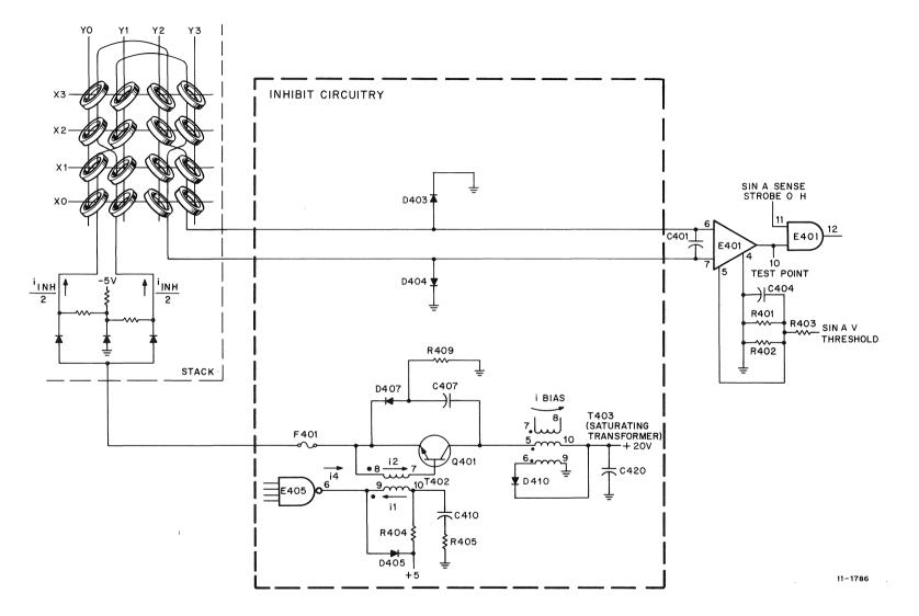
Figure 3-9 Sense Amplifier and Inhibit Driver
