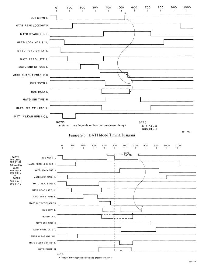
Figure 2-6 DATIP Mode Timing Diagram
