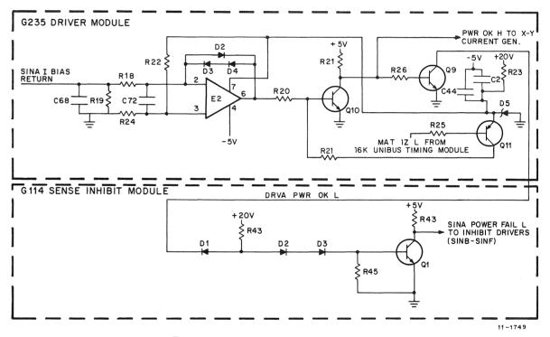
Figure 2-3 Bias Current Detection Circuit
