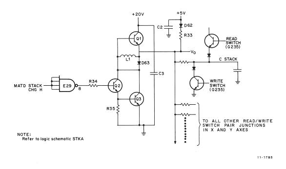
Figure 3-11 Stack Charge Circuit
