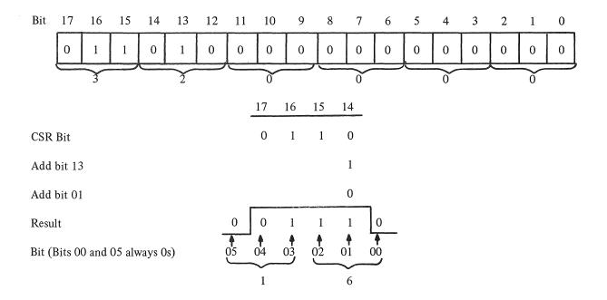
*Example:* Assume a starting address of 52K ( $320000_8$ ) is desired. The example illustrates how the CSR parity address is determined.
