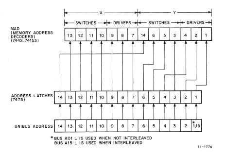
Figure 2-4 Switch and Driver Selection
