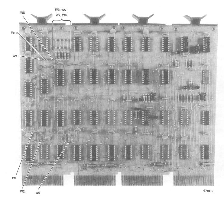
NOTE: W1, W2, W8, W9, and W10 ARE SELECTED FOR INTERLEAVED OR NON-INTERLEAVED OPERATION' W3, W4, W5, W6, and W7 ARE SELECTED FOR STARTING ADDRESS REFER TO PRINT MATA FOR JUMPER CONFIG— URATION
