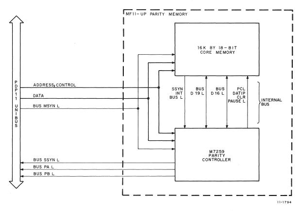
Figure 4-2 Parity Controller Block Diagram
