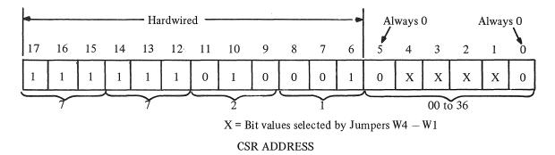
Table 4-4 shows the CSR addresses for all possible memory starting addresses and their jumper configurations. For example, if the lowest address memory responds to is 28K, the jumpers are cut for address 722110. If the lowest address memory responds to is 32K, the jumpers are also cut for address 772110. This is because the CSR addresses are assigned on a basis of 8K of memory. Thus, there are 16 unique addresses in the table.
