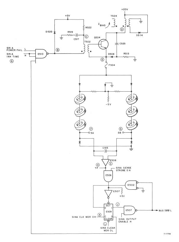
Figure 5-6 Typical Sense/Inhibit Circuit (D00)
