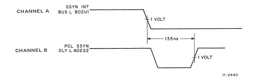
Figure 5-4 SSYN DLY L Timing Waveform
