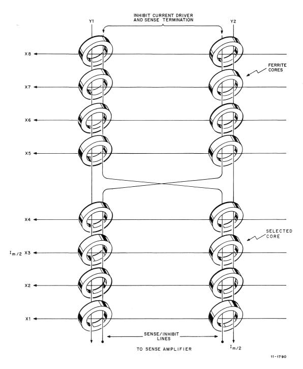
Figure 3-1 Three-Wire Memory Configuration
