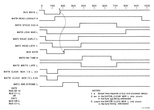
Figure 2-7 DATO, DATOB Mode Timing Diagram
