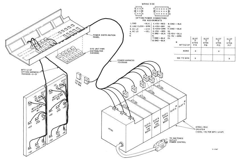
Figure 5-1 New MF11-U Power Distribution System
