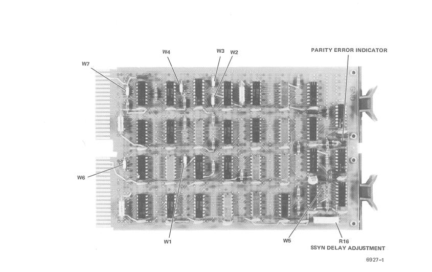
Figure 5-14 M7259 Parity Control Module
