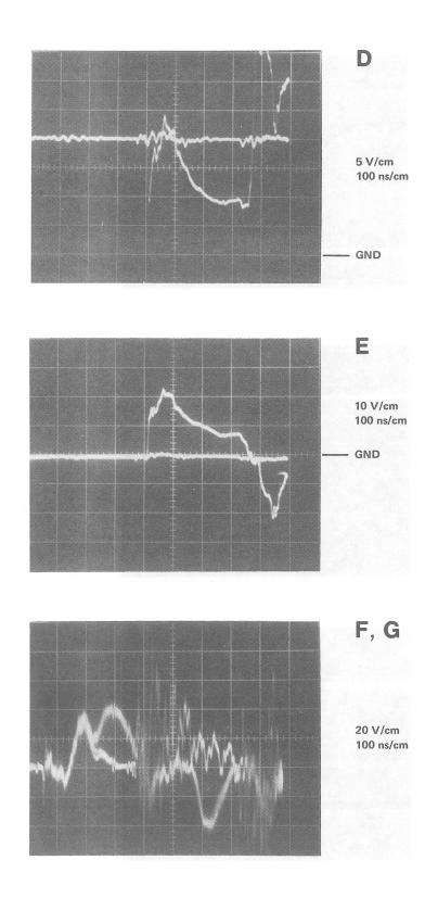
Figure 5-7 Sense Inhibit Module Waveforms (Sheet 2 of 4)
