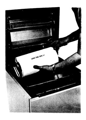
Figure 3-3 Inserting Roll Paper
