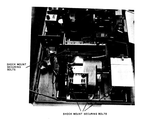
Figure 4-4 35 ASR and 35 KSR Left-Side Shock Mount Bolts
