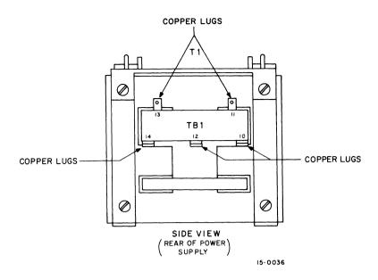
Figure 4-7 Transformer Terminal Connector Diagram (Side View)
