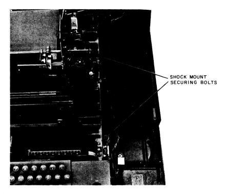
Figure 4-3 35 ASR and 35 KSR Right-Side Shock Mount Bolts
