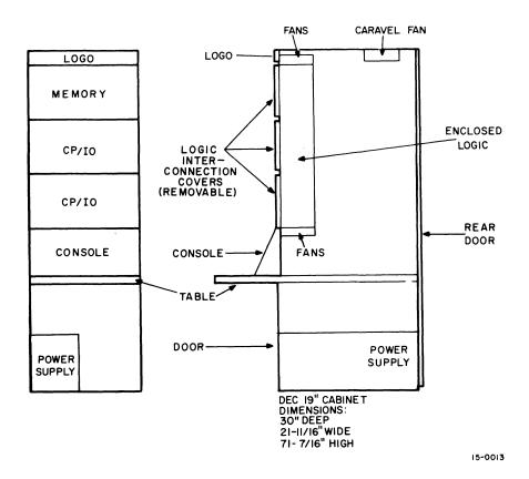
Figure 2-1 PDP-15/10 System Configuration Diagram
