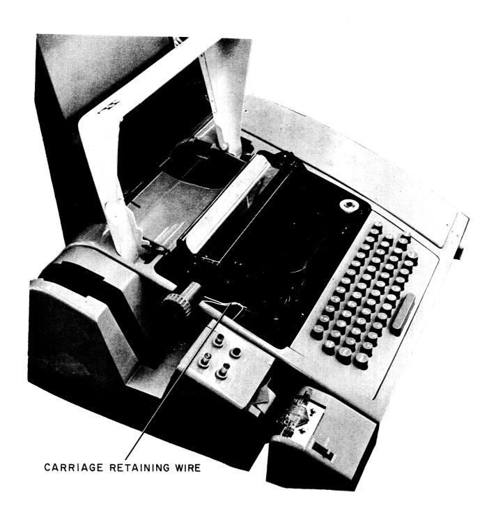
Figure 4-2 33 ASR and 33 KSR Carriage Retaining Wire Location
