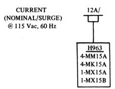
Figure 3-4 Memory Multiplexer Cabinet Power Requirements
