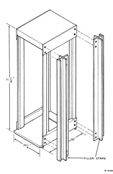
Figure 4-1 Cabinet Bolting Diagram
