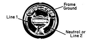
Figure 3-5 Hubbell Wall Receptacle Connector Diagram
