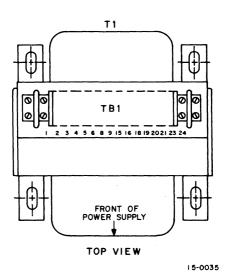
Figure 4-6 Transformer Terminal Connector Diagram (Top View)
