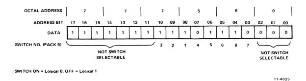
Figure 4-10 DL11-W Device Address Selection
