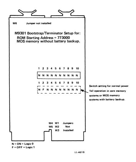
Figure 5-9 Typical Jumper Placement and Switch Settings of Modules (Sheet 4 of 9)
