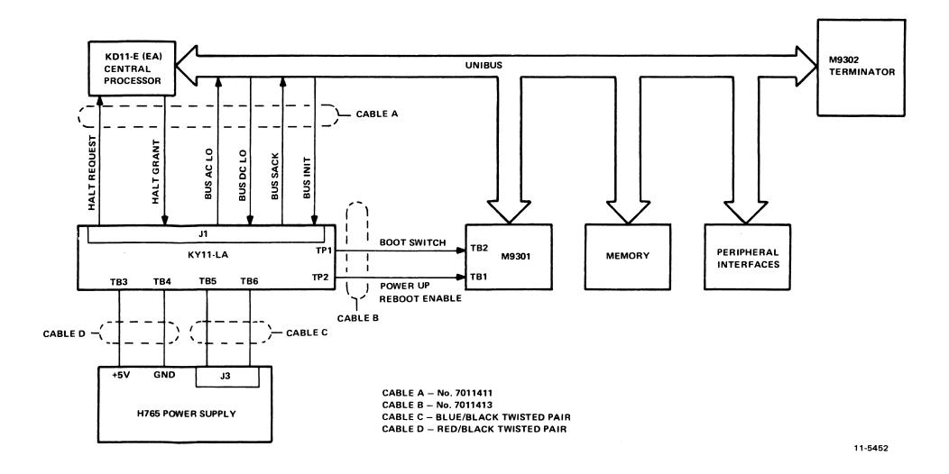
Figure 3-2 PDP-11/34 System Interconnections (BA11-K Mounting Box)
