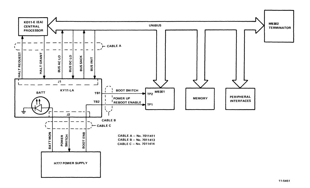
Figure 3-1 PDP-11/34 System Interconnections (BA11-L Mounting Box)
