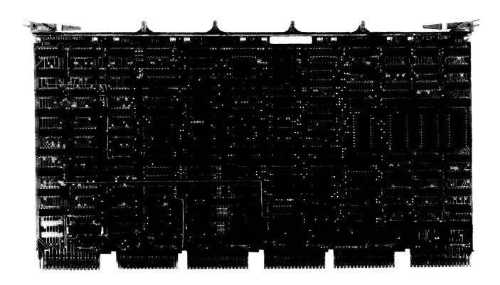
Figure 1-3 KD11-E Central Processor Unit (M7265 Module)
