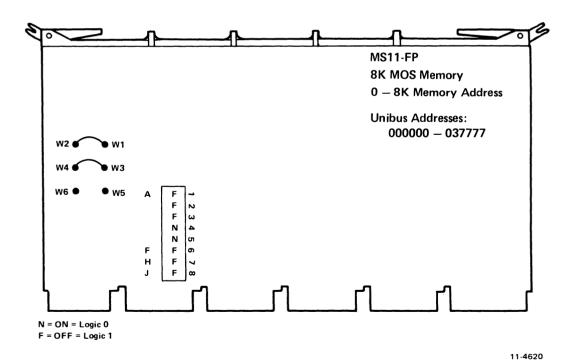
Figure 5-9 Typical Jumper Placement and Switch Settings of Modules (Sheet 5 of 9)
