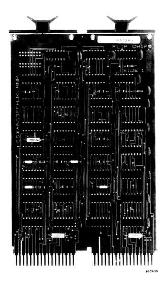
Figure 1-11 M7850 Parity Controller
