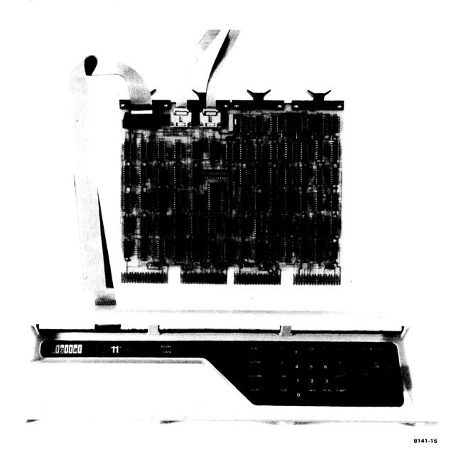
Figure 1-13 KY11-LB Console and Interface Module
