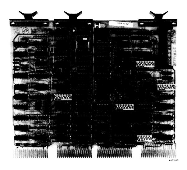
Figure 1-12 DL11-W Serial Line Interface and Real-Time Clock
