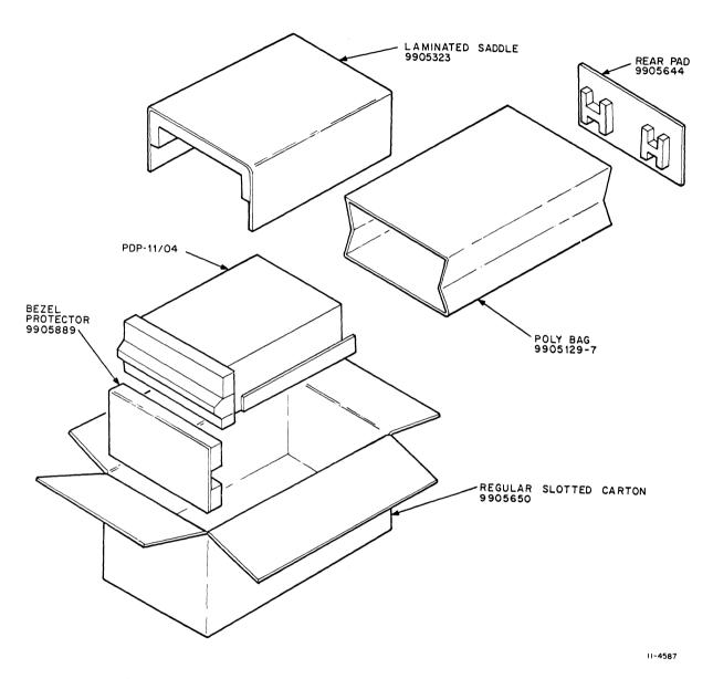
Figure 5-3 Packaging of PDP-11/34 [26.3 cm (10-1/2 inch Box)]
