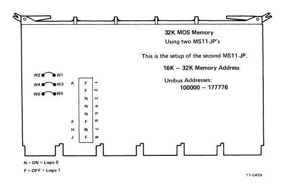
Figure 5-9 Typical Jumper Placement and Switch Settings of Modules (Sheet 6 of 9)
