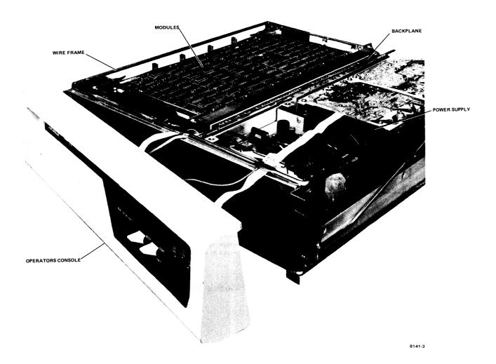
Figure 5-6 Computer Subassemblies of BA11-L Mounting Box
