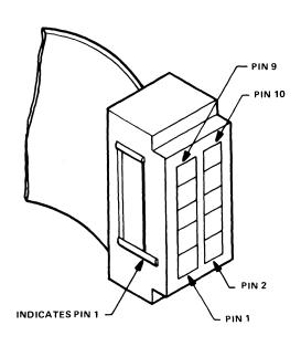
Figure 4-3 3M Connector Pin Locations (Viewed from Pin Side)
