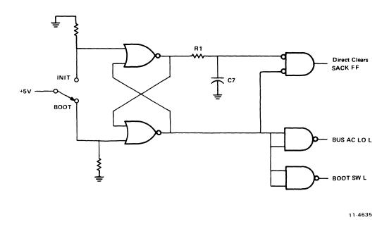
Figure 3-5 BOOT/INIT Switch Logic
