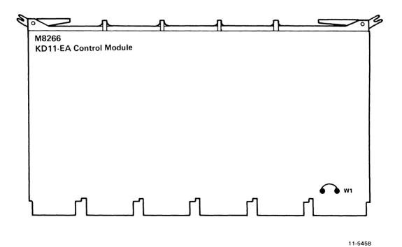
Figure 5-9 Typical Jumper Placement and Switch Settings of Modules (Sheet 3 of 9)
