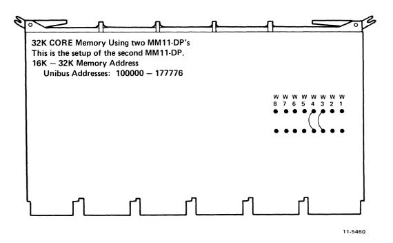
Figure 5-9 Typical Jumper Placement and Switch Settings of Modules (Sheet 8 of 9)
