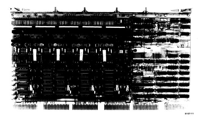
Figure 1-9 MM11-CP Core Memory Module
