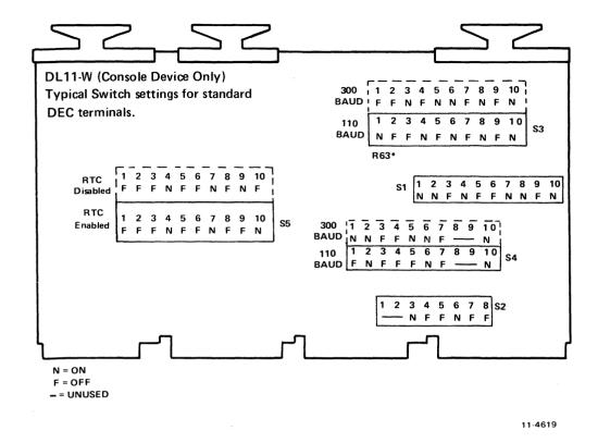
Figure 5-9 Typical Jumper Placement and Switch Settings of Modules (Sheet 9 of 9)
