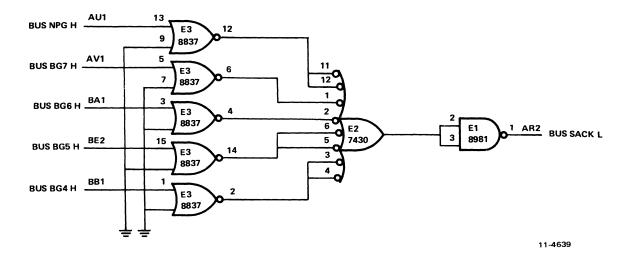
Figure 3-3 M9302 Sack Turnaround Logic
