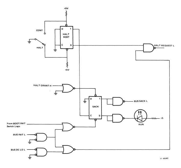
Figure 3-4 HALT/CONT Switch Logic
