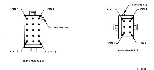
Figure 4-2 Mate-N-Lok Connector Pin Locations (Viewed from Wire Side)
