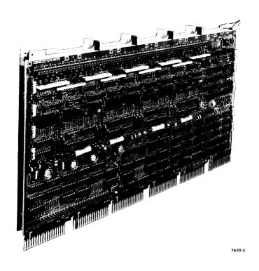
Figure 1-10 MM11-DP Core Memory Module
