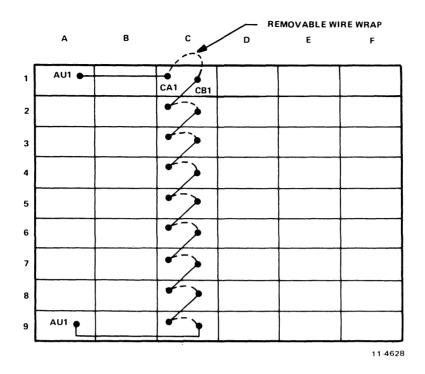
Figure 4-6 NPG Signal Path
