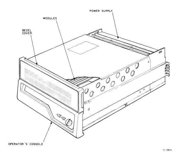
Figure 5-7 Computer Subassemblies of BA11-K Mounting Box
