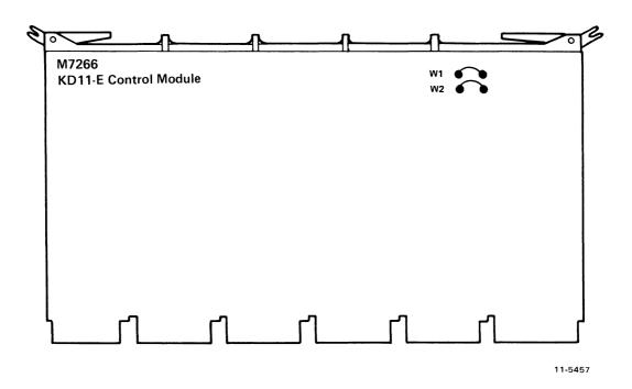
Figure 5-9 Typical Jumper Placement and Switch Settings of Modules (Sheet 2 of 9)
