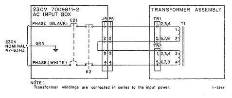
Figure 3-4 230 V Power Configuration
