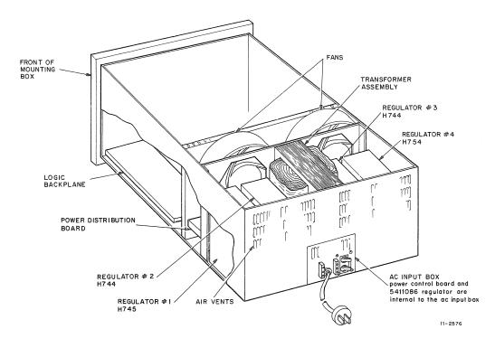
Figure 1-3 Physical Layout of H765 Power Supply
