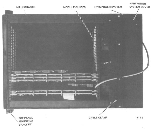
Top View - Main Chassis Cover Removed
