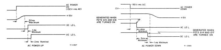
Figure 3-8 5411086 Power Up and Power Down
