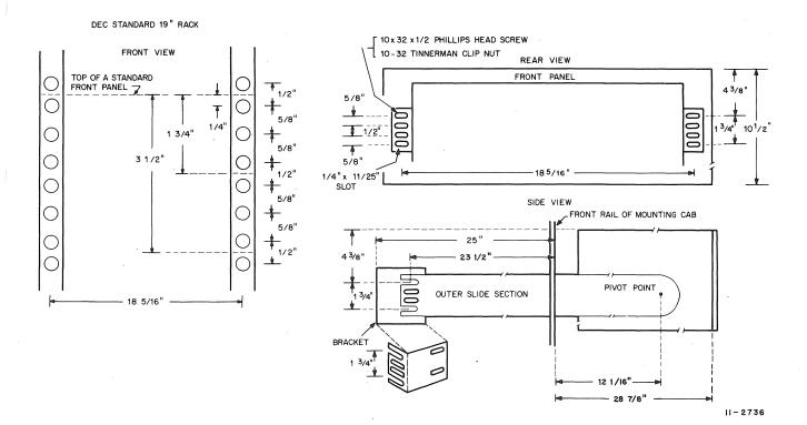
Figure 2-8 Chassis-Trak Slide Mounting Specification
