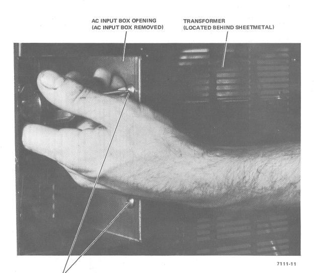
V TRANSFORMER ASSEMBLY MOUNTING SCREWS
