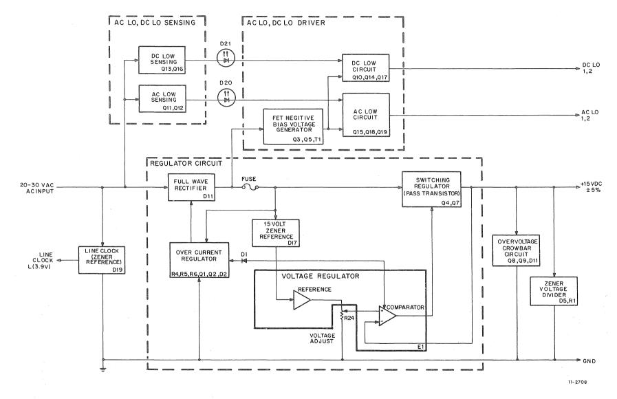
Figure 3-6 5411086 Block Diagram
