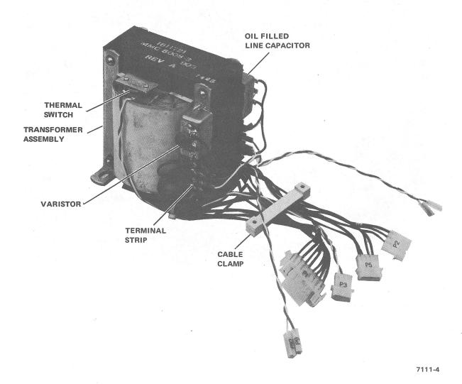
Figure 4-8 Transformer Assembly
