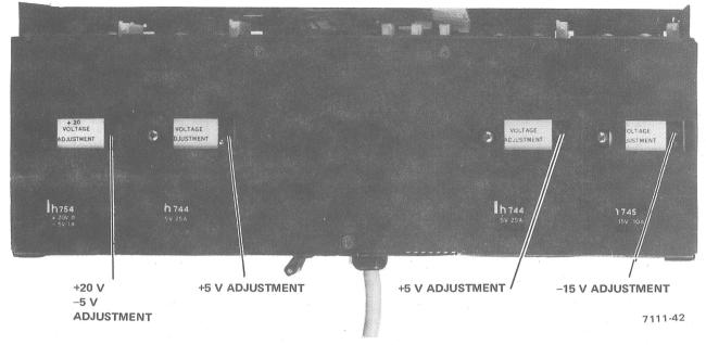
Figure 4-2 Regulator Adjustments
