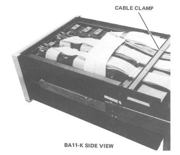
Figure 2-5 Cable Routing
