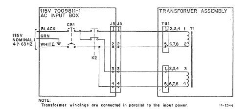
Figure 3-3 115 V Power Configuration
