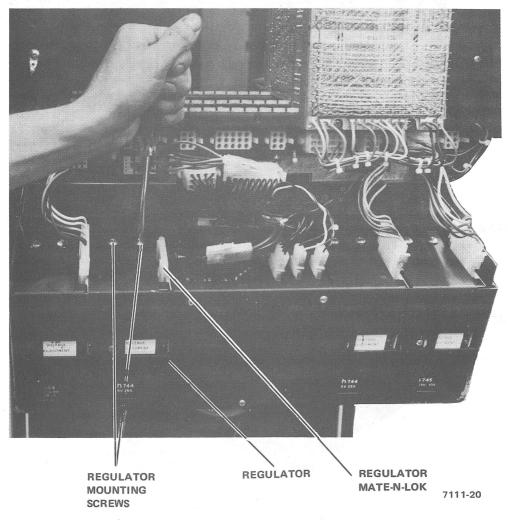
Figure 4-5 Regulator Removal
