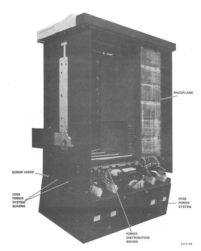
Figure 4-4 H765 Power System Access (Maintenance Position)
