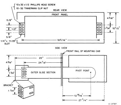
Figure 2-7 Accuride Slide Mounting Specification
