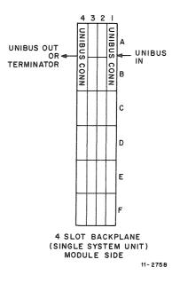
Figure 2-1 Standard Unibus Connection
