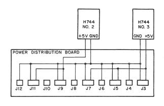
NOTE: Regulators H745, H754, and 5411086 output voltages are common to MATE-N-LOKS J3, J5, J7, J9, and J11. 11-2565
