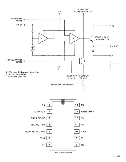
Figure 3-9 Voltage Regulator E1, Simplified Diagram
