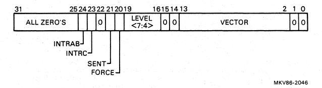
Figure A-12 Error Interrupt Control Register
