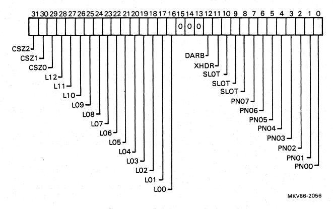
Figure A-22 Port Parameter Register
