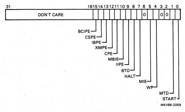
Figure A-25 Port Maintenance Control/Status Register
