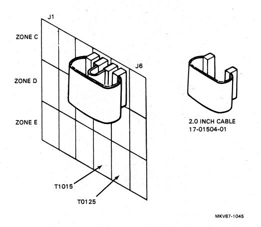
Figure 2-5, VAXBI Backplane - CIBCA Intermodule Cable Connections
