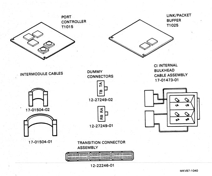
Figure 1-3 Hardware Components of the CIBCA
