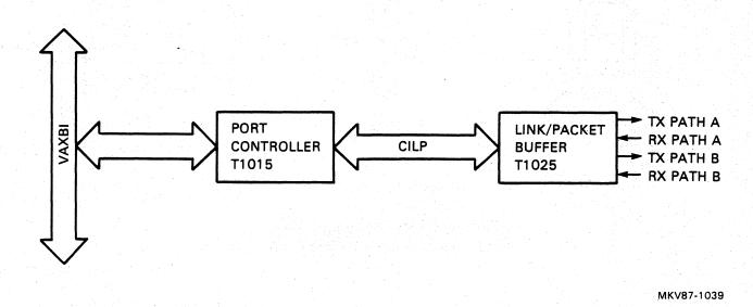
Figure 1-2 Simplified CIBCA Block Diagram
