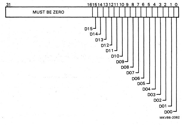
Figure A-28 Maintenance Data Register
