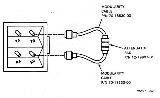
Figure 3-2 Diagnostic Loopback Cable Connections
