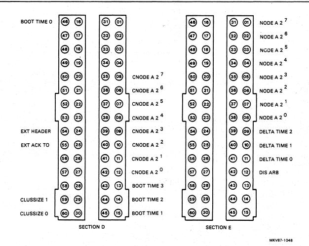
Figure 2-8 CIBCA Backplane Jumper Pinning
