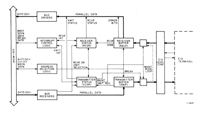
Figure 1-3 DL11-W Terminal Control
