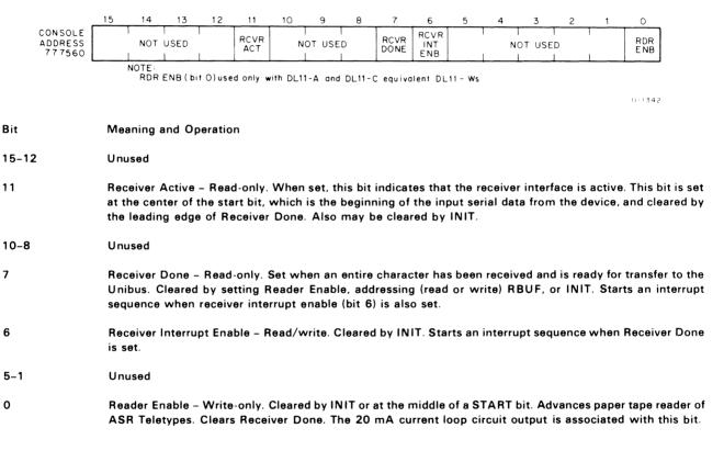
Figure 3-1 Receiver Status Register Bit Format
