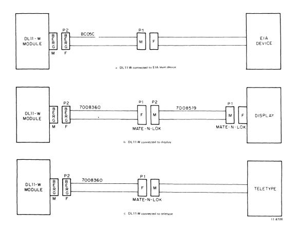
Figure 2-5 DL11-W Cable Connections
