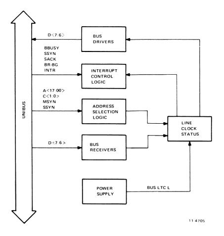
Figure 1-4 Line Clock Block Diagram
