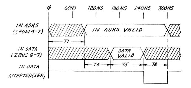
Figure 4-21 Typical Input Bus Timing
