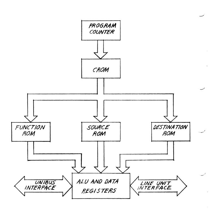
Figure 1-3 Microprocessor Simplified Block Diagram
