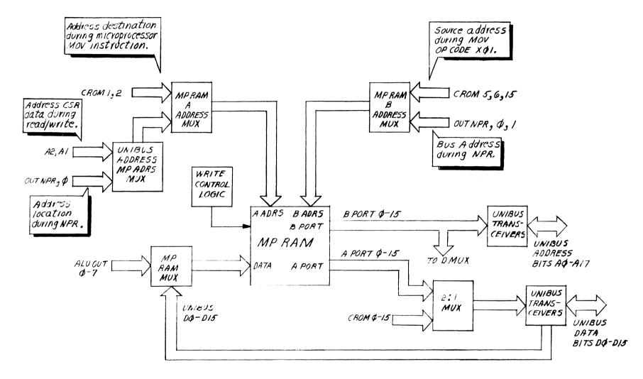
Figure 4-14 Block Diagram of Multiport RAM and Associated Logic
