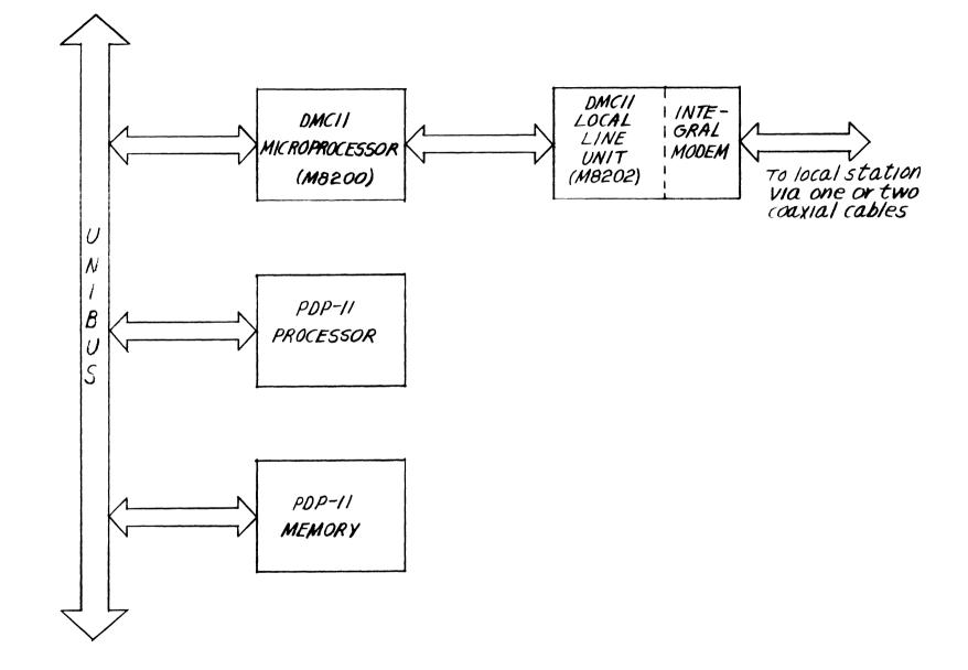
Figure 1-2 DMC11 Local Line Unit Interface
