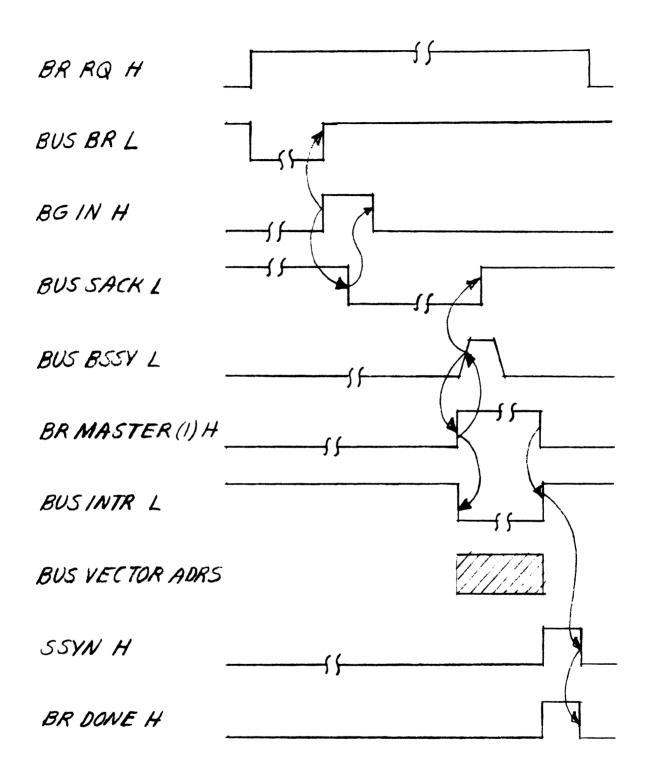
Figure 4-19 Interrupt Timing Diagram
