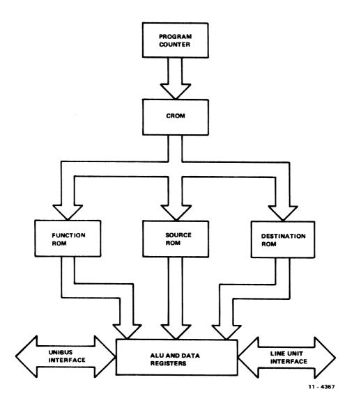
Figure 1-3 Microprocessor Simplified Block Diagram
