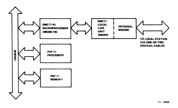
Figure 1-2 DMC11 Local Line Unit Interface
