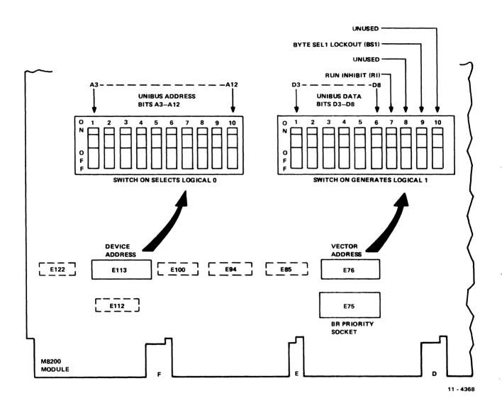
Figure 2-1 Microprocessor Device and Vector Address Switches
