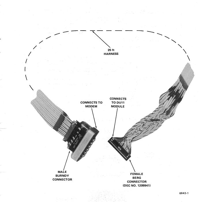
Figure 2-7 BC01W-25 Cable Harness Used to Connect DU11-EA to Bell 303 Modem
