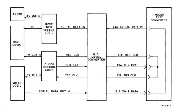
Figure 4-11 External Loop Maintenance Mode Interconnection Diagram
