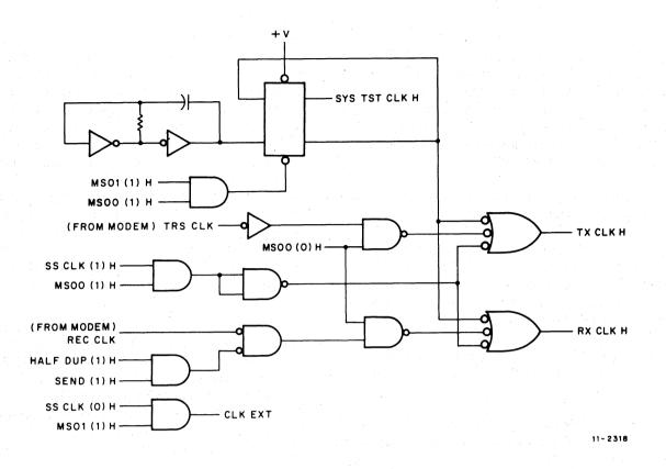
Figure 4-12 Clock Control Logic
