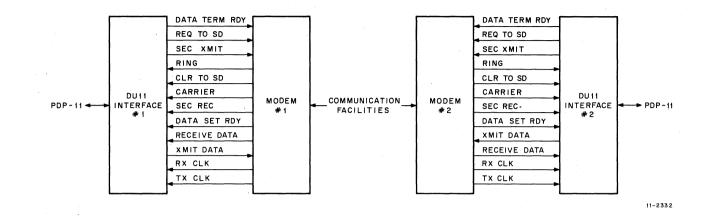
Figure 4-1 DU11 to Modem Interface Diagram
