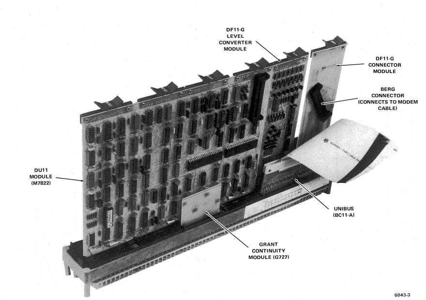
Figure 2-4 Current Mode Configuration (DU11-EA) Using DD11-B Mounting Panel
