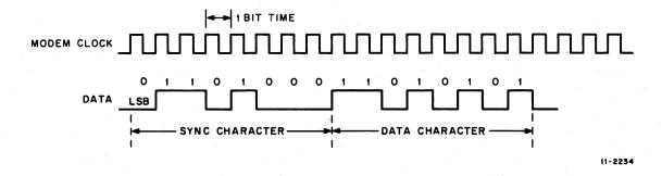
Figure 1-2 Synchronous Format
