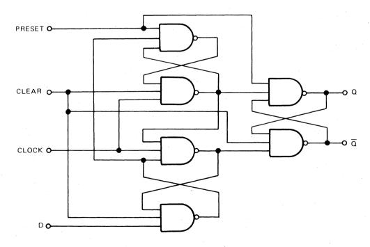
Figure C-7 74H74 Logic Diagram
