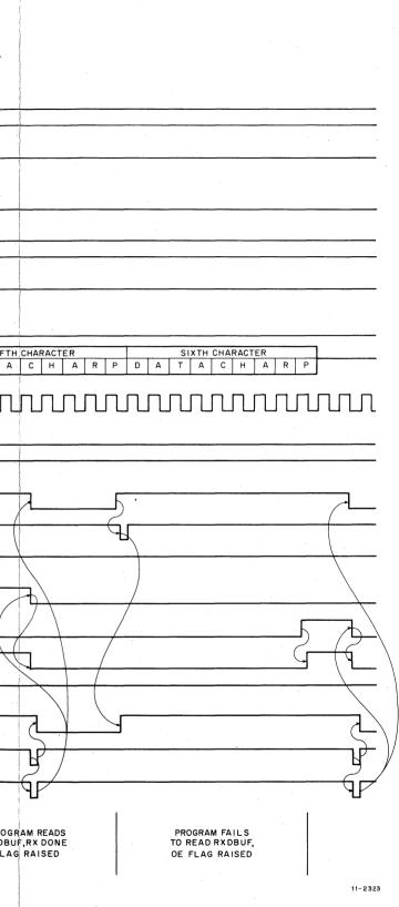
Figure 4-15 RCVR Internal Synchronous Mode Timing Diagram (Example II)
