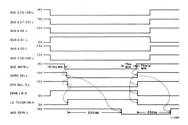
Figure 4-7 DATOB Timing Diagram
