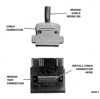
Figure 2-9 Modem Test Connection Installation
