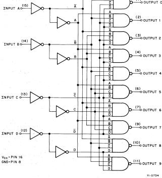
Figure C-1 7442 Package and Logic Diagrams
