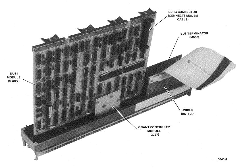
Figure 2-1 Standard Configuration (DU11-DA) Using DD11-B Mounting Panel
