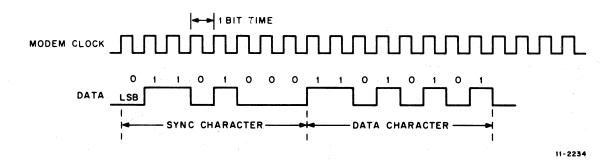
Figure 1-2 Synchronous Format
