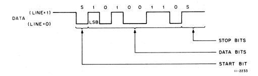
Figure 1-1 Asynchronous Technique Format
