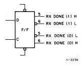
Figure 1-5 Flip-Flop Signal Names
