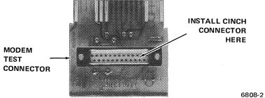
Figure 2-9 Modem Test Connection Installation
