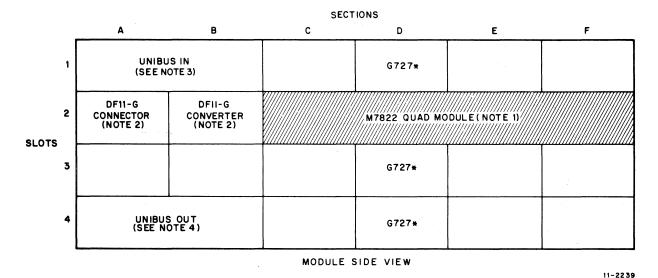
\*Grant Continuity Module (G727) must be installed in each slot that does not receive an interface logic module.
