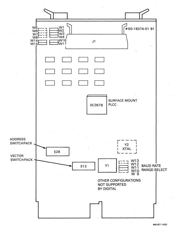
Figure 2-2 Jumper Locations (DC367B Surface Mount)
