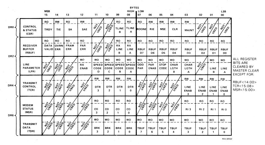
Figure 3-1 Register Bit Assignment
