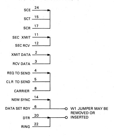
Figure 1-5 Loopback Connection
