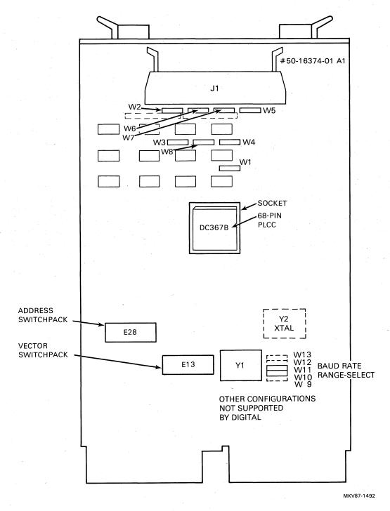
Figure 2-1 Jumper Locations (DC367B Socket Mount)
