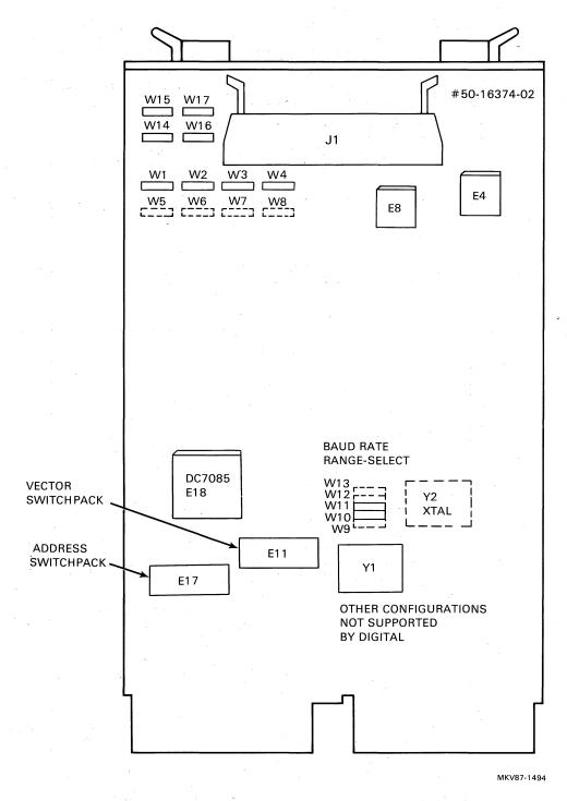
Figure 2-3 Jumper Locations (DC7085 Surface Mount)
