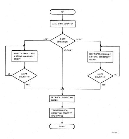
Figure 3-3 KE11-E ASH Algorithm
