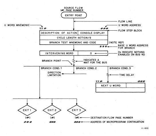
Figure 4-7 Flow Diagram Conventions
