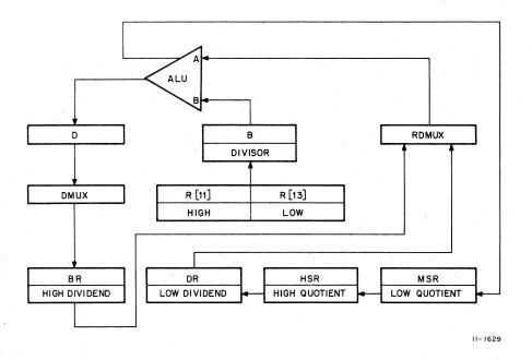
Figure 4-13 FDIV Flow Block Diagram
