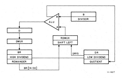
Figure 4-10 DIV Flow Block Diagram
