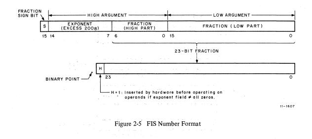
The KE11-F Option stores the exponent in excess  $200_8$  ( $128_{10}$ ) notation. As a result, exponent values from -128 to +127 are represented by the binary equivalent of 0 to 255 (octal 0-377). Mantissas are represented in sign magnitude form.
