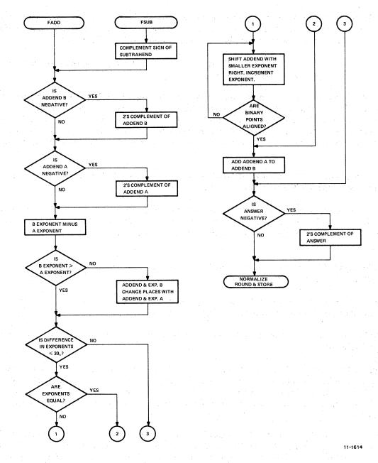
Figure 3-7 KE11-F FADD and FSUB Algorithm
