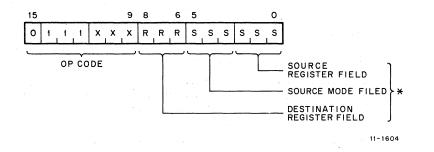
\*Note that for the EIS instructions the Source Register is considered the Destination since the answer is stored in that register. The Destination Mode and Register Field are considered to be the source. This is not consistent with other PDP-11 family instruction formats but is used throughout the discussions of the EIS instructions in this manual.
