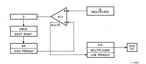
Figure 4-9 MUL Flow, Block Diagram
