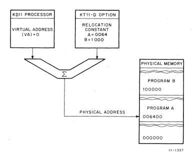
Figure 3-1 Simplified Memory Relocation Example
