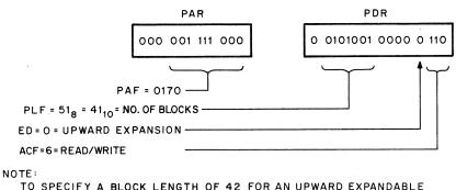
TO SPECIFY A BLOCK LENGTH OF 42 FOR AN UPWARD EXPANDABLE PAGE, WRITE HIGHEST AUTHORIZED BLOCK NO. DIRECTLY INTO HIGH BYTE OF PDR. BIT 15 IS NOT USED BECAUSE THE HIGHEST ALLOWABLE BLOCK NUMBER IS 1778
