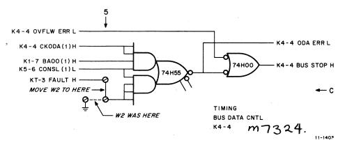
Figure 2-4 KD11-A Wiring Change No. 4
