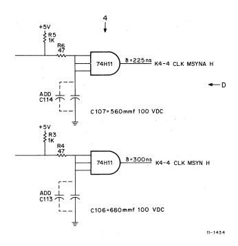
Figure 2-6 KD11-A Wiring Changes No. 6 and No. 7
