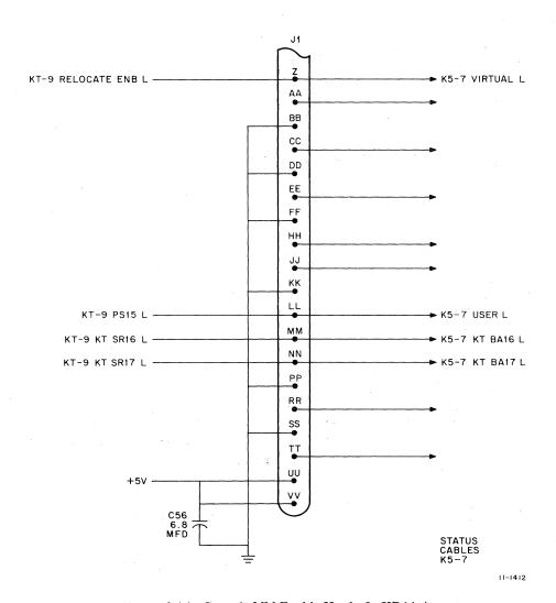
Figure 2-14 Console MM Enable Hooks In KD11-A
