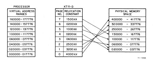
Figure 3-2 Relocation of a 32K Word Program Into 124K Word Physical Memory
