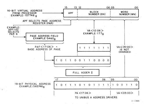
Figure 3-3 Construction of an 18-Bit Physical Address
