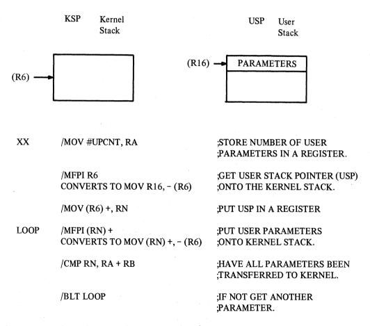
The monitor can now initiate the required command to the I/O. Although all devices have the capability of accessing all of physical core (meaning the ability to access user core), this practice usually is not preferred because the user is subject to being "swapped out" at any time. Therefore, data is normally placed into a monitor (Kernel) buffer. The monitor must then transfer that data to user core by means of the MTPI instruction.
