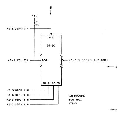
Figure 2-7 KT-3 Fault H Hook In KD11-A
