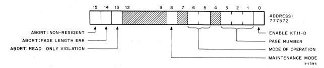
Figure 3-9 Format of Status Register 0 (SR0)
