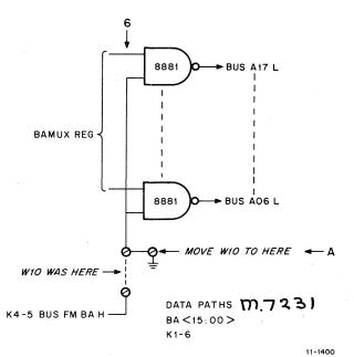
Figure 2-1 KD11-A Wiring Change No. 1
