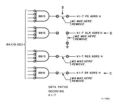
Figure 2-3 KD11-A Wiring Change No. 3 7231
