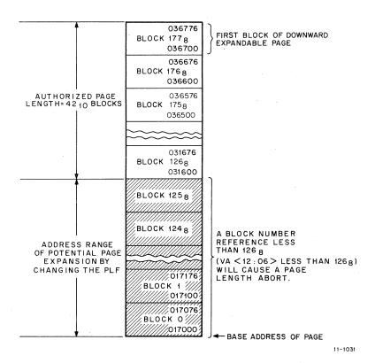
Figure 3-8 Example of a Downward Expandable Page
