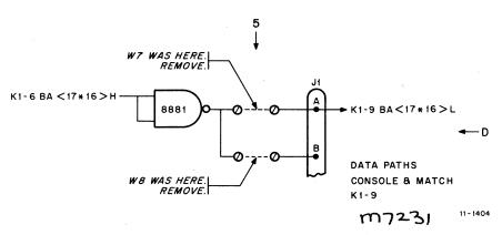
Figure 2-5 KD11-A Wiring Change No. 5
