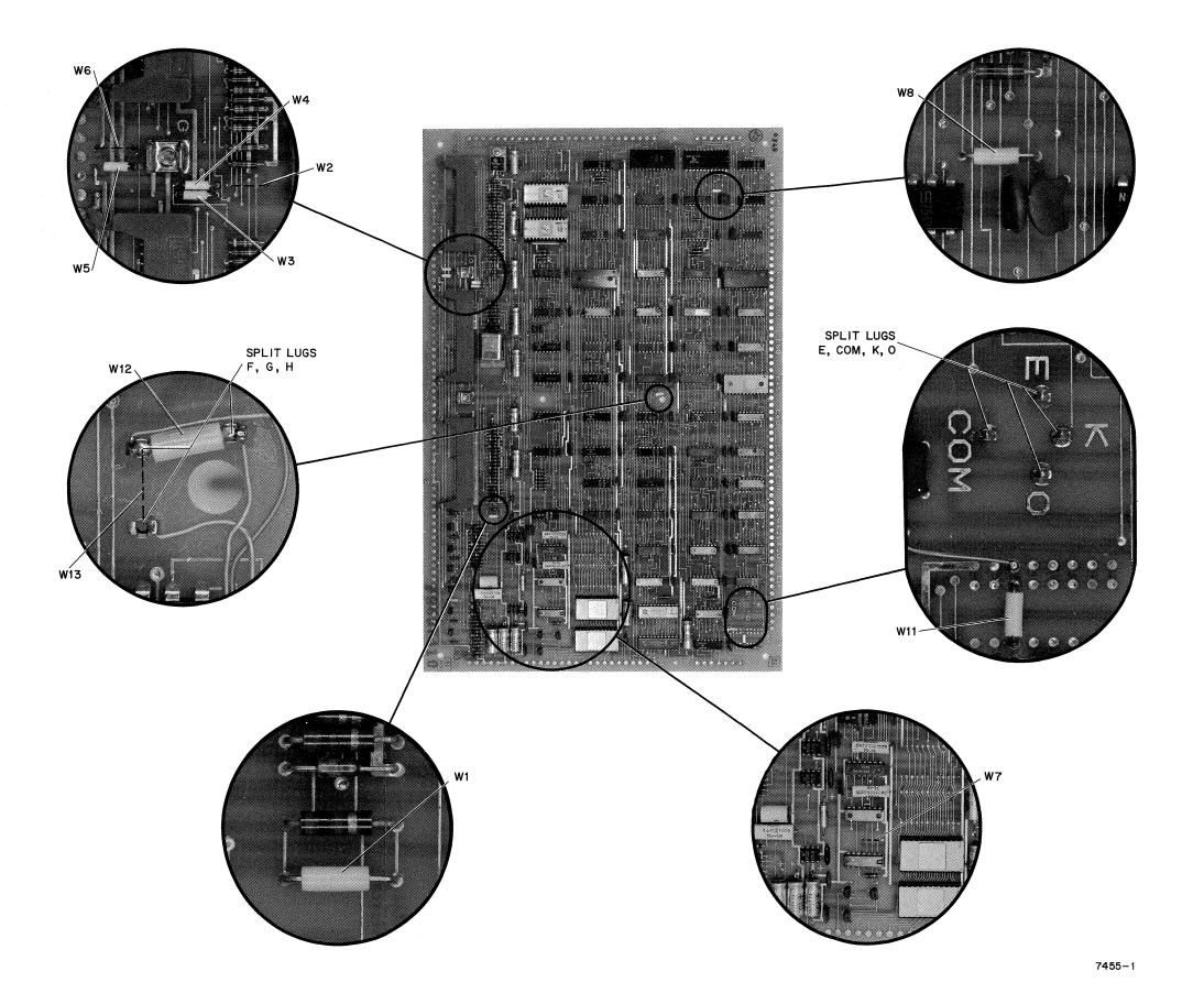
Figure 8 Logic Board Jumper Locations
