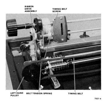
Figure 23 Belt Tension Spring Location
