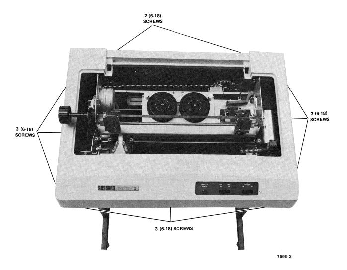
Figure 19 Printer Housing Removal
