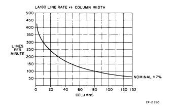
Figure 9 LA180 Line Rate Versus Column Width
