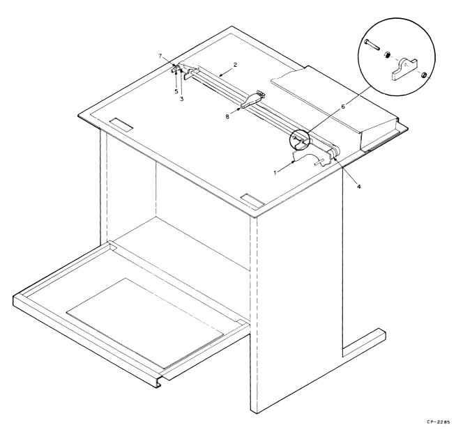
Figure 21 Installation of Compressed Font Option Kit (LAXX-KJ)
