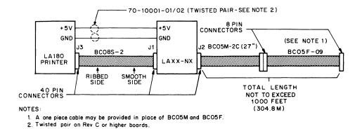
Figure 17 Current Loop LAXX-NX Cabling
