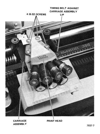
Figure 20 Print Head Removal
