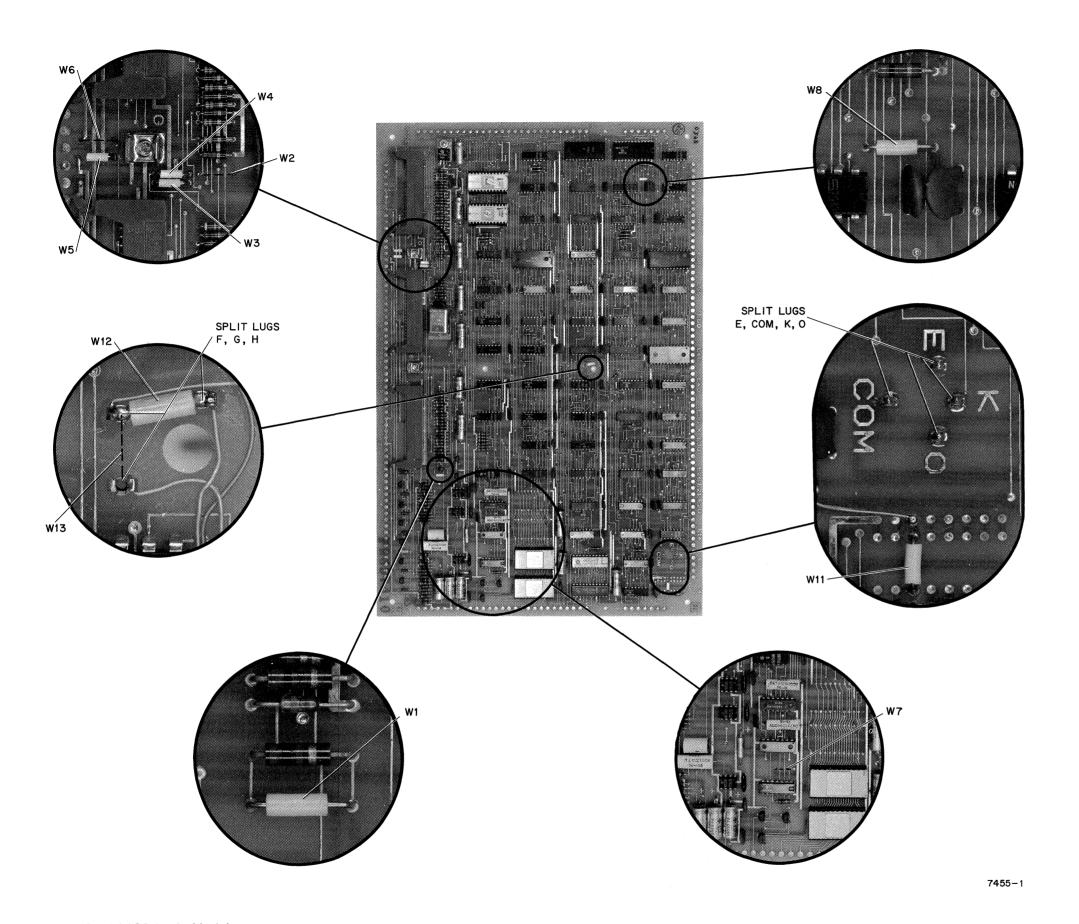
Figure 18 LA180 Logic Module Jumper Locations
