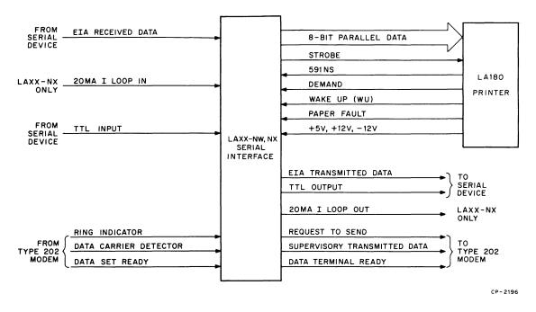
Figure 12 Serial Interface/LA180 Simplified Interface Diagram
