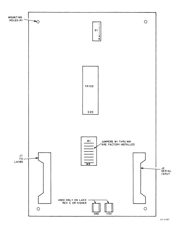
Figure 14 Serial Interface Component Location
