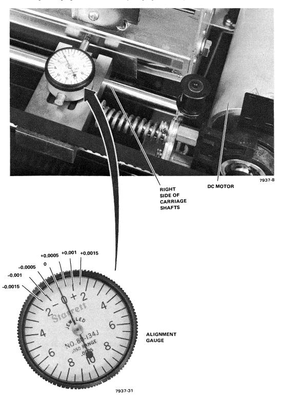
Figure 22 Alignment Gauge Positioning
