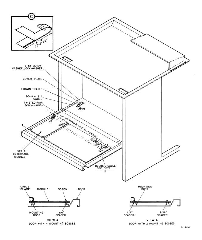
Figure 13 Module Installation on LA180 Rear Door
