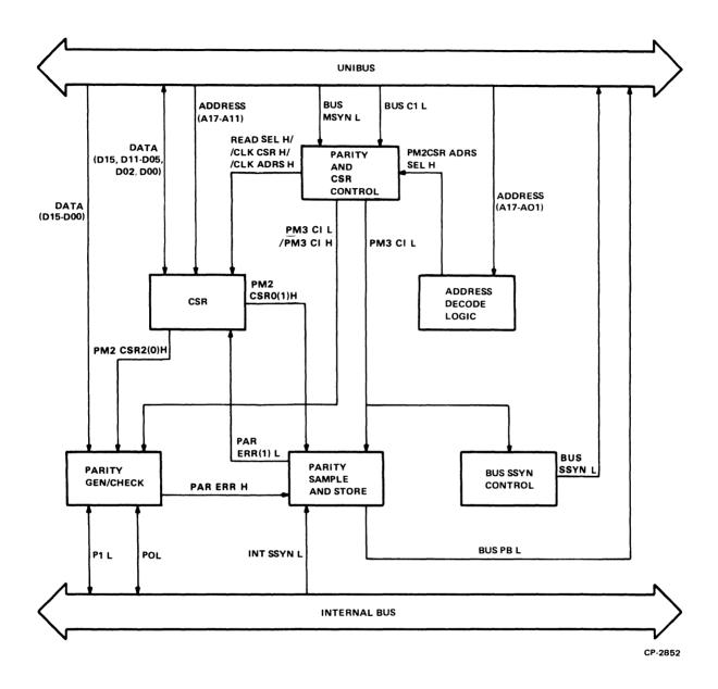
Figure 2-3 M7850 Block Diagram
