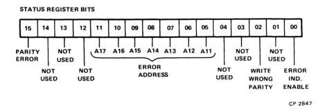
Figure 2-7 Control and Status Register Bit Allocation
