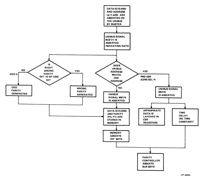
Figure 2-4 DATO Flow Diagram
