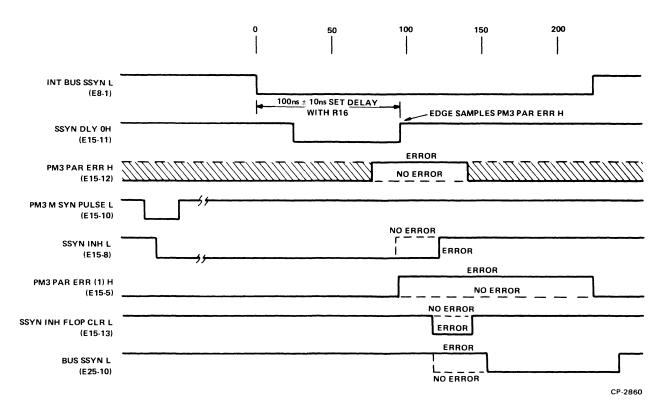
Figure 3-5 Timing Diagram of BUS SSYN Control
