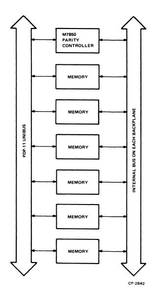
Figure 1-2 Unibus/Internal Bus Simplified Block Diagram
