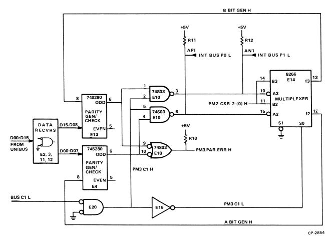
Figure 3-2 Parity Generation and Check Circuit
