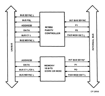
Figure 2-1 Unibus/Internal Bus Connections
