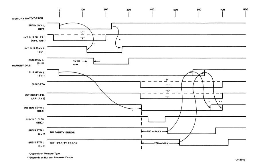
Figure 4-4 Typical Timing Waveforms When Addressing Memory
