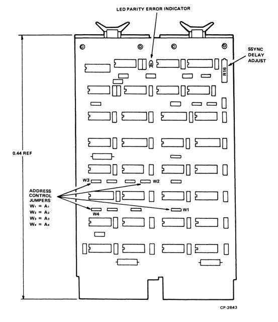
Figure 1-3 Physical Layout of M7850
