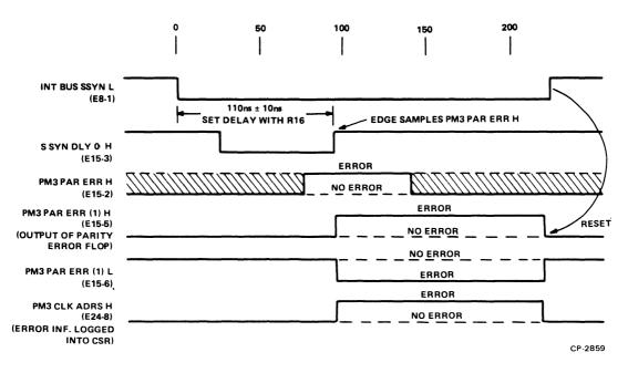
Figure 3-4 Timing Diagram of CSR Error Logging
