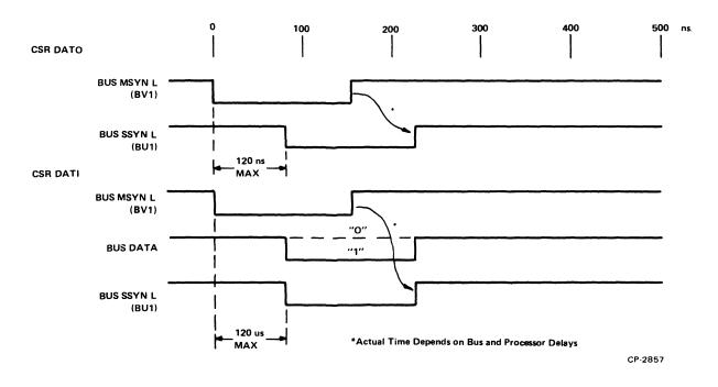
Figure 4-3 Typical Timing Waveforms When Addressing CSR
