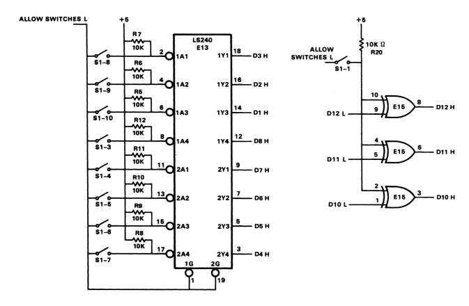
OFFSET SWITCHES AND CORRESPONDING BUS ADDRESS BITS
