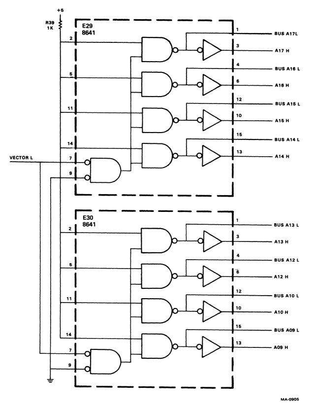
Figure 2-5 Address Generation Logic
