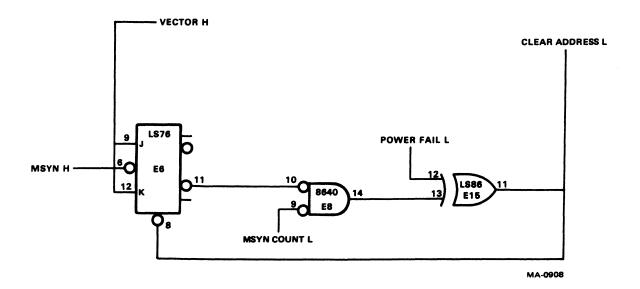
Figure 2-8 Power-Up Transfer Detection Logic
