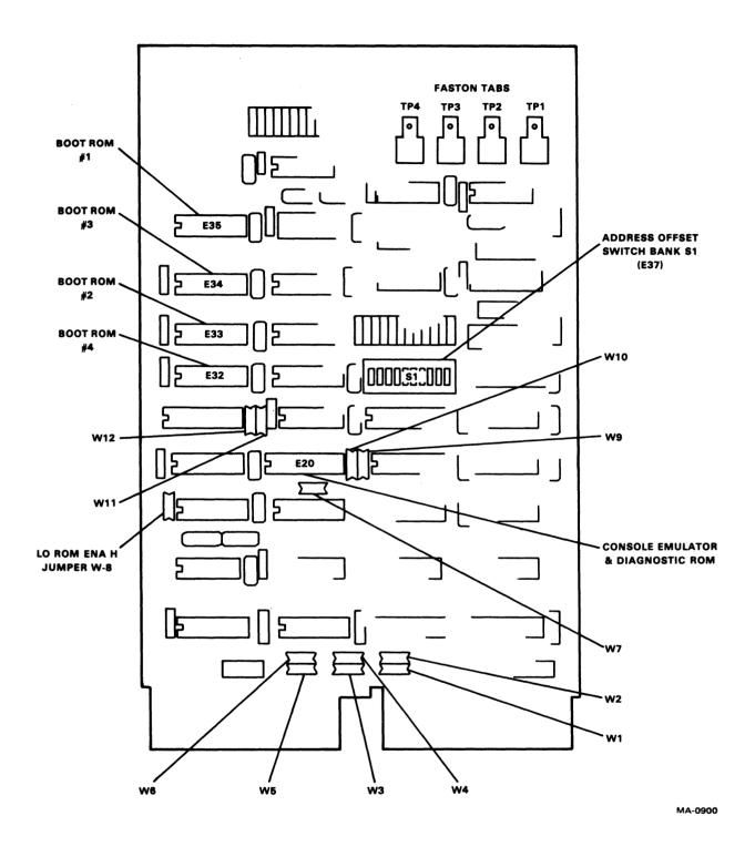
Figure 1-1 M9312 Bootstrap/Terminator Module
