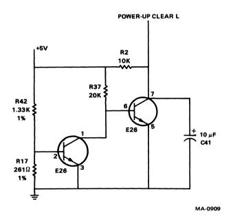
Figure 2-9 Power-Up Clear Circuitry
