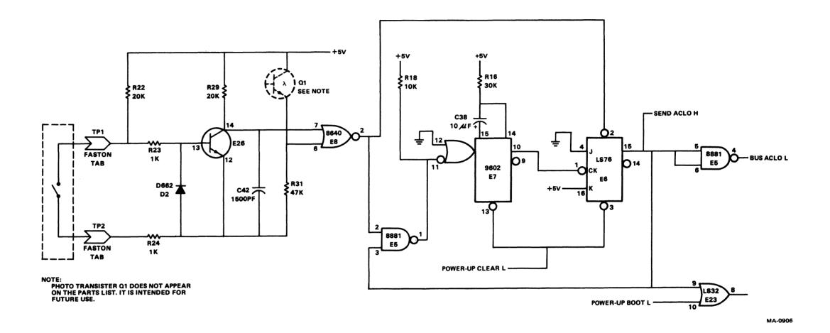
Figure 2-6 External Boot Logic
