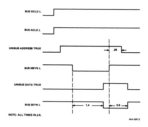
Figure 1-2 M9312 Timing Constraints
