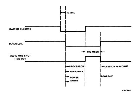
Figure 2-7 External Boot Timing
