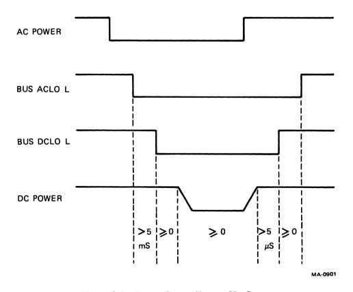
Figure 2-3 Power-Down/Power-Up Sequence
