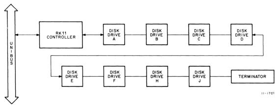
Figure 1-1 RK11-D and RK11-E Disk Drive System
