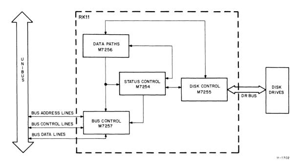
Figure 1-2 RK11 Controller, Functional Block Diagram
