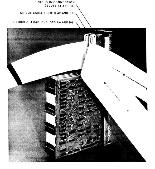
Figure 2-1 RK11 Cable Connections
