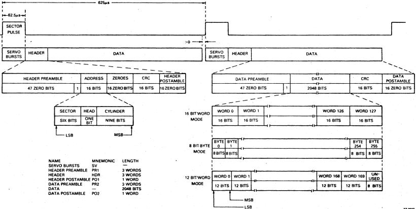
Figure 2-2 RLØ1K/RLØ2K Disk Cartridge Characteristics
