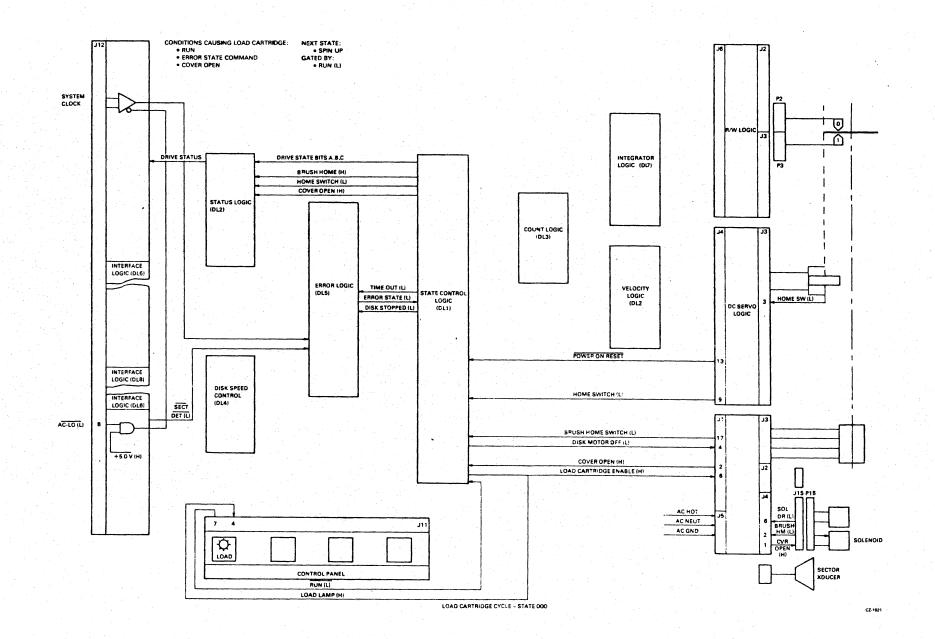
Figure 4-2 Device Startup - Load Cartridge Cycle
