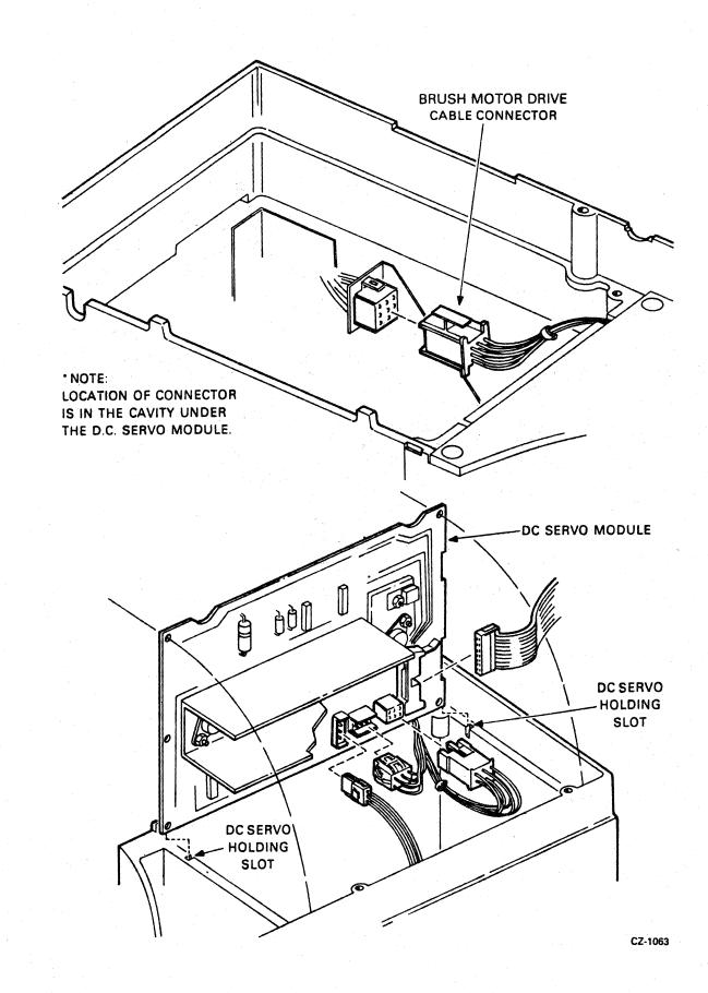
Figure 2-9 DC Servo Module
