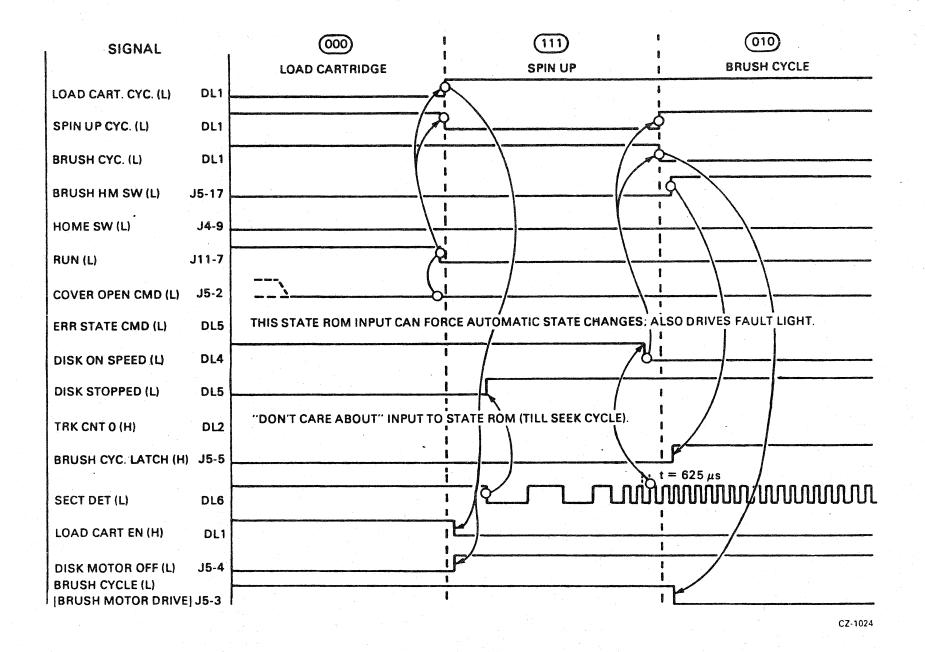
Figure 4-5 Device Startup - Spin-up Cycle Timing
