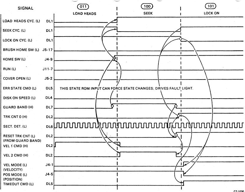
Figure 4-11 Device Start-up - Seek Timing
