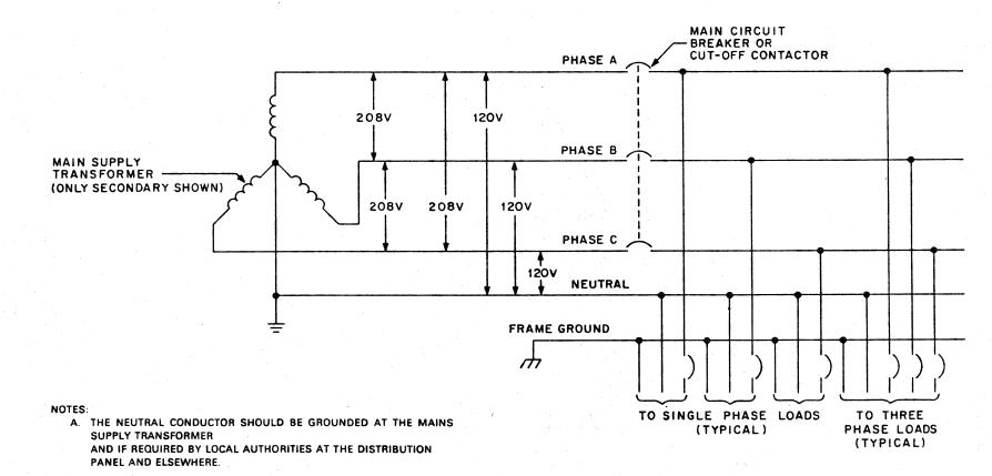
B. THE FRAME GROUND CONDUCTOR MAY CONSIST OF ELECTRICAL METALLIC CONDUIT OR RACEWAY IF APPROVED BY LOCAL AUTHORITIES.
