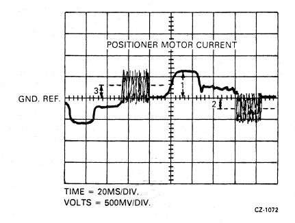
Figure 3-13 Positioner Motor Current Check
