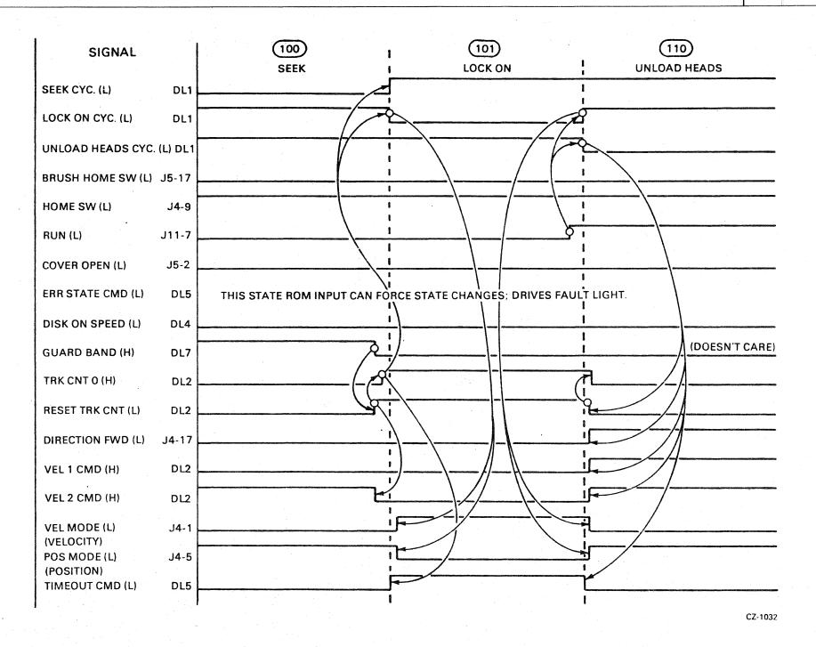
Figure 4-13 Device Startup - Lock on Track Ø Timing
