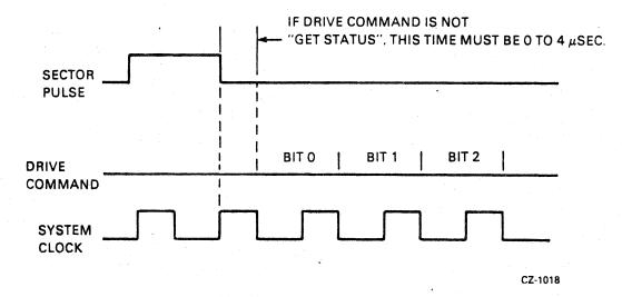
Figure 3-3 Relationship Between System Clock and Drive Command Word Bits
