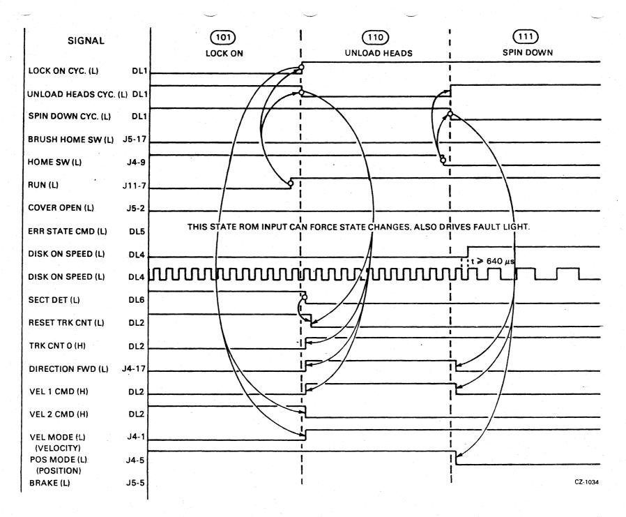
Figure 4-15 Device Startup - Unload Heads Timing
