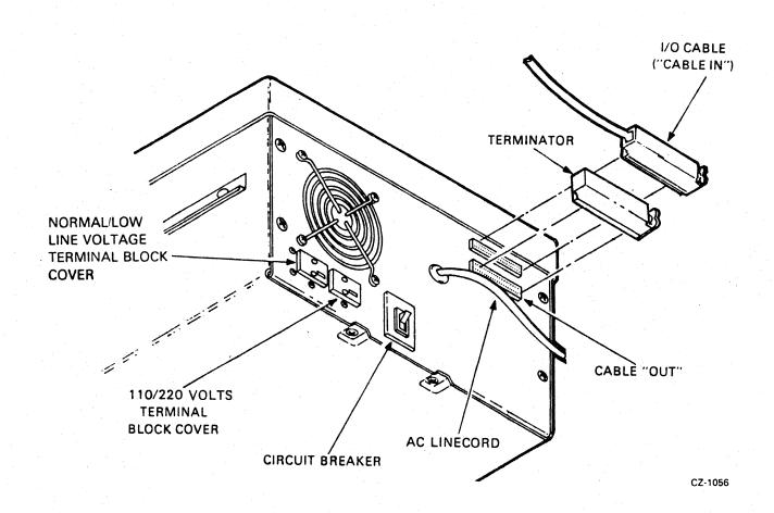
Figure B-22 RLØ1/RLØ2 Disk Drive - Rear View
