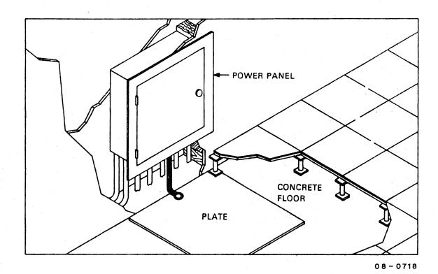
Figure B-4 Power Panel Grounded to Metal Plate
