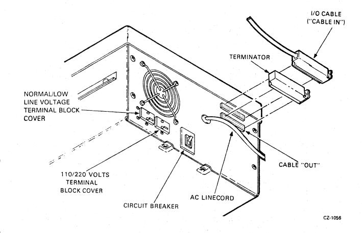
Figure B-1 RLØ1/RLØ2 Disk Drive - Rear View
