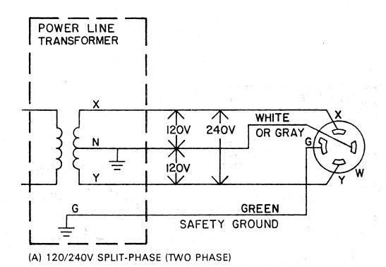
Figure B-7 Split Phase (2-Phases) Power System
