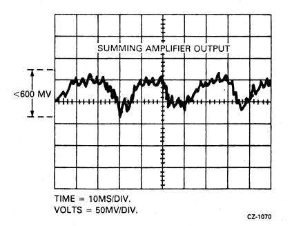
Figure 3-11 Summing Amplifier Output
