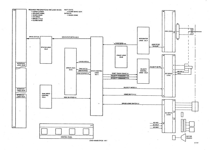
Figure 4-8 Device Start-up - Load Heads Cycle
