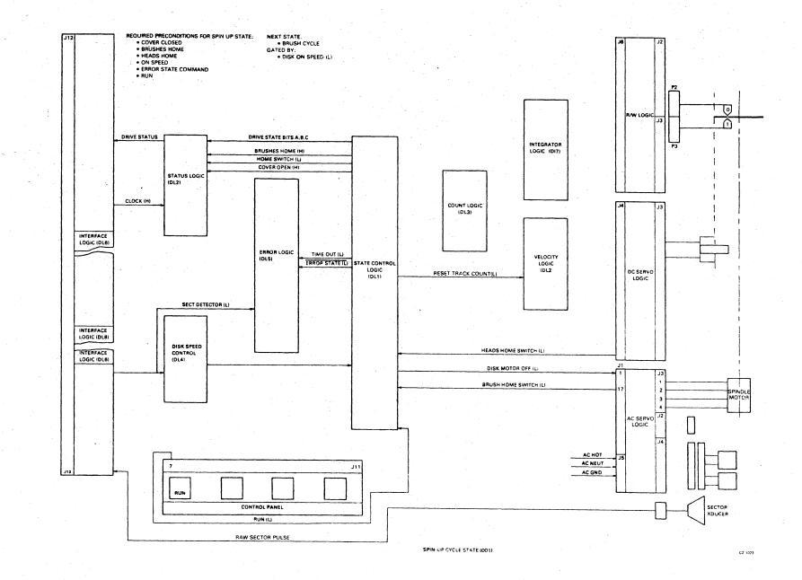
Figure 4-4 Device Startup - Spin-up Cycle
