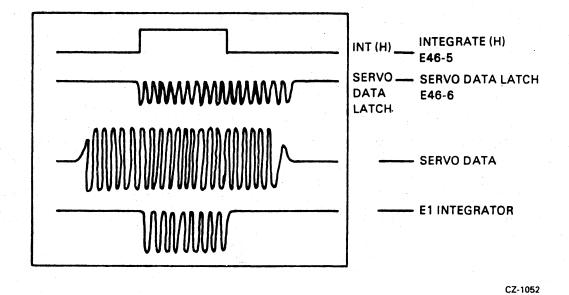
Figure 5-9 Servo Data and Integrate Enable Waveforms
