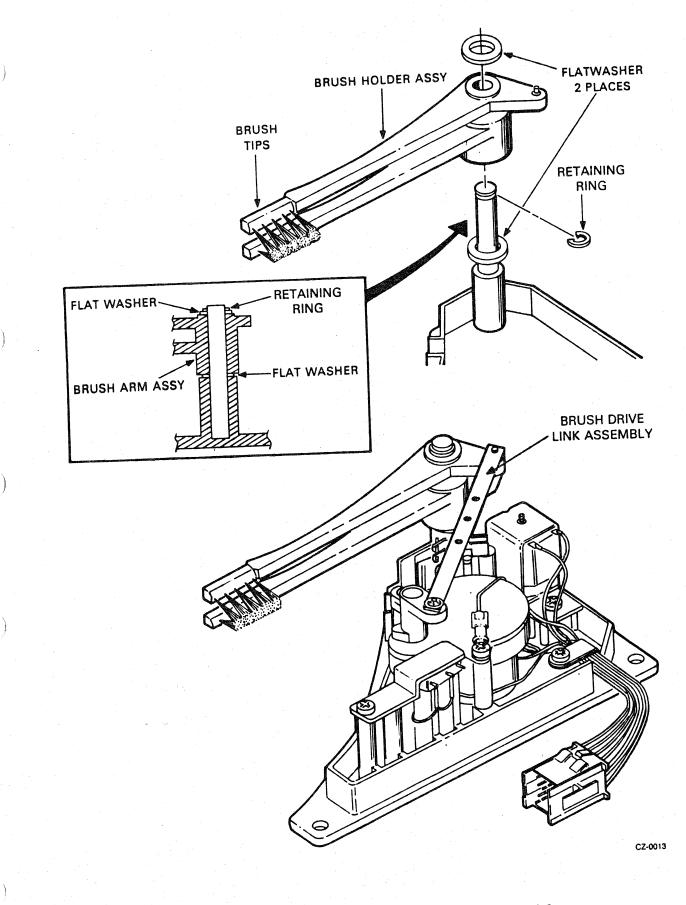
Figure 2-11 Exposed Brush Drive Assembly
