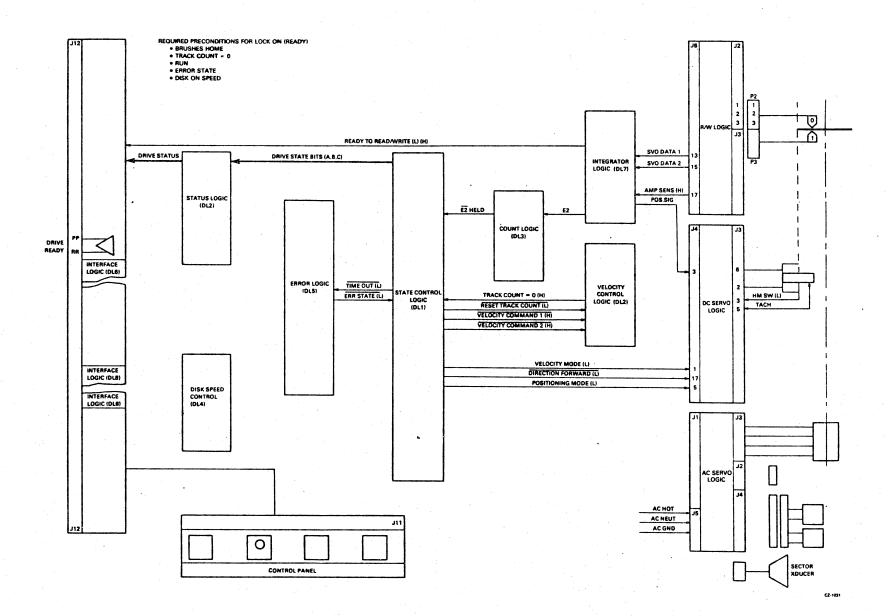
Figure 4-12 Device Startup - Lock on Track Ø
