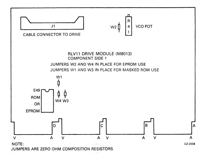
Figure B-16 RLV11 Drive Module (M8013)
