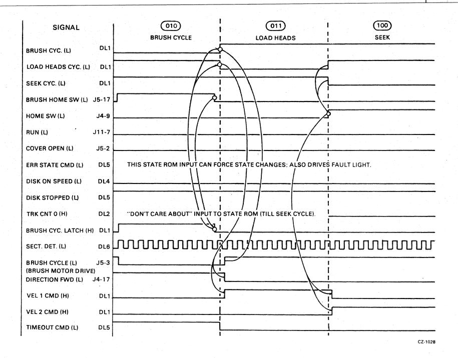
Figure 4-9 Device Start-up - Load Heads Cycle Timing
