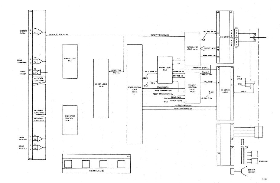
Figure 4-20 Seek Functional Block Diagram
