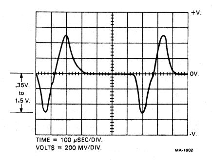
Figure 3-2 Sector Transducer Output
