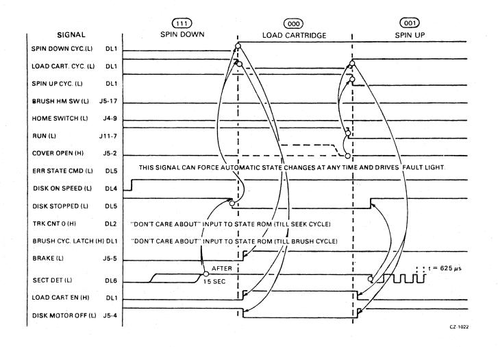
Figure 4-3 Device Startup - Load Cartridge Timing
