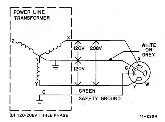
Figure B-8 Three Phase Y Power System
