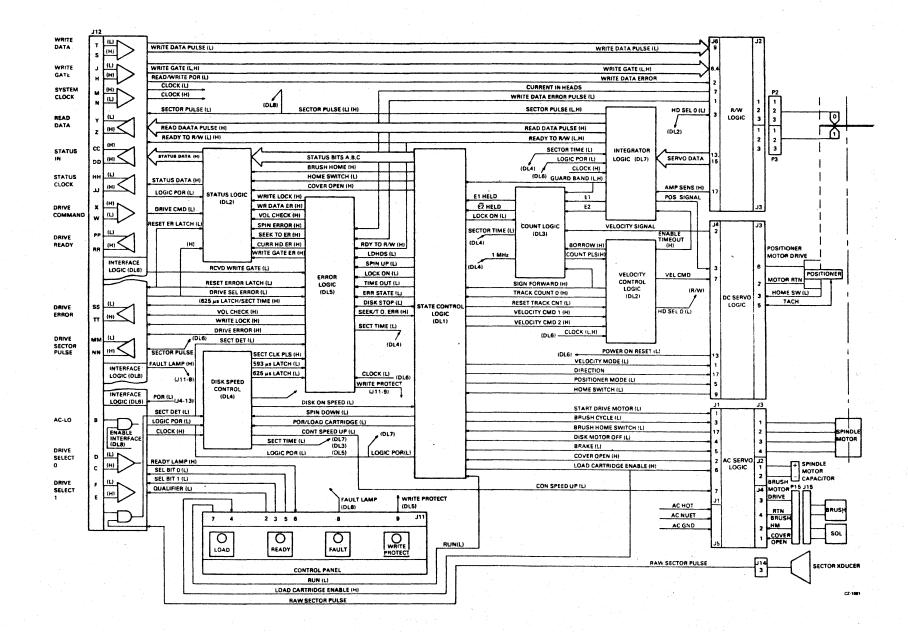
Figure 4-1 Disk Drive Detailed Block Diagram
