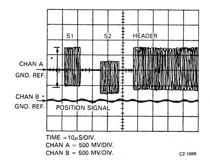
Figure 3-7 Servo Bursts and Position Signal
