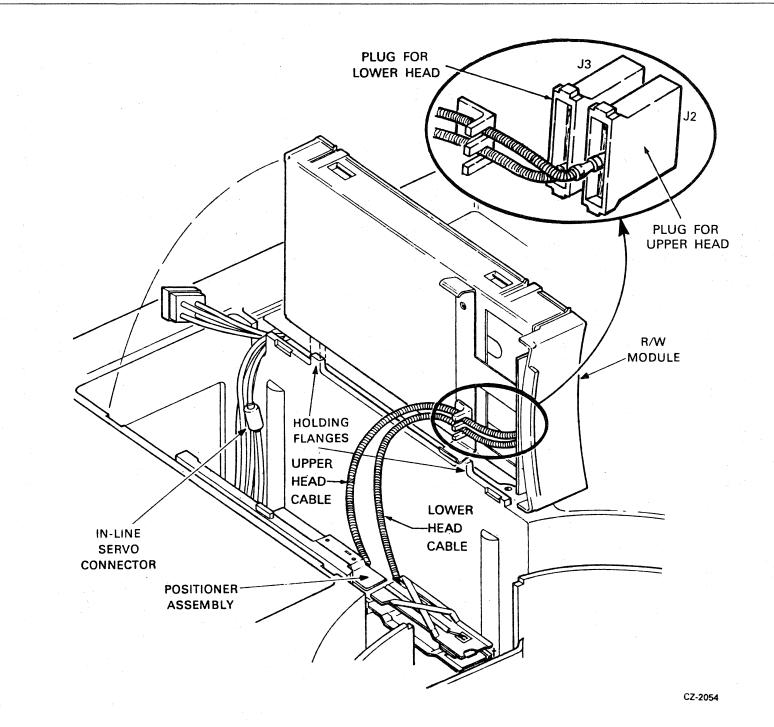
Figure 2-13 Read/Write Module (Upright)
