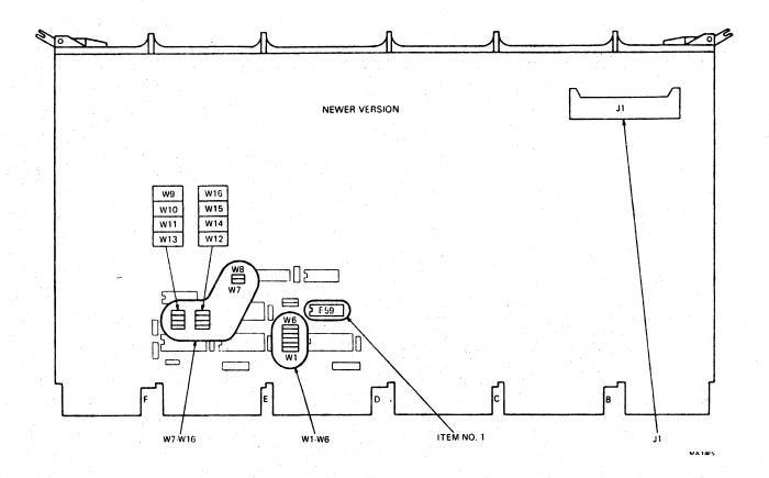
Figure B-9 RL11 Component Layout (Sheet 2 of 2)
