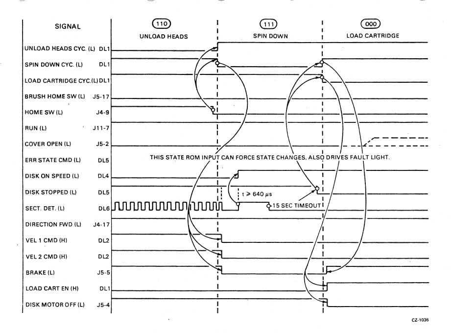
Figure 4-17 Device Startup - Spin Down Timing
