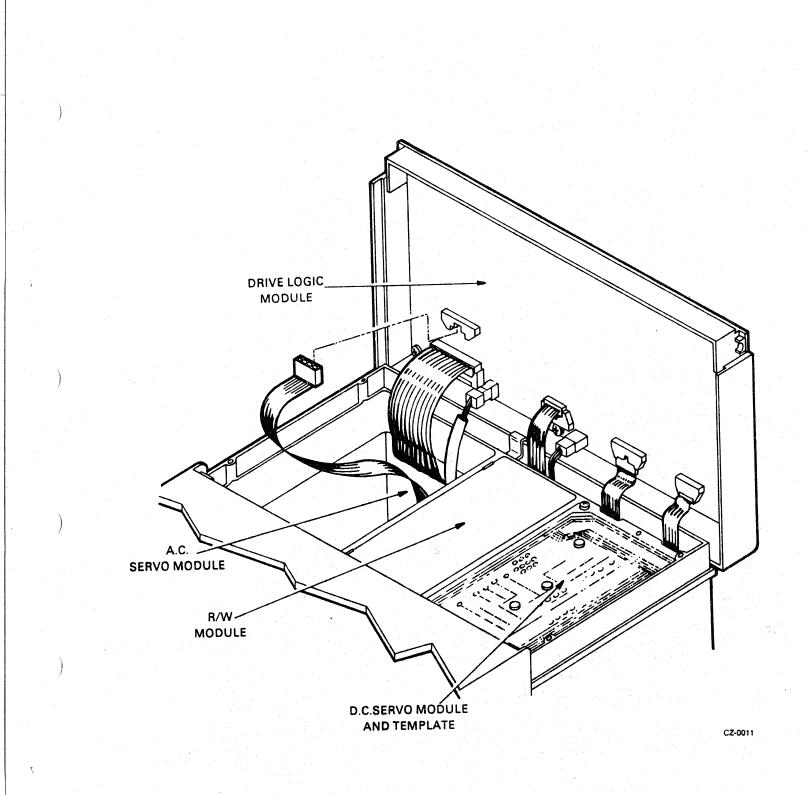
Figure B-24 RLØ1/RLØ2 Disk Drive - Exposed Drive Logic Module
