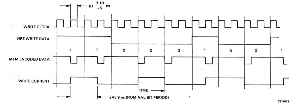
Figure 2-7 Modified Frequency Modulation (MFM) Encoding
