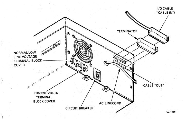
Figure 2-20 Rear View of Drive
