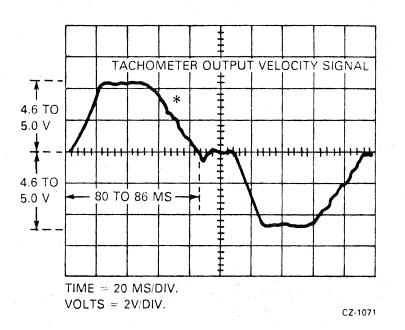
Figure 3-12 Tachometer Output Velocity Signal
