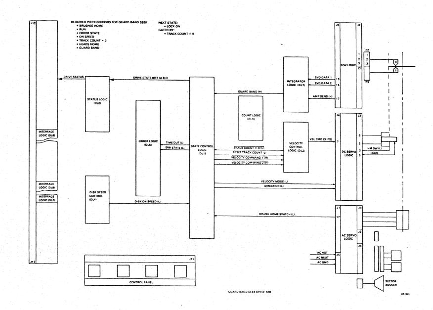
Figure 4-10 Device Start-up - Seek Cycle
