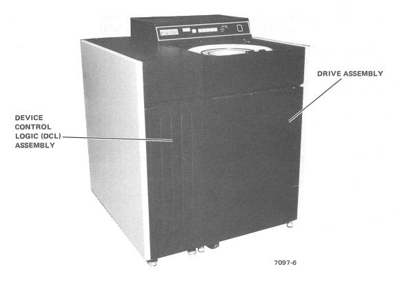
Figure 1-1 RP04 Drive and DCL Assemblies
