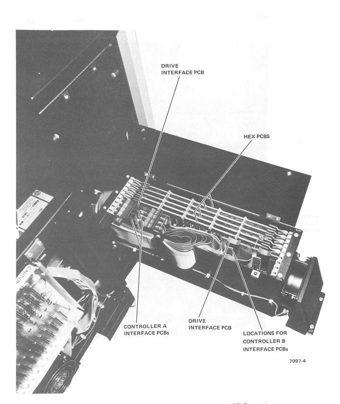
Figure 2-3 Card Nest and Cable Assembly PCB Layout
