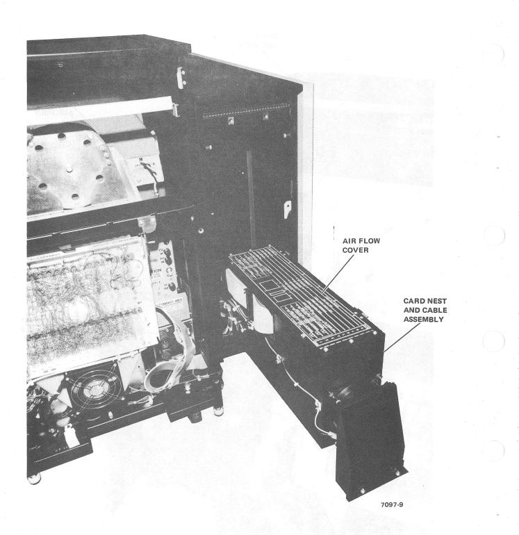
Figure 2-2 DCL Rear View, Card Nest and Cable Assembly Extended
