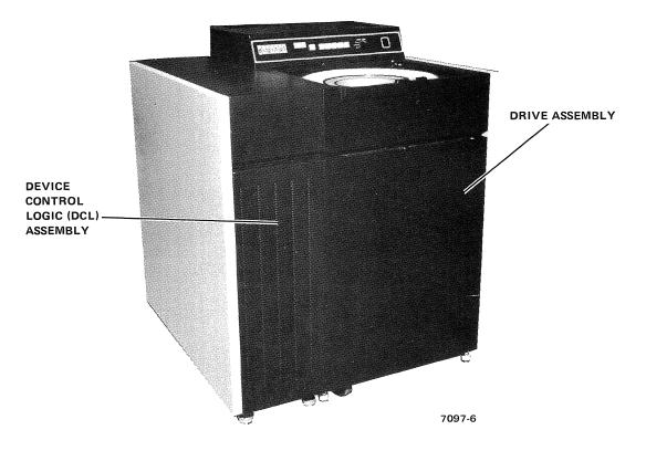
Figure 1-1 RP04 Drive and DCL Assemblies
