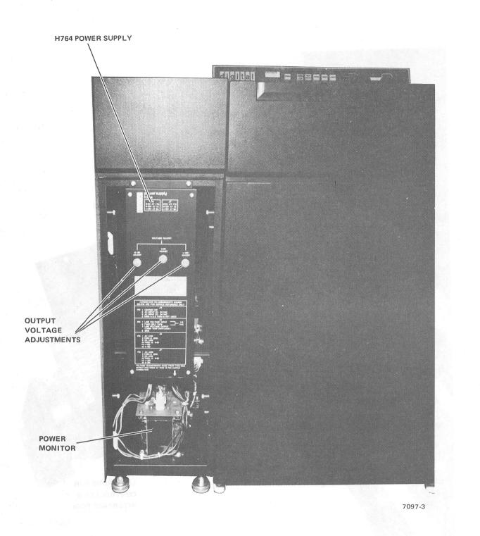
Figure 2-4 DCL Assembly Front View, Front Panel Removed
