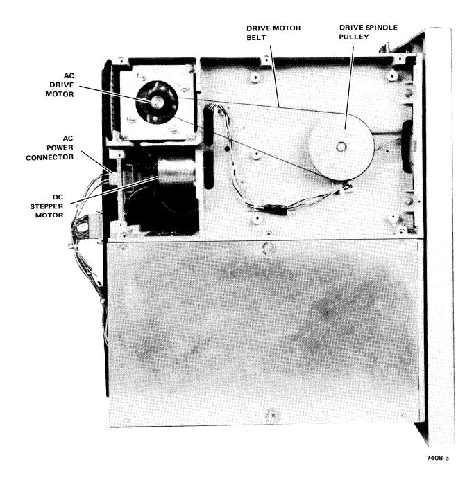
Figure 1-6 Underside View of Drive
