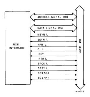
Figure 5-3 Unibus to RX11 Interface Signals
