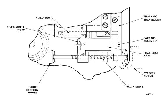
Figure 5-26 Positioning Mechanism
