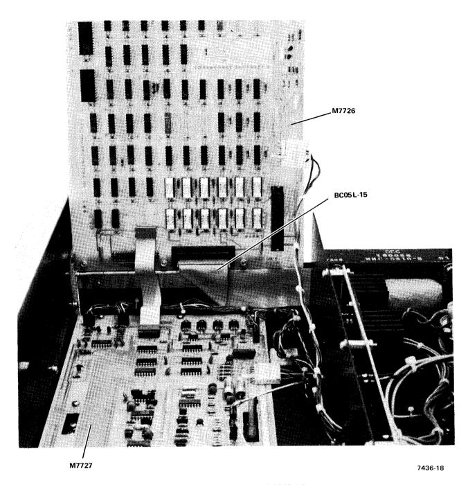
Figure 2-6 Cable Routing, BC05L-15
