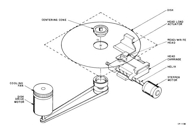
Figure 5-23 Disk Drive Mechanical System
