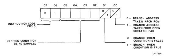
Many conditions are sampled by the Conditional Branch instruction; examples are 12-bit mode, drive ready, read/write head located at track zero, and two index pulses have occurred. A complete breakdown of all Conditional Branch subfunctions is given in the RX8/RX11 Print Sets.
