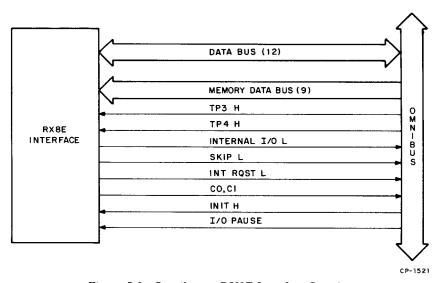
Figure 5-2 Omnibus to RX8E Interface Signals
