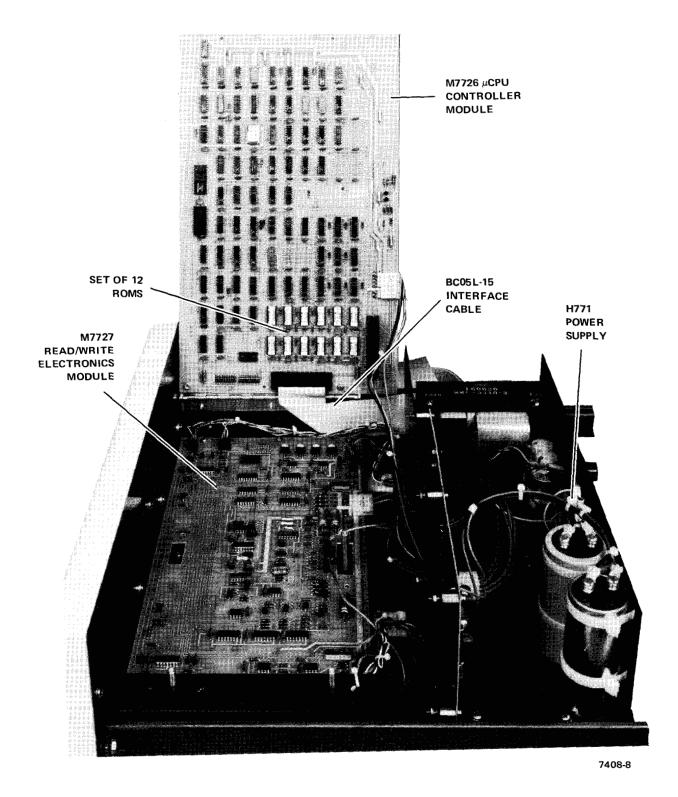
Figure 1-5 Top View of the RX01
