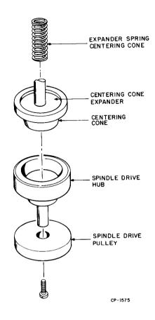
Figure 5-25 Centering Cone and Drive Hub
