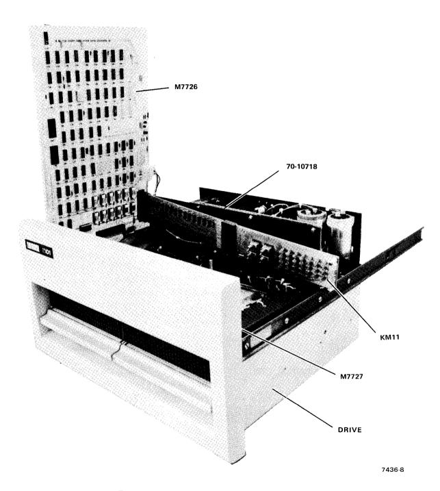
Figure 6-6 KM11 Maintenance Module Inserted
