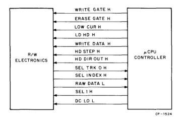
Figure 5-5 µCPU Controller to Read/Write Electronics Signals
