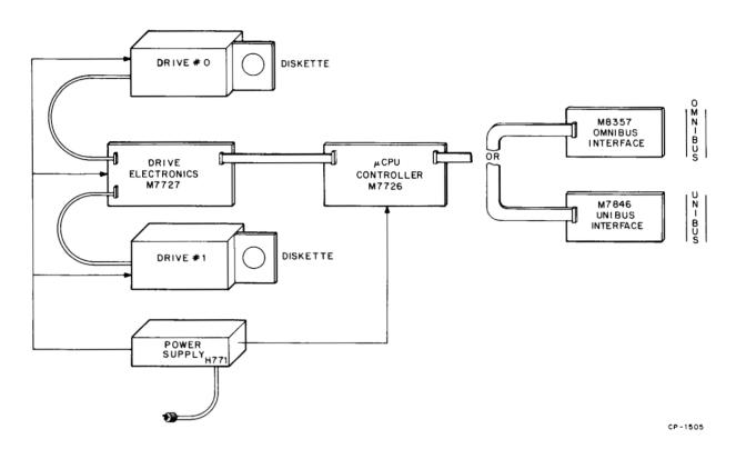
Figure 1-1 Floppy Disk System Configuration
