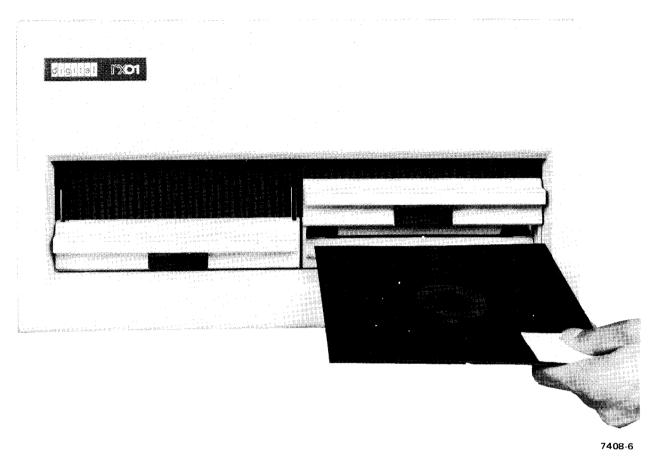
Figure 2-7 Flexible Diskette Insertion
