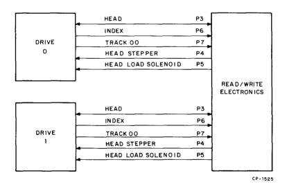
Figure 5-6 Read/Write Electronics to Drive Signals
