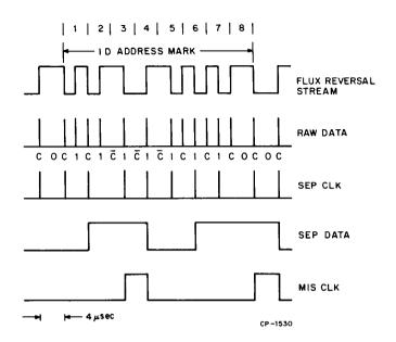
Figure 5-11 ID Address Mark Data Separation
