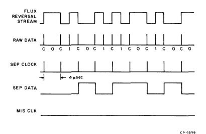
Figure 5-10 Data and Clock Separation
