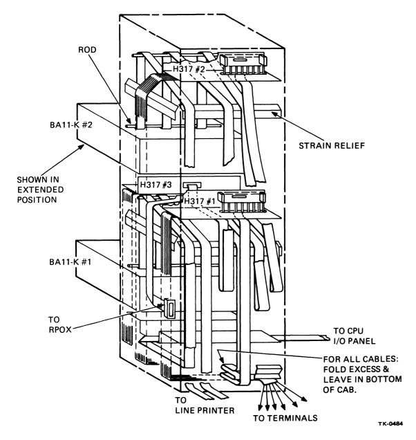
Figure 3-12 Unibus Expander Cabinet, Cable Arrangement, Rear View
