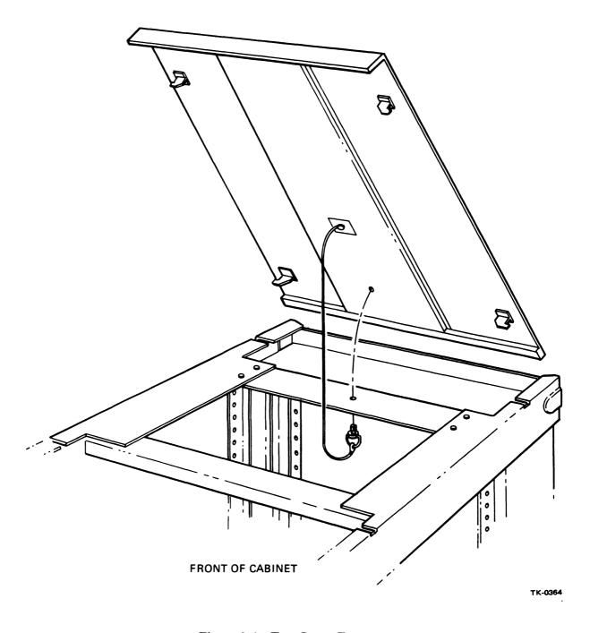
Figure 3-4 Top Cover Fastener
