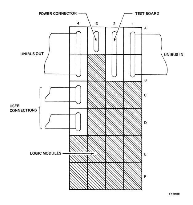
Figure 3-16 DR11-B System Unit Slot Allocation
