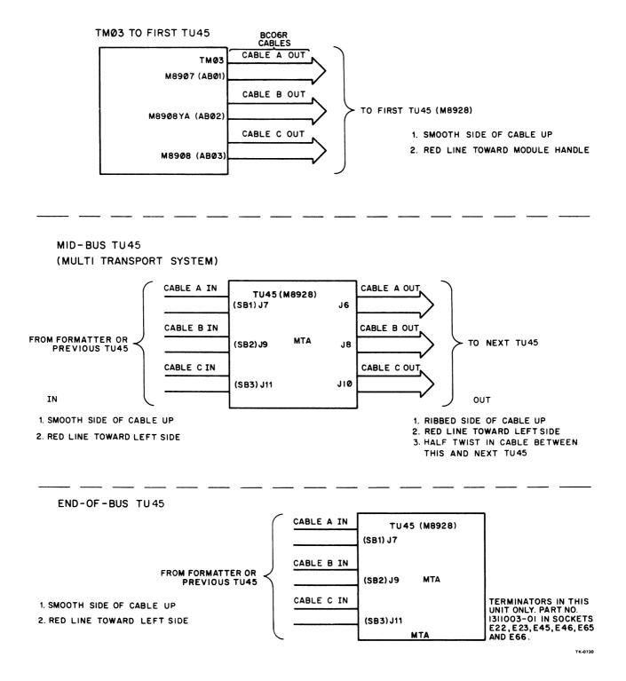
Figure A-2 TM03/TU45 Slave Bus Cabling
