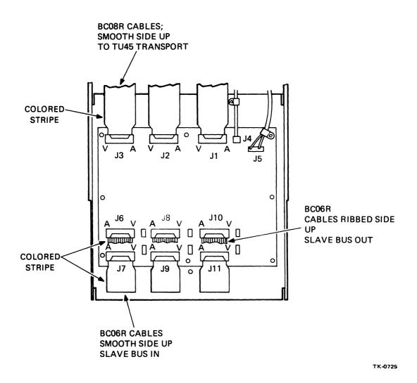
Figure A-3 Cable Orientation on M8928 MTA Module
