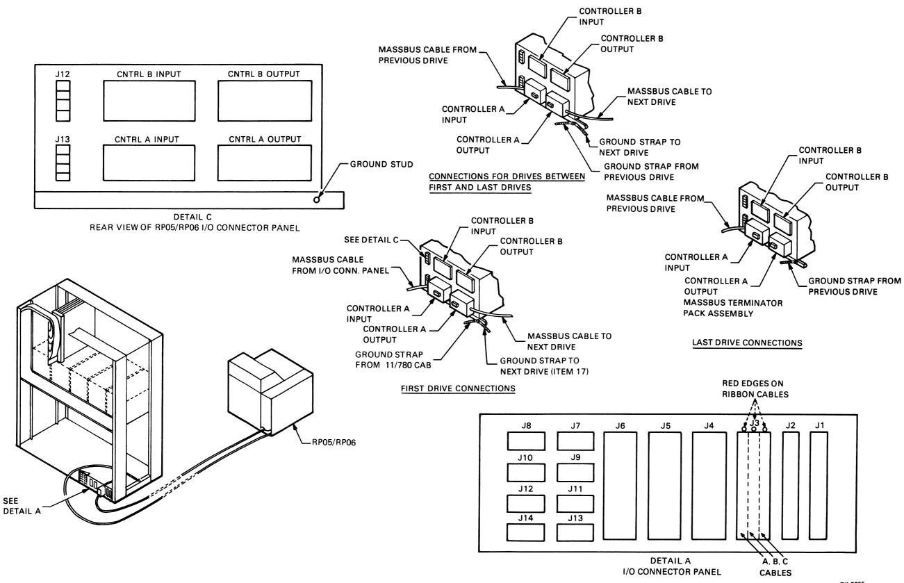
Figure 3-14 RP05/RP06 Cable Connections
