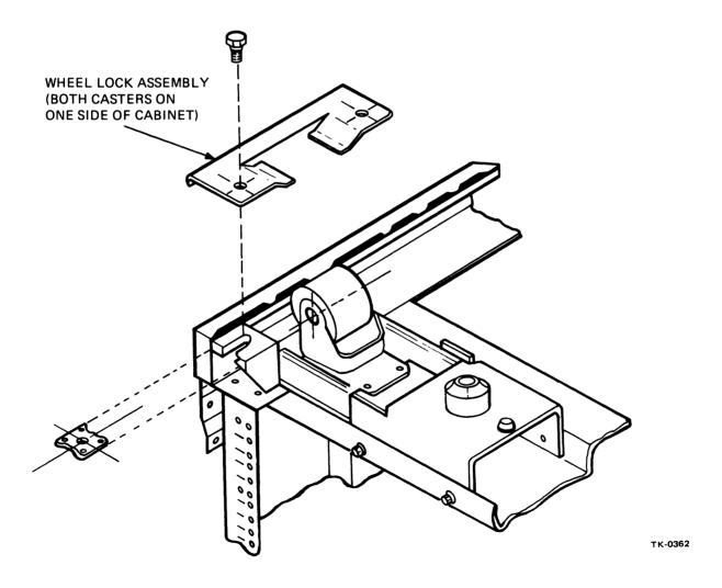
Figure 3-3 Wheel Lock Assembly
