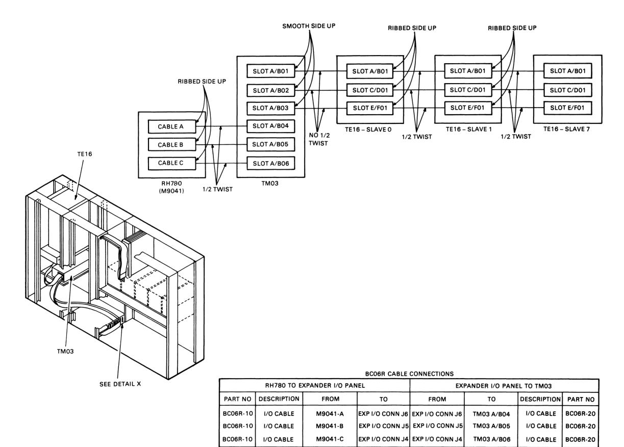
Figure 3-13 TE16 Cable Connections
