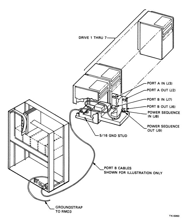
Figure 3-15 RM03 Cable Connections
