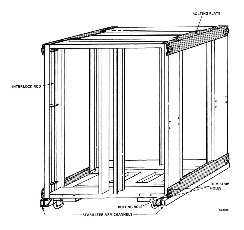
Figure 3-8 Cabinet Frame with Bolting Plates, Stabilizer Channels, and Interlock Rod
