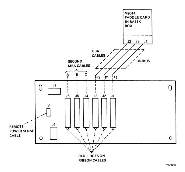
Figure 3-11 Unibus Ribbon Cable Connections
