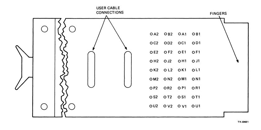
Figure 3-17 M957 Split Lug Cable Board
