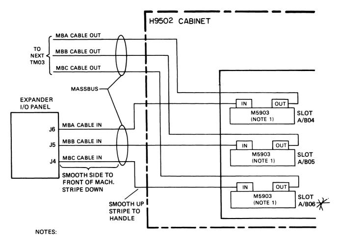
IF ONLY ONE TM03 IS USED IN SYSTEM, AN H870 TERMINATOR IS INSERTED INTO EACH OUT JACK, OR M5903-YA MODULES ARE USED WHICH PROVIDE MASSBUS TERMINATION.
