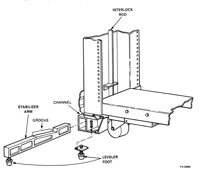
Figure 3-5 Stabilizer Arm and Leveling Pad
