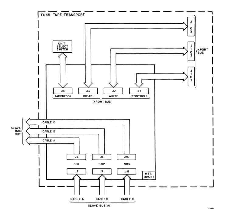
Figure A-4 MTA/TU45 Slave Bus Cabling
